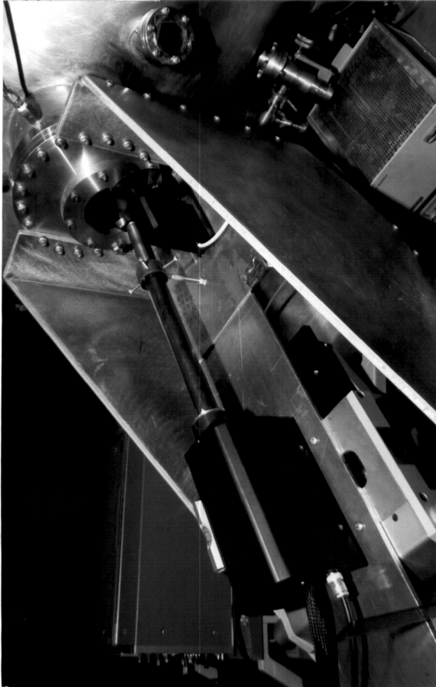
Figure 5.39: The radiometer, optics tube, and optical chopper mounted on the movable platform.
