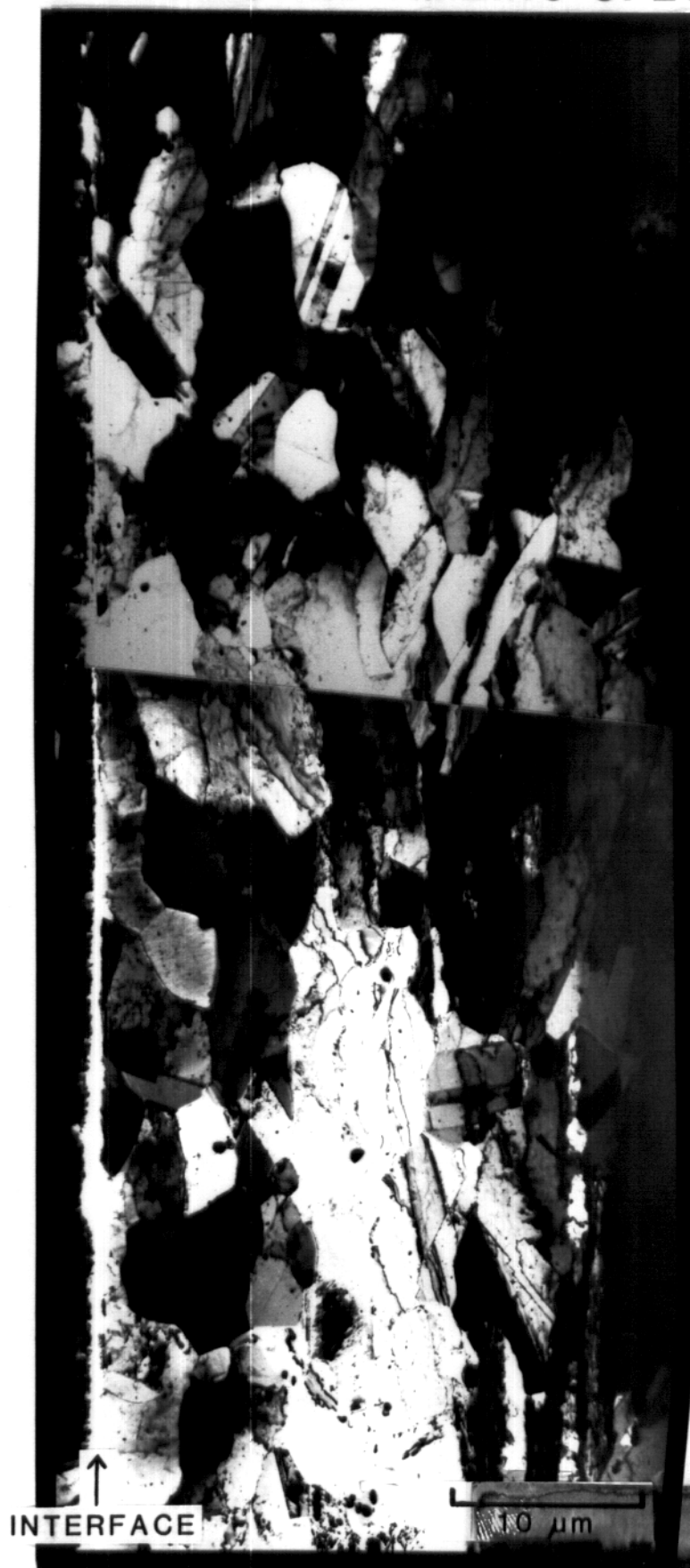
Figure 7. TEM micrograph showing the extent of the electron-transparent region along the irradiated boundary of a cross-sectioned Cu-Zr specimen.
