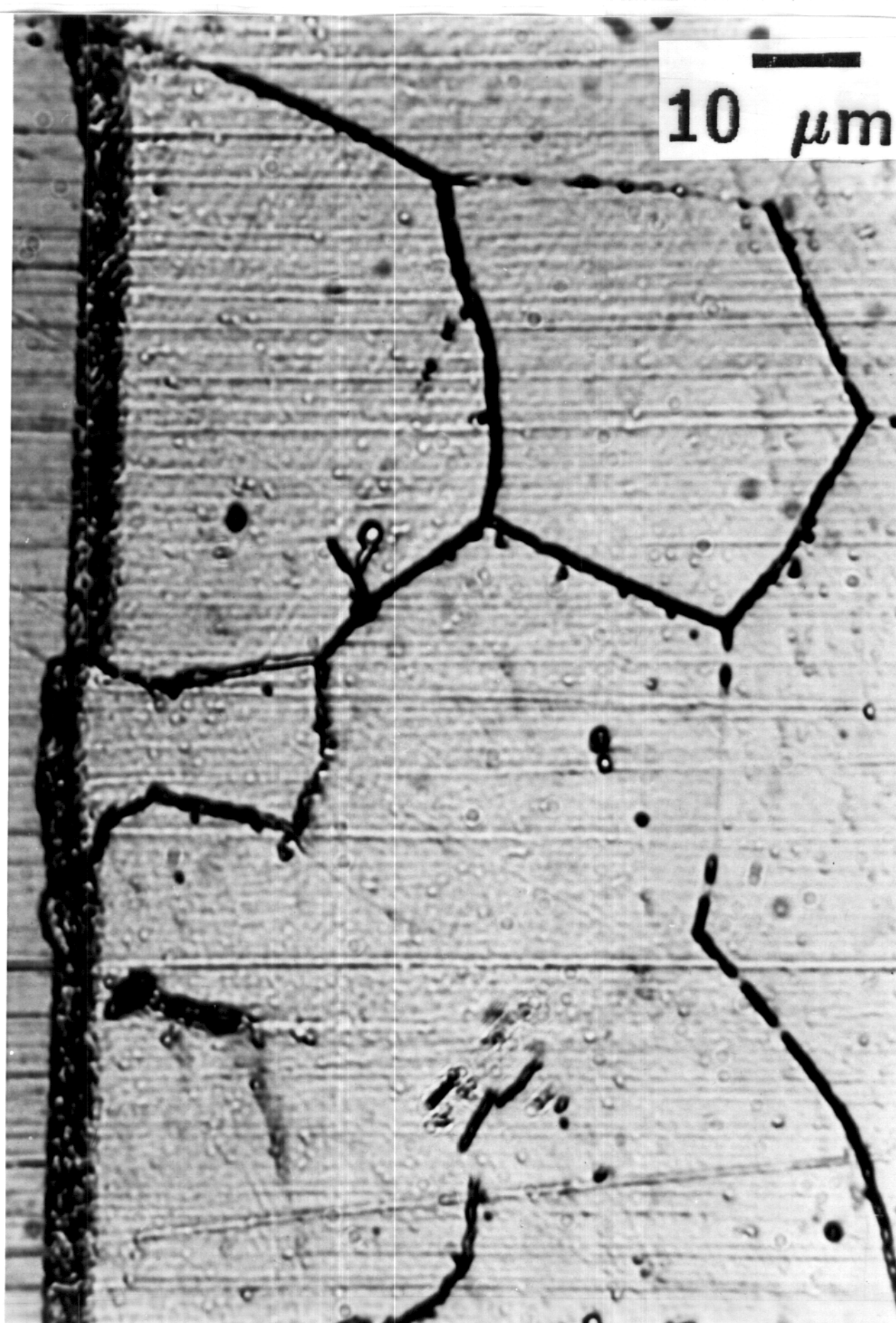
Figure 8. Optical micrograph of a 14-MeV Ni ion irradiated 316 stainless steel cross-section specimen (40 dpa peak damage). The 3 \mu\text{m} -wide band along the irradiated interface corresponds to the radiation damage region.
