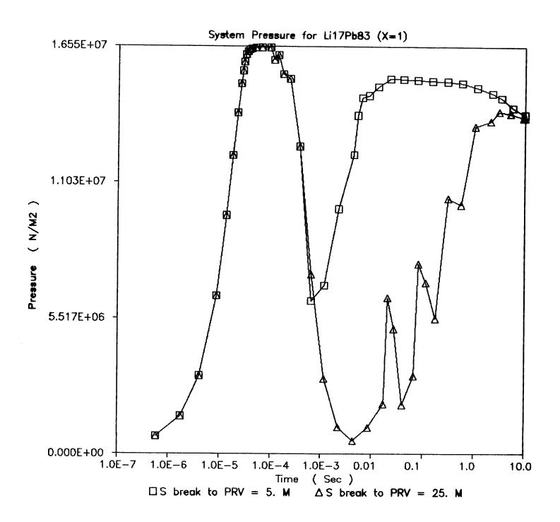
break to the pressure relief valve and for the subsequent pressure relief to be felt back at the break. Therefore the balance between water inflow and liquid metal outflow will take place on a timescale greater than 27 ms. This is the the reason for the oscillating behavior displayed by the pressure trace from 20 ms to 1 s.
