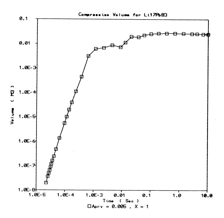
unreacted liquid metal out of the system through the pressure relief valve, is then quickly established. Once the balance is established, the compressible effects are suppressed and the break pressure for the new model mimics the break pressure for the old model.
