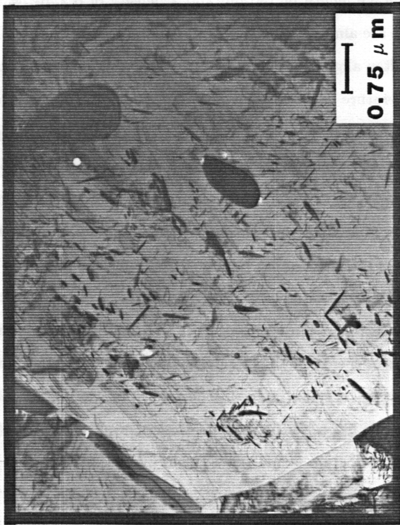
Figure 5.30 TEM micrograph showing all 6 \beta i precipitate orientations. Also shown are faulted loops pinned on \beta i precipitates.
