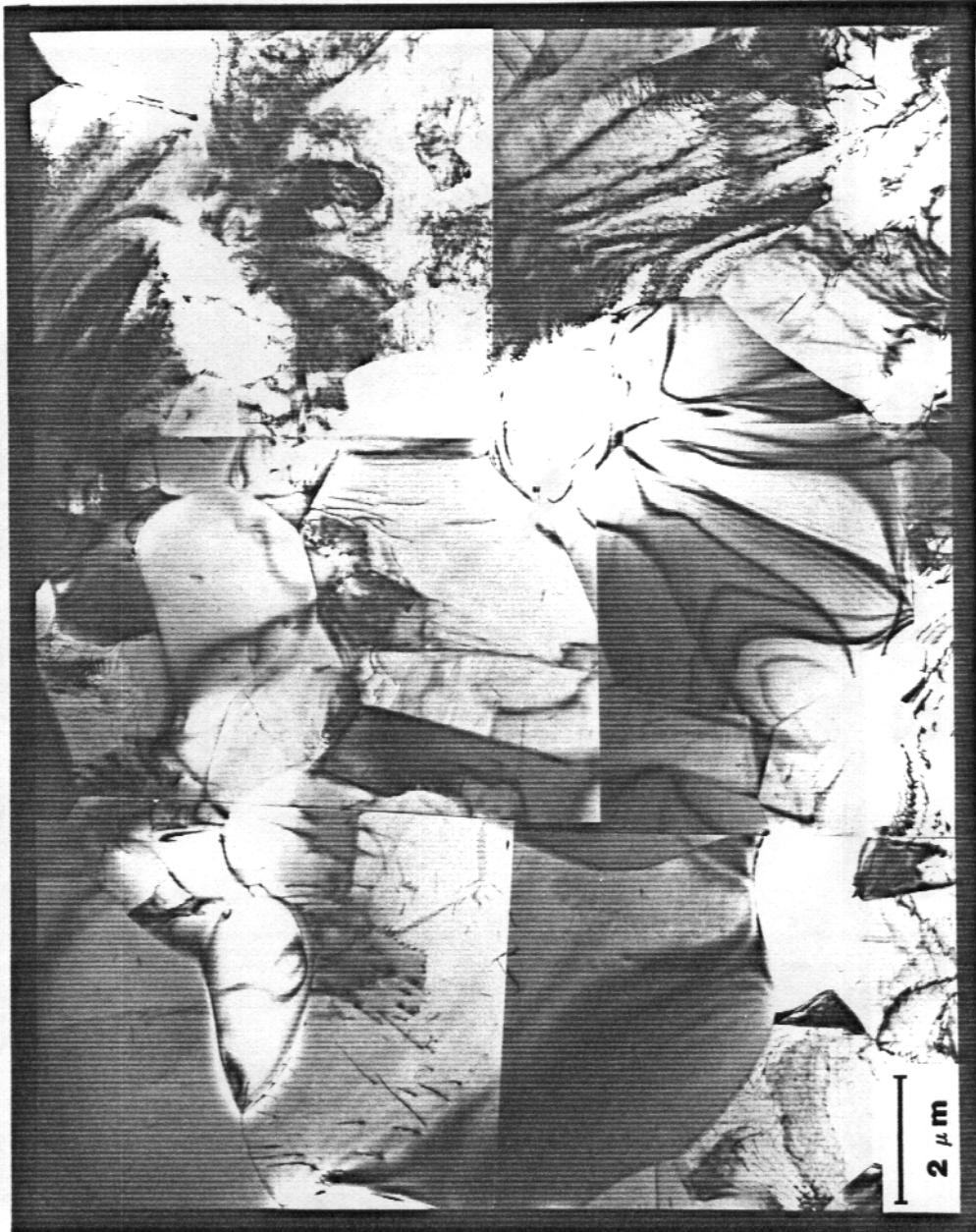
TEM micrograph showing some grain growth and recovery for Ti-64 annealed at 650°C for 8 hr.
