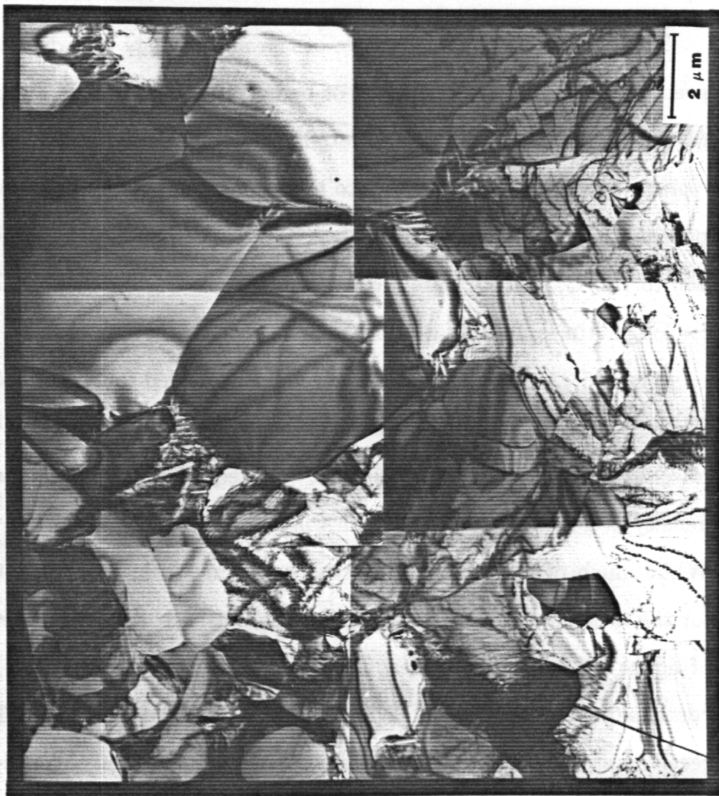
Figure 5.22 TEM micrograph illustrating grain structure and dislocation distribution in Ti-6242S annealed at 500°C for 8 hours.
