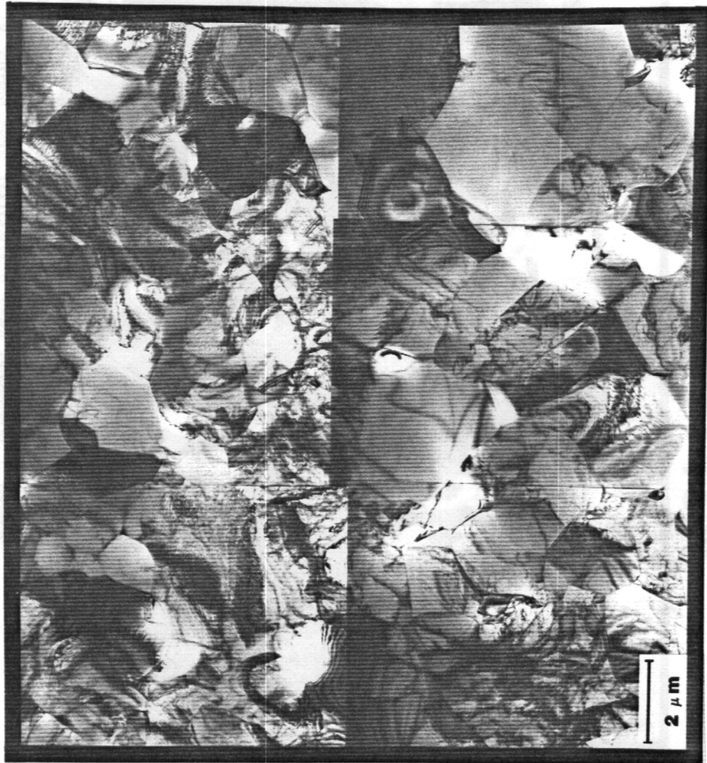
Figure 5.12 TEM micrograph showing the grain structure and dislocation distribution in Ti-64 annealed at 500°C for 8 hr.
