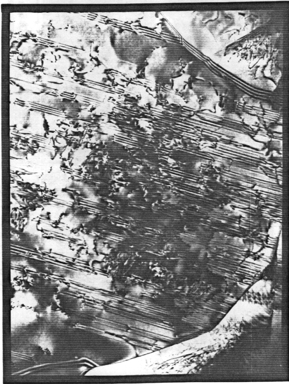
Figure 5.32 TEM micrograph showing stacking faults, an indication of the extensive recovery that has occurred.
