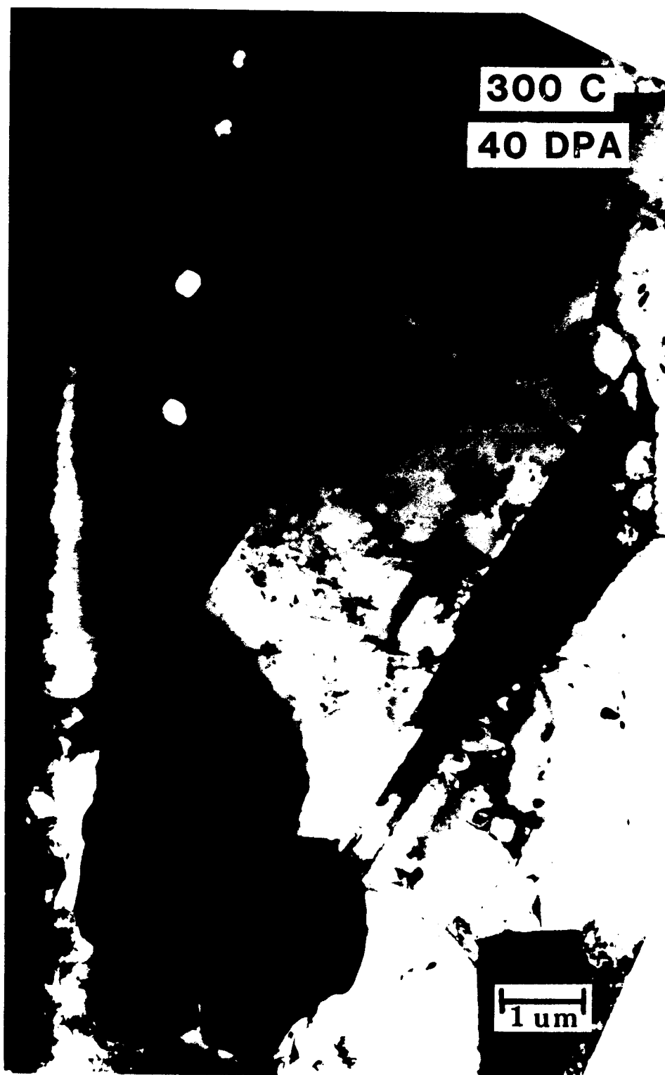
Fig. 7.25. Isolated voids observed in annealed AMZIRC following ion irradiation at 300°C to a peak damage level of 40 dpa.
