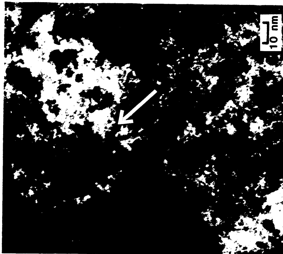
Fig. 7.31. Moiré fringe precipitate in AMAX-MZC following ion irradiation to 10 dpa at 100°C and associated matrix plus precipitate diffraction pattern.
