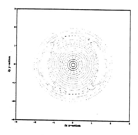
Figure 7  $x_o = 1.0$  and s = 0.01. The section shows again the increase in amplitude as compared to one-half the Bennett radius.
