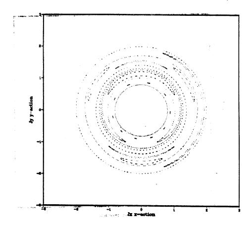
Figure 15  $x_o = 1.0$  and s = 0.001. Interaction between the one-one and onethree islands has generated satellites but there is no apparent instability yet.
