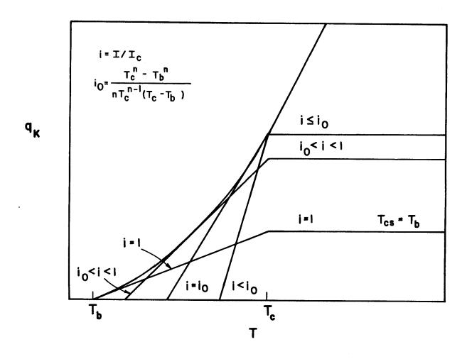
Fig. 3. Relationship of the Kapitza heat conducting curve to Joule heat generation curves for various values of i, the ratio of operating to critical current.
