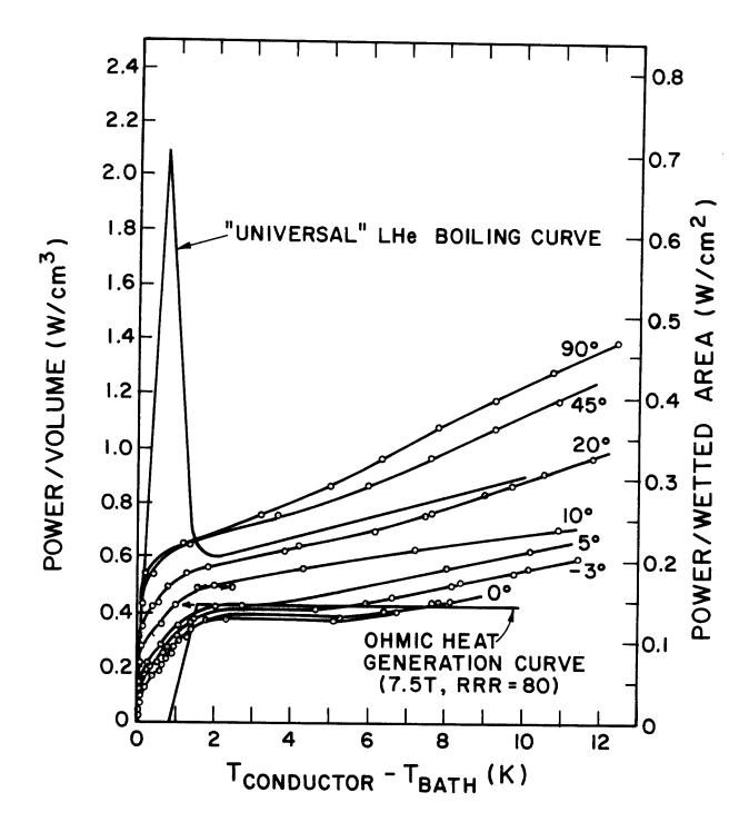
Fig. 2. Measured steady-state heat removal in saturated 4.2 K He-I from a mockup of the General Electric LCP coil winding pack at various inclinations of the conductor axis from the horizontal. Shown for comparison is a "typical" heat transfer curve.
