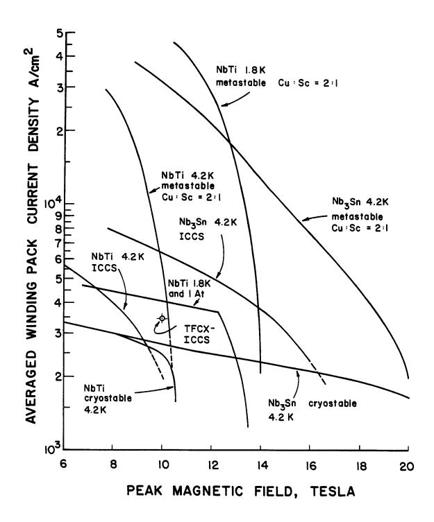
Fig. 1. Stability-limited winding pack current densities for various stabilization methods. See text for detailed explanations of assumptions to derive the individual curves.
