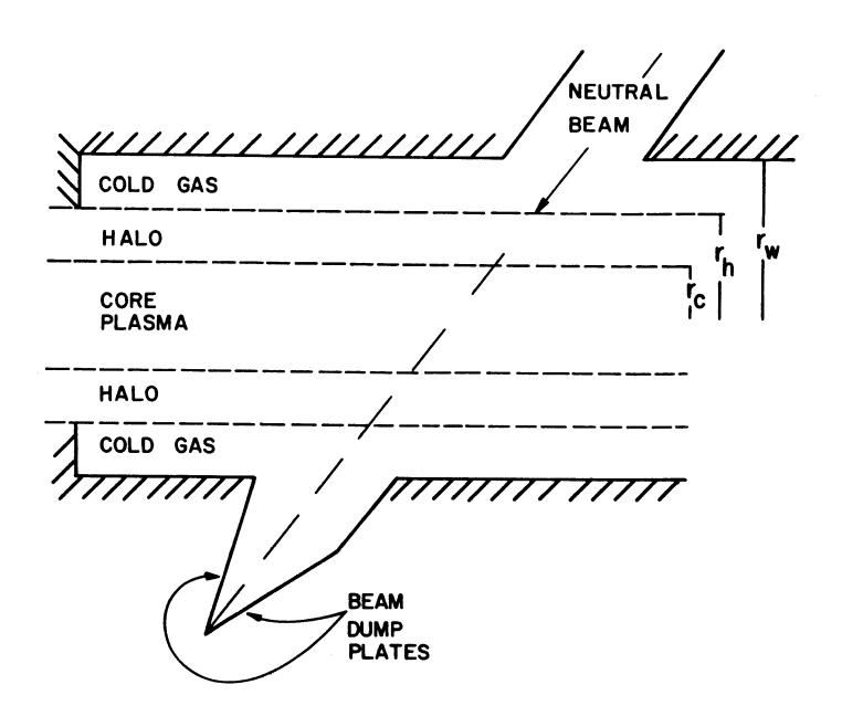
Fig. 1. Model geometry used for the halo calculations. The plasma is modeled as concentric cylinders.
