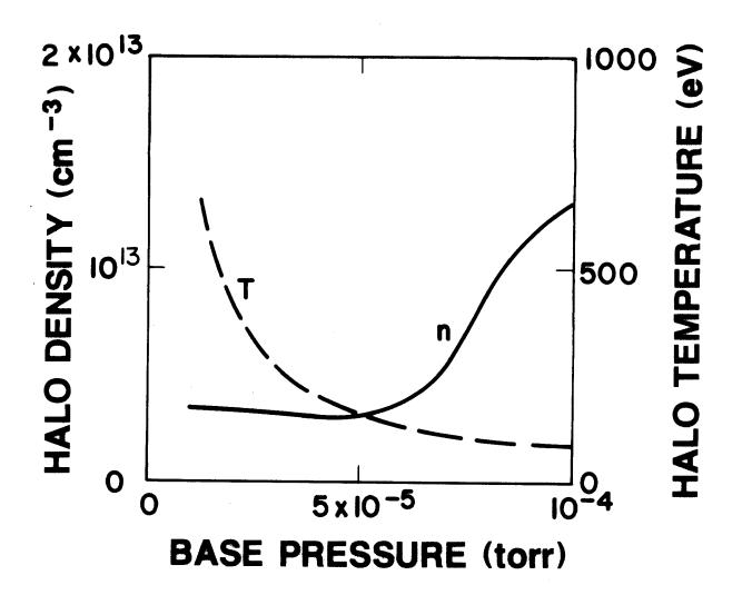
Fig. 6. TASKA-M halo density and temperature vs. base pressure.
