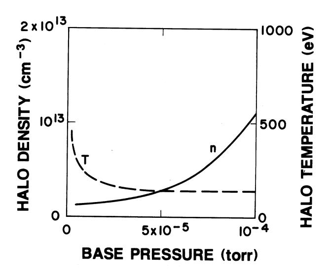
Fig. 5. TDF halo density and temperature vs. base pressure.
