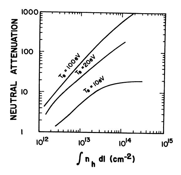
Fig. 2. Attenuation of neutral gas vs. line density ( $\int n_h d \mathbf{l}$ ).
