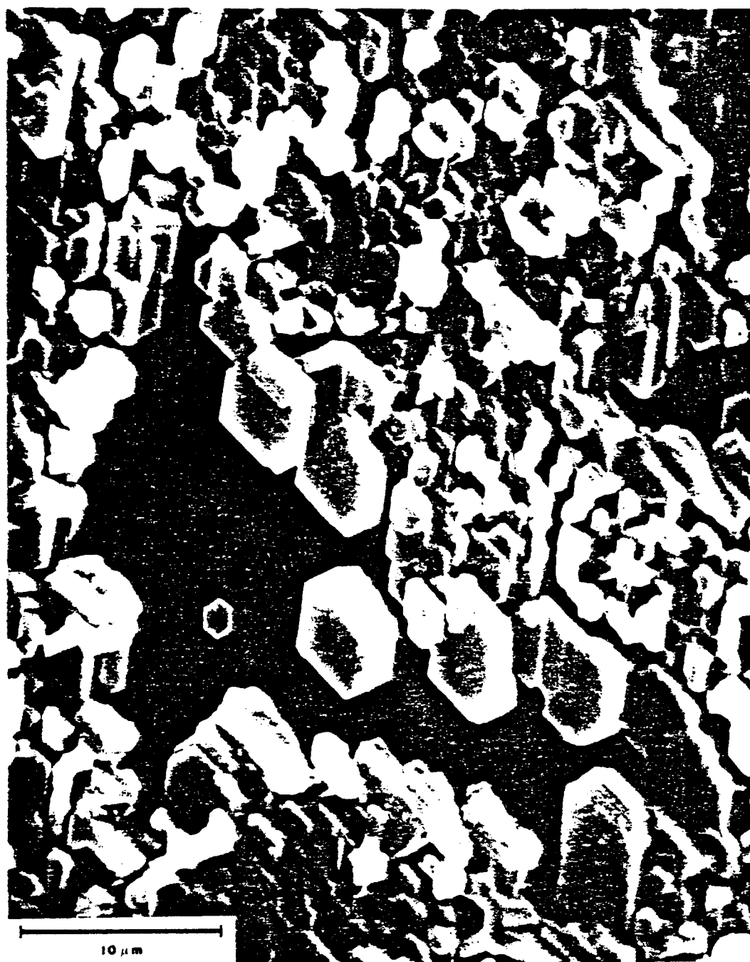
Figure 4.27 A scanning electron micrograph of the zincating material reveals the hexagonal nature of the zinc electroless deposit. The chemical activity of the aluminum drives the reaction to replace the aluminum with zinc metal. The close packed atom planes of the FCC aluminum and HCP zinc are closely matched.
