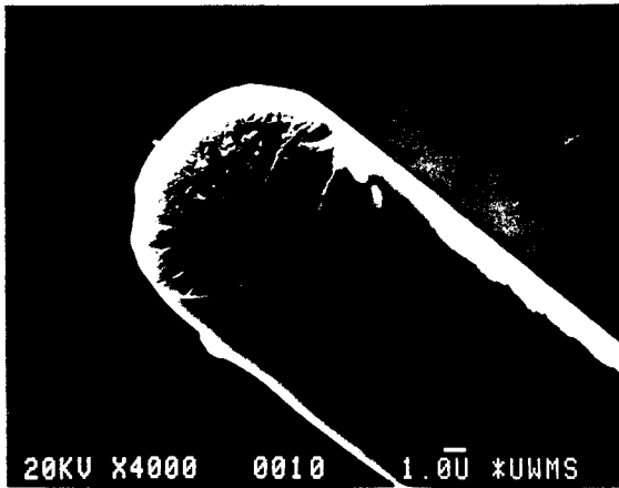
FIGURE 7 SEM micrograph of filament tensile failure.
