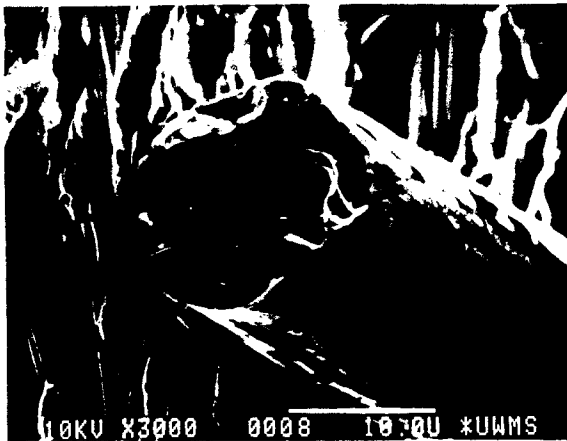
FIGURE 12 Fatigue fiber fracture at 18,600 cycles for \sigma_m/\sigma_f = 40\% ; \sigma_a/\sigma_f = 20\% .
