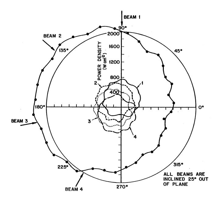
Fig. 3. Composite polar distribution of charge exchange power density at the first wall for four beams. The axial coordinate is  $z'=-0.025\ m.$
