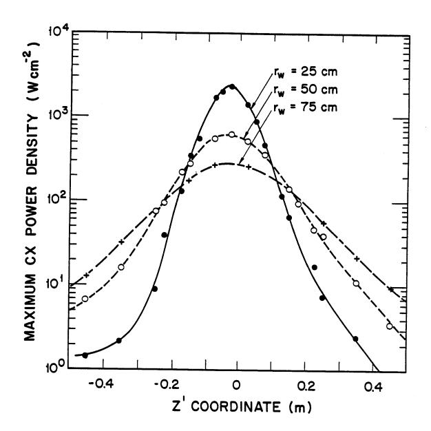
Fig. 5. Effect of first wall radius on the axial variation of maximum charge exchange heat loads.
