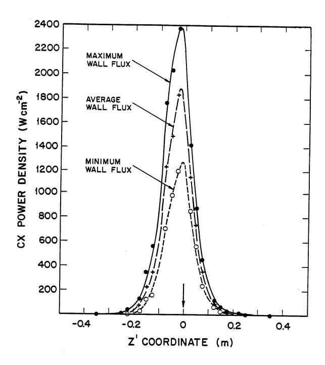
Fig. 4. Axial variation of charge exchange heat loads for a first wall radius of 25 cm. The beam intersection point is at z'=0.
