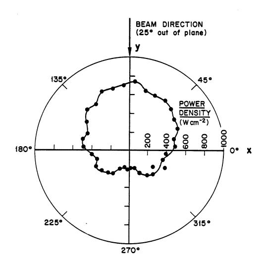
Fig. 2. Polar distribution of charge exchange power density at the first wall for one beam. The axial coordinate is  $z'=-0.025\ m$ .
