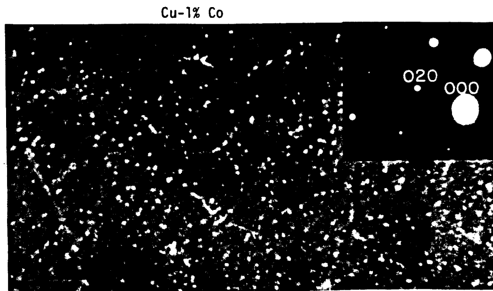
Figure VIII.4. Cu-1%Co solution annealed and quenched, then irradiated at 475°C to 5 dpa. Dark field image using (002) matrix reflection.
