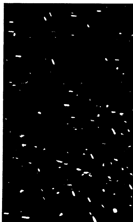
Figure VII.27(a) [001] diffraction pattern from Cu-3.4 at% Be irradiated at 350°C to about 10 dpa. The matrix reflections (intense spots) and precipitate reflections are indexed in the schematic. Precipitate reflections labeled B-E correspond to the (100), (200), (110) and (220) planes of CuBe, respectively. Reflections A and F are from (100) and (111)-type CuBe planes. DF image(i) is from (020) / (110) ppt. reflections, while (ii) and (iii) DF images are from ppt. reflections A and B respectively.
