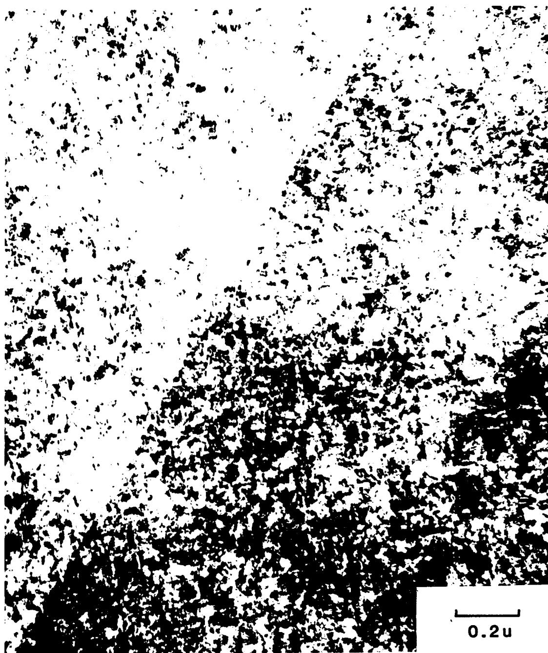
Figure VI-8. Bright field image of the damage structure at a grain boundary irradiated at 23°C to 0.64dpa at a damage rate of 1.8 \times 10^{-4} dpa/sec.
