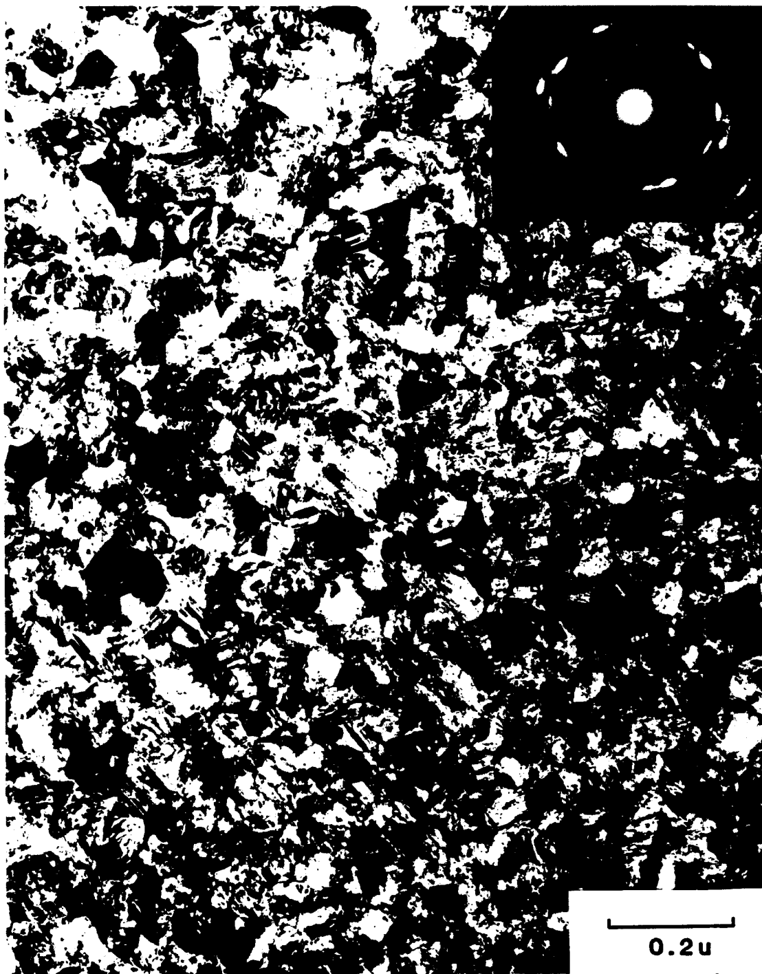
Figure VI-4. Bright field micrograph showing damage structure of an initially ordered specimen irradiated at 23°C to 0.26 dpa at 1.3 \times 10^{-3} dpa/sec including the diffraction pattern.
