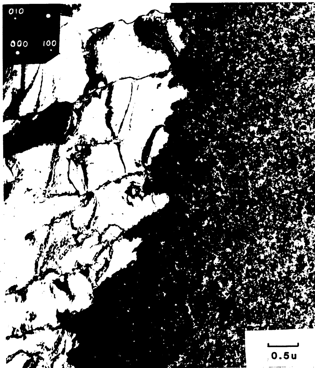
Figure VI-19. Boundary between the recrystallized ordered structure and the disordered matrix after post-irradiation annealing at 260^{\circ}\text{C} for 90 minutes. The sample was initially disordered by irradiation. The inserted diffraction pattern is from the recrystallized grain.
