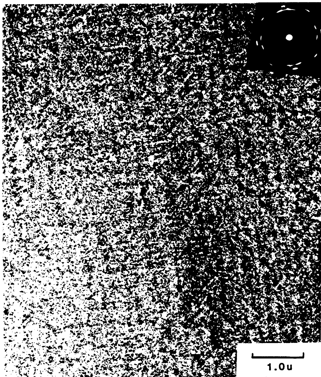
Figure VI-1. Damage structure shown in bright field of an initially ordered CuPd sample irradiated with 14MeV copper ions at 23°C to 0.64dpa at a rate of 1.0 \times 10^{-3} dpa/sec. Selected area diffraction is shown in insert.
