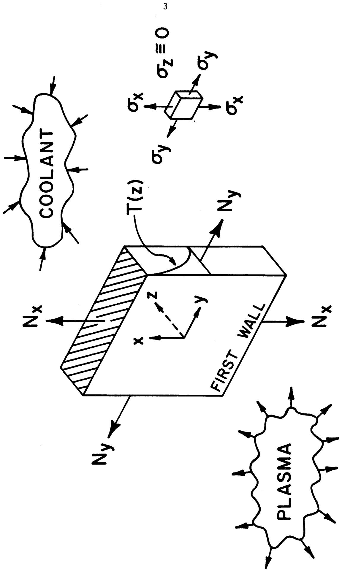
Figure 1 Thin Walled Shell Element Model of First Wall.
