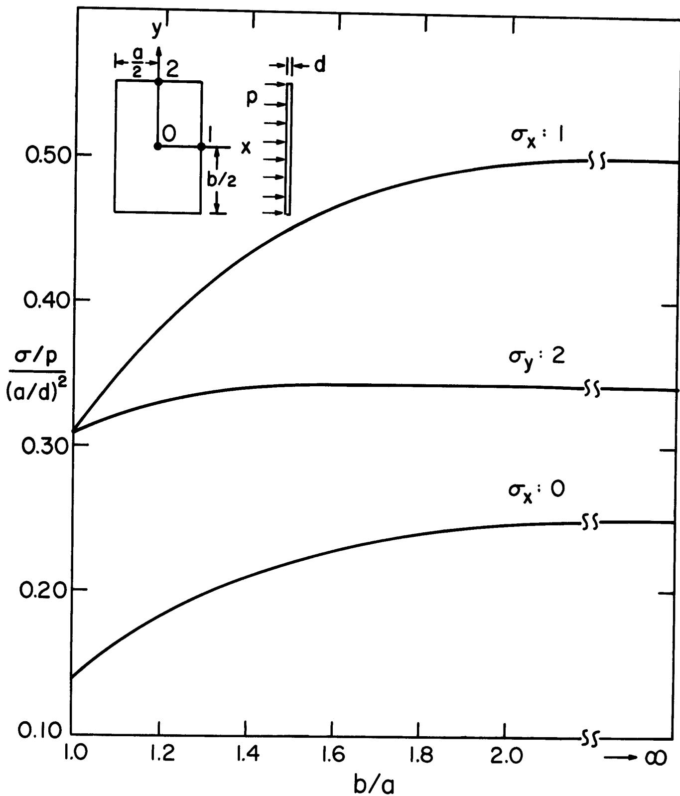
DIMENSIONLESS STATIC STRESS VS. ASPECT RATIO
