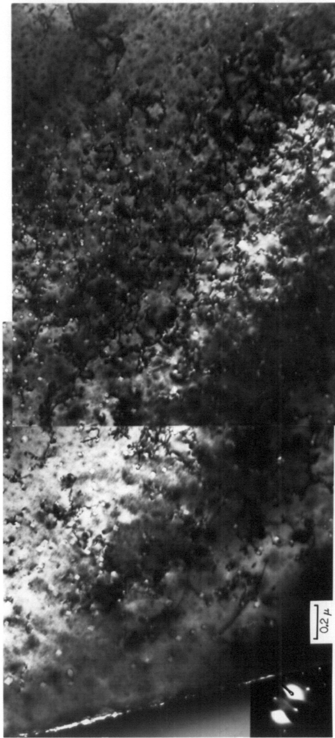
Figure 19. The dislocation structure in nickel after irradiation at 525 °C with 19 MeV copper ions to a fluence of 5 \times 10^{15} \text{ ions/cm}^2 .
