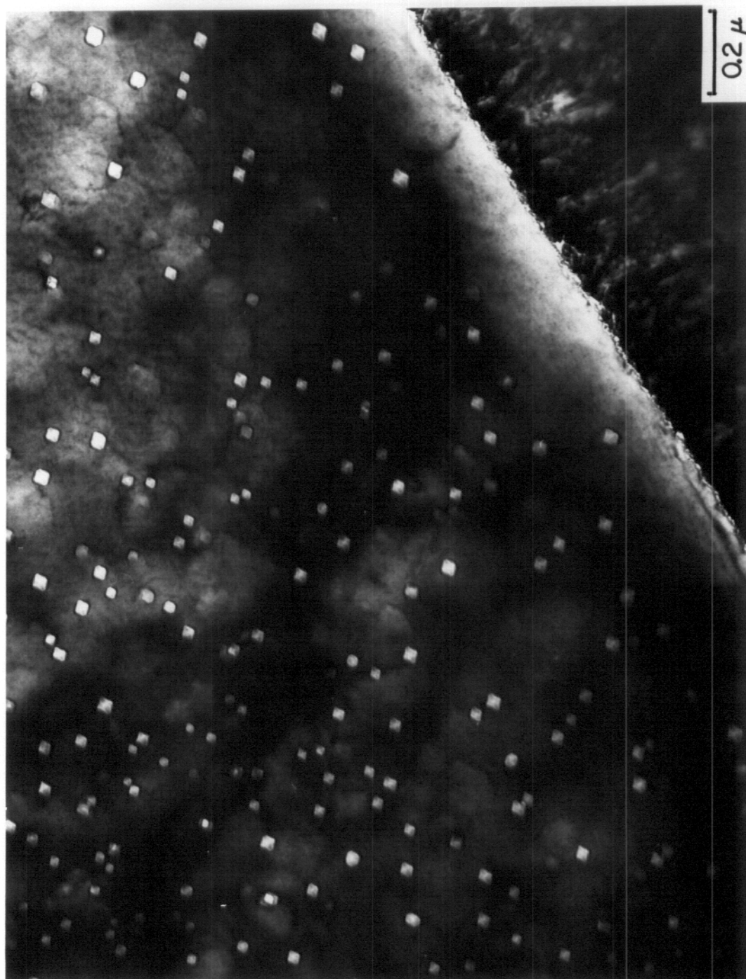
Figure 72. The surface region of a sample irradiated at 525°C with 19 MeV copper ions to a fluence of 5 \times 10^{15} ions/cm 2 .
