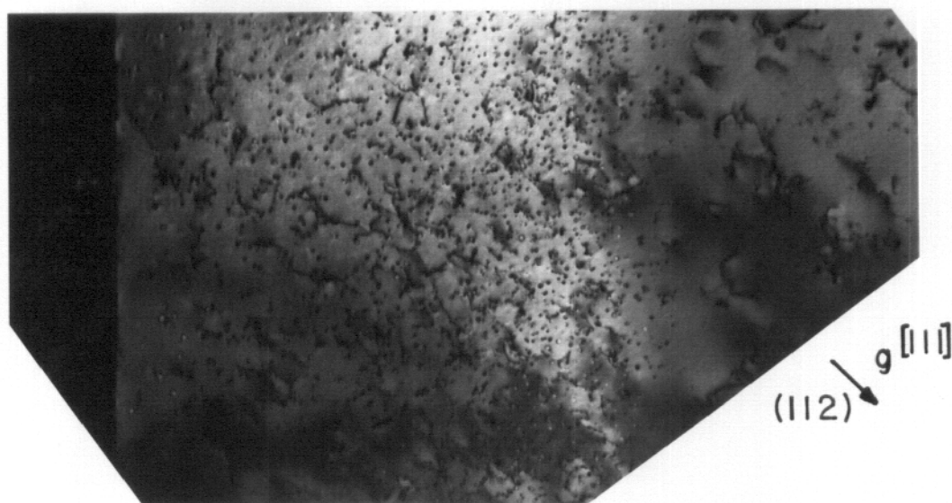
Figure 52. Dislocation structure in nickel irradiated at 525^\circ\text{C} with 14 MeV nickel ions to the fluence levels shown.
