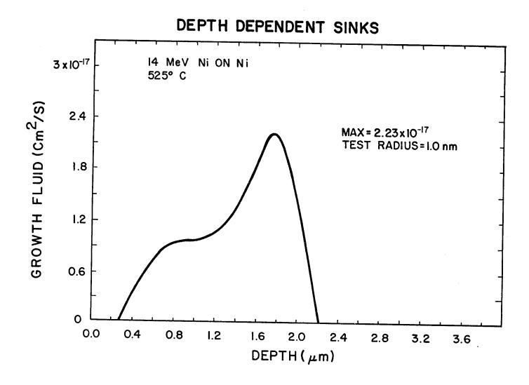
Fig. 5. The depth dependent growth fluid for a test radius of 1.0 nm using the defect concentration shown in Fig. 3.
