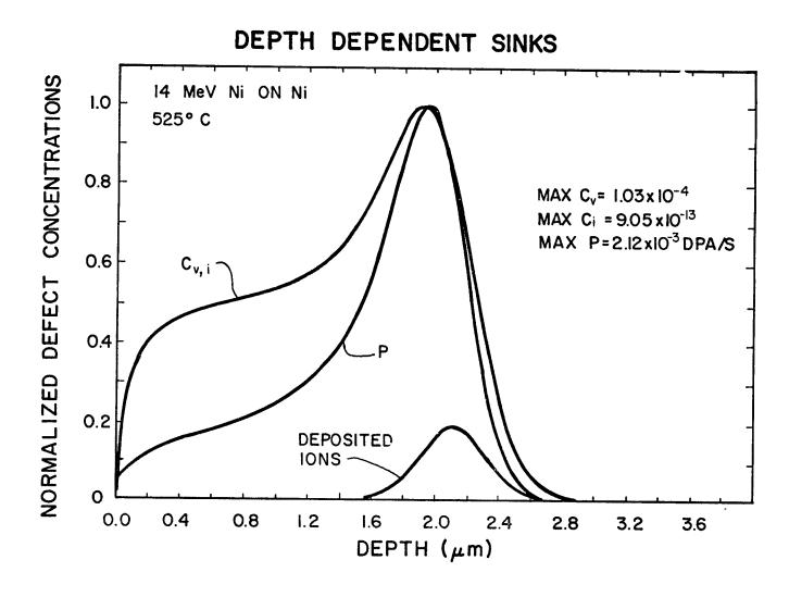
Fig. 3. Defect profiles for conditions identical to those of Fig. 1 except that an experimentally measured depth dependent dislocation density taken from Reference 3 was used.
