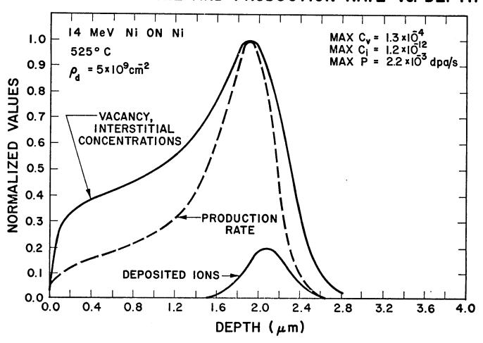
Fig. 1. Calculated vacancy and interstitial concentration profiles for 14 MeV nickel ions incident onto a nickel target. The curves are all normalized to the peak values shown in the figure.
