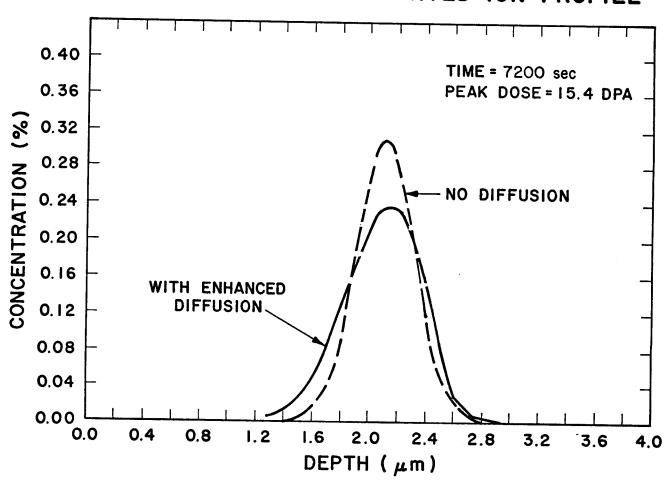
Fig. 11. The end-of-range distribution of copper ions incident on nickel after a total ion fluence of about  $1.5 \times 10^{16}$  ions/cm². The increased defect concentrations to the left of the ion end-of-range leads to a preferred migration of the copper toward the surface.
