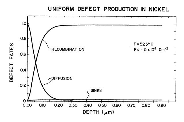
Fig. 9. The defect distributions from the calculations of Fig. 8. Note that diffusion of defects to the surface dominates over the first 0.1  $\mu m$  for these conditions.
