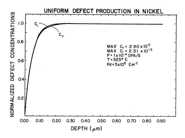
Fig. 8. The defect concentration profiles in a foil with uniform defect production and a uniform dislocation density of 5 x  $10^8$  cm<sup>-2</sup>.
