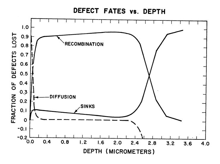
Fig. 2. The distribution of the defects produced by the calculation of Fig. 1 to their various sinks. A positive fraction for diffusion refers to a net loss of defects out of the depth interval while a negative fraction refers to a net gain of defects.
