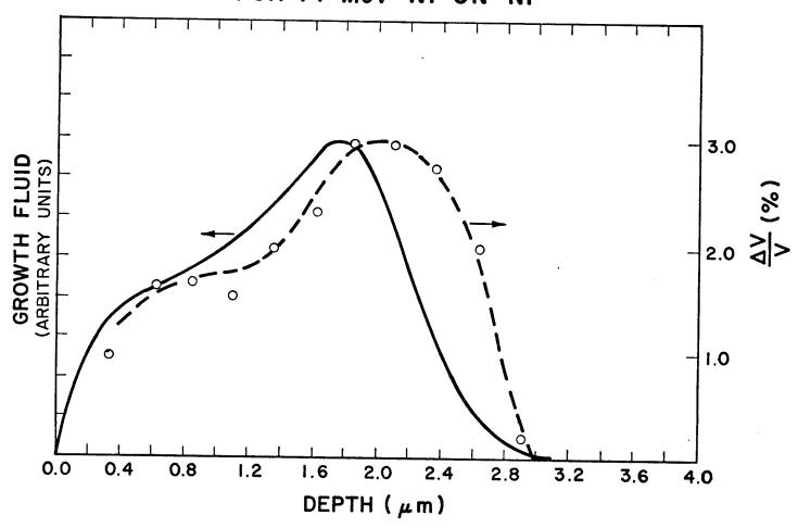
Fig. 7. A comparison of the growth fluid calculated using the defect concentrations shown in Fig. 1 to an experimentally measured swelling profile from Reference 3.
