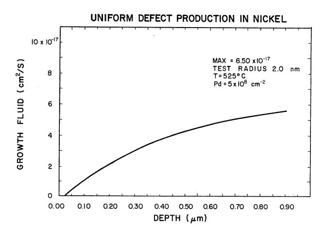
Fig. 10. The growth fluid calculated from the defect concentrations of Fig. 8.
