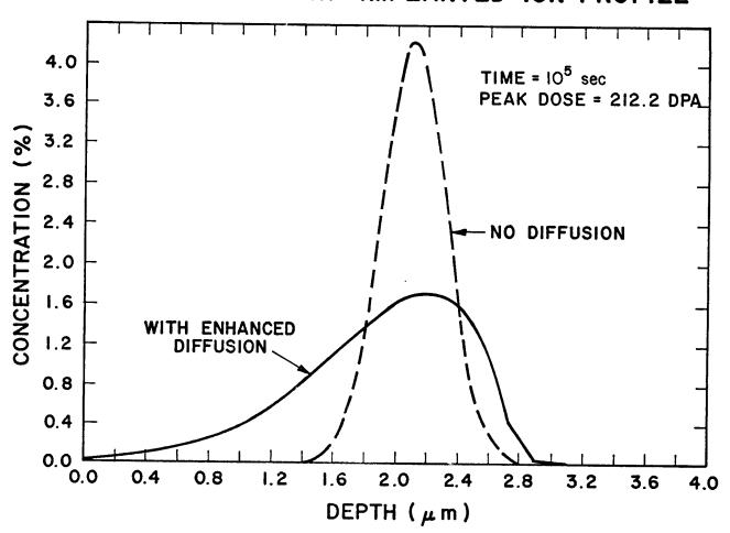
Fig. 12. The end-of-range distribution after a total ion fluence of about 2 x  $^{10^{17}}$  ion/cm $^2$ . The copper has now distributed itself throughout the ion range.
