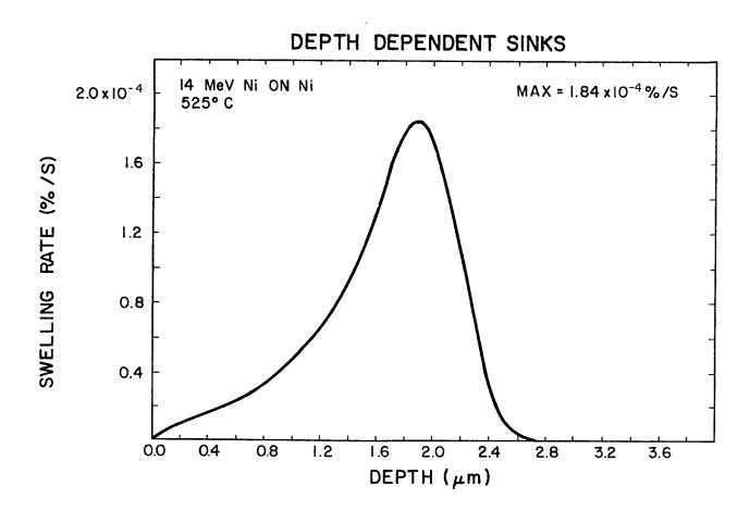
Fig. 6. The depth dependent swelling rate calculated using the defect concentrations of Fig. 3 and the experimentally measured void concentrations and sizes from Reference 3.
