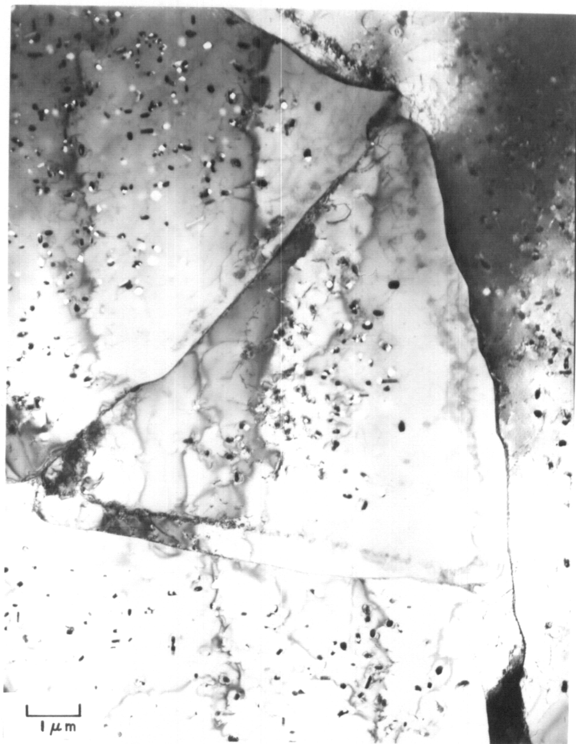
FIGURE 27. Void and precipitate denuding along grain boundaries in vanadium (Group I) irradiated at 650°C with 14 MeV Cu ions to 5 dpa.
