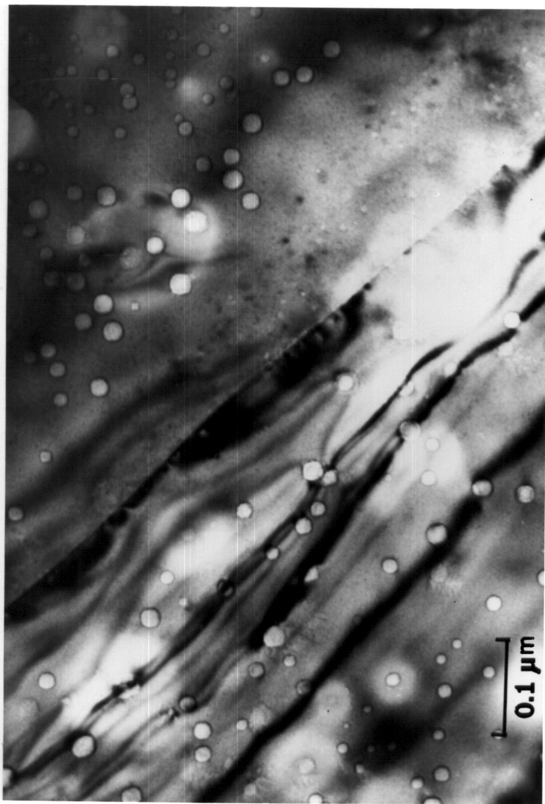
Figure IX. Void denuding near a grain boundary in Mo irradiated at 900°C to 1.9 dpa with 17 MeV copper ions.
