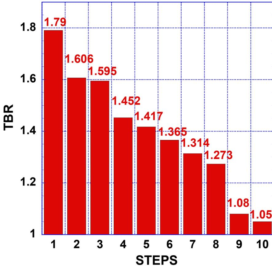
Fig. 3. Bar chart showing the reduction in TBR from 1.8 to 1.05 as a result of including internals and externals of ARIES-ACT-2 DCLL blanket.
