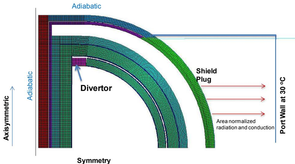
Fig. 6. Axisymmetric finite element model of the power core.
