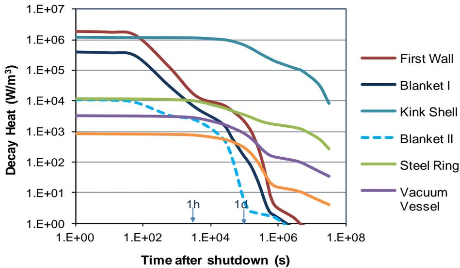
Fig. 7. Decay heats in outboard components.
