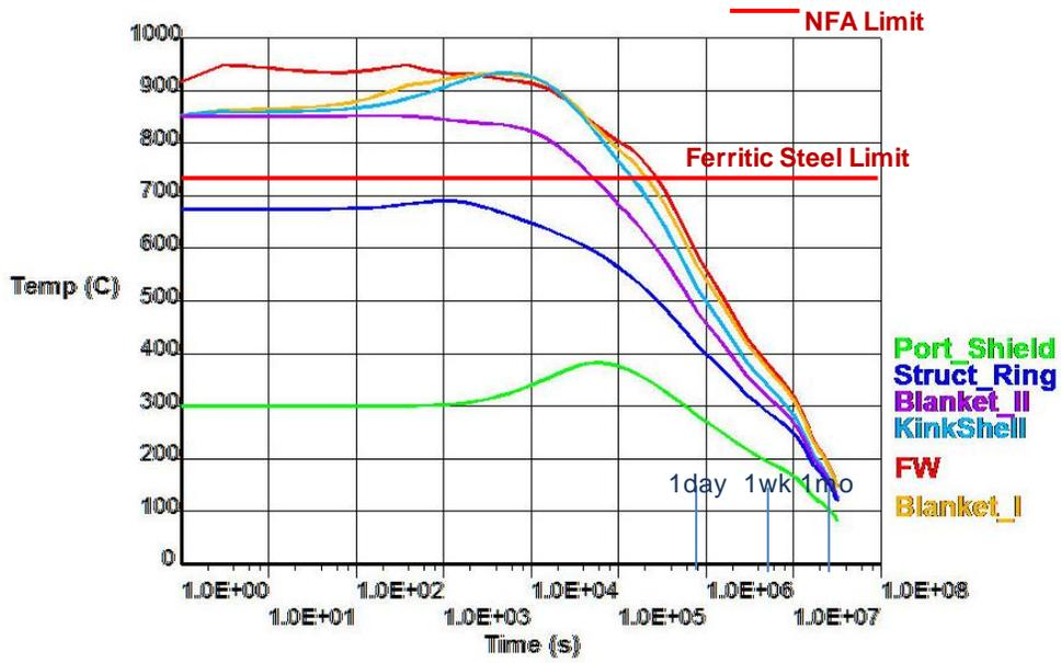
Fig. 15. Outboard temperatures with B-FS filler in inboard LT shield and assumed emissivities of 0.9 for all surfaces.
