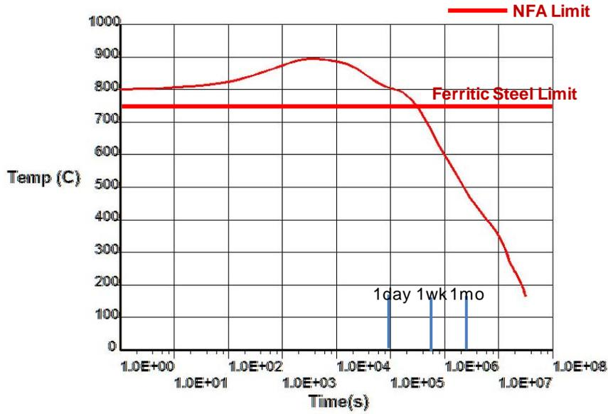
Fig. 17. Bulk divertor plate temperatures (emissivities of 0.9 for all surfaces).
