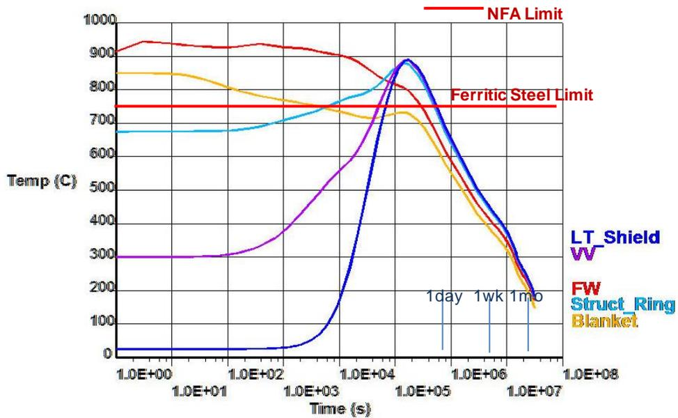
Fig. 16. Inboard temperatures with B-FS filler in inboard LT shield and assumed emissivities of 0.9 for all surfaces.
