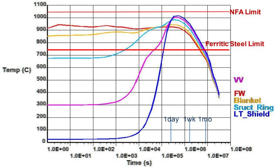
Fig. 12. Temperatures at midplane of inboard components after LOCA with cross channel radiation included.
