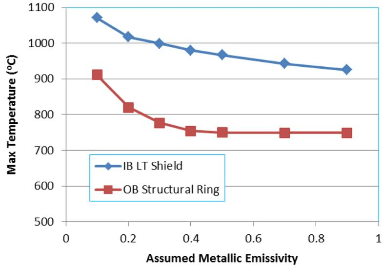
Fig. 13. Effect of assumed emissivity of the metallic surfaces on inboard and outboard temperatures of FS-based components.
