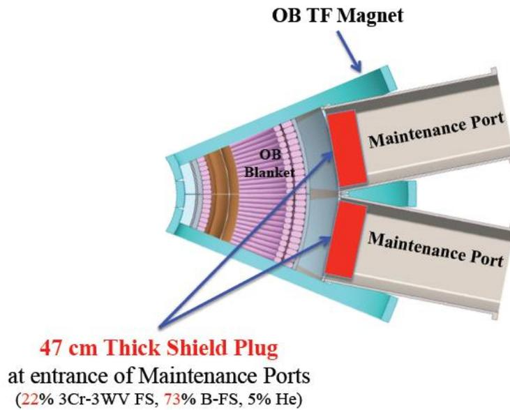
Fig. 2. Schematic of the maintenance port region and shield plugs.
