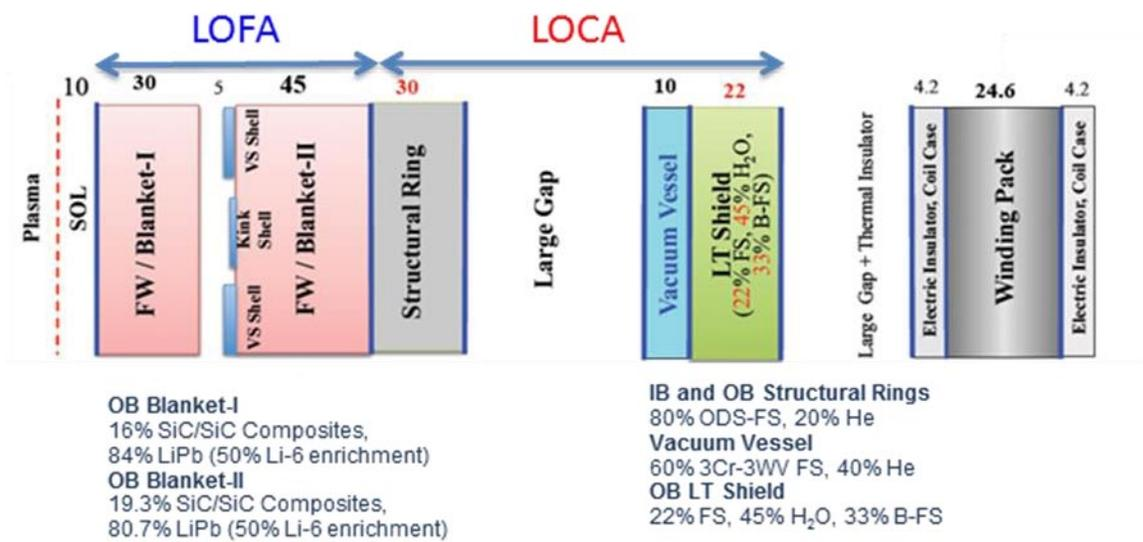
Fig. 3. Schematic of the outboard radial build with component material compositions.
