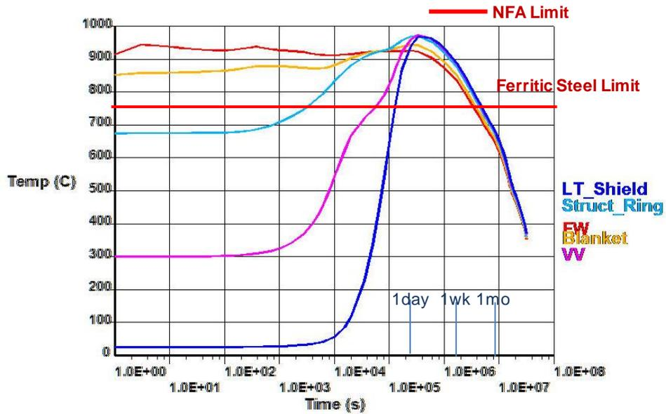
Fig. 14. Inboard temperatures with B-FS inboard LT shield and assumed 0.2 emissivity for the metallic surfaces.
