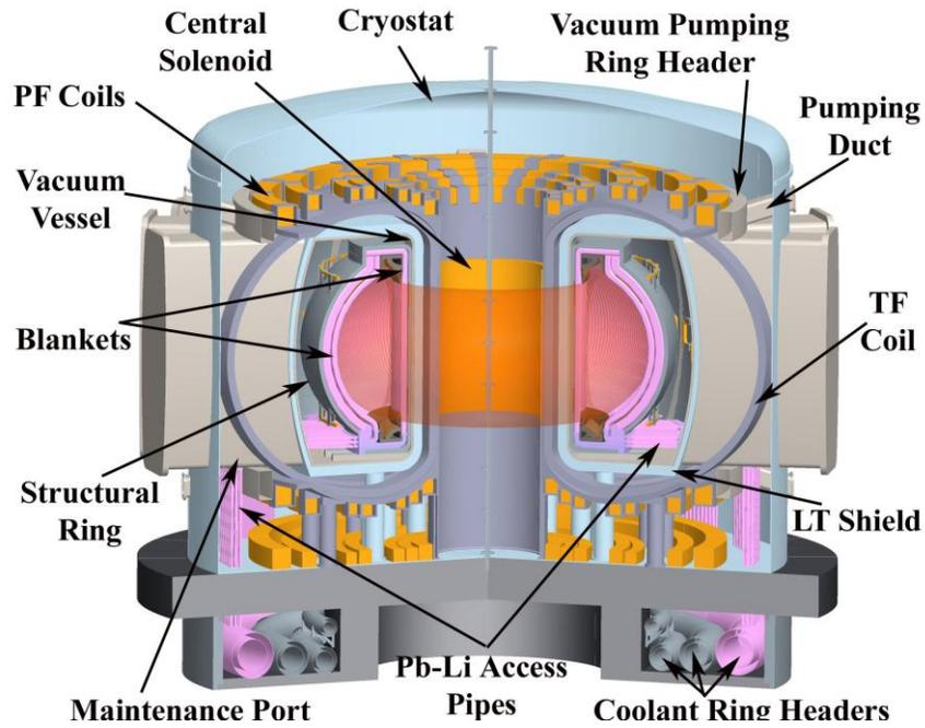
Fig. 1. Schematic of the ARIES-ACT-1 power core.
