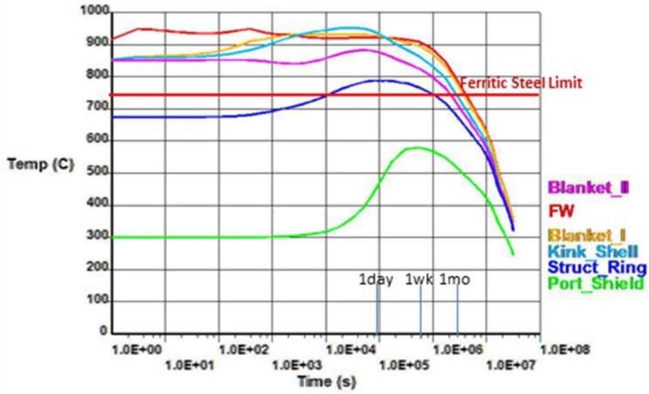
Fig. 11. Temperatures at midplane of outboard components after LOCA with cross channel radiation included.
