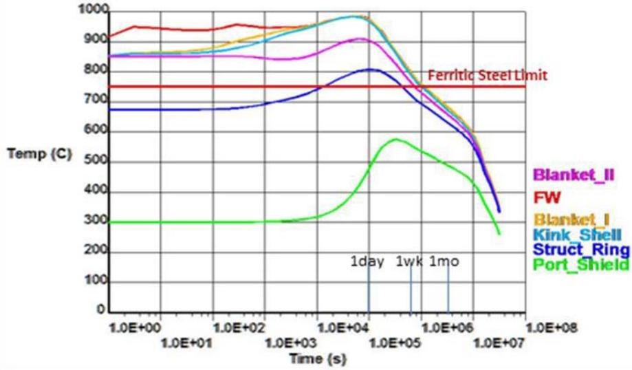
Fig. 9. Transient temperatures at midplane of outboard components after LOCA without cross-channel radiation modeled.
