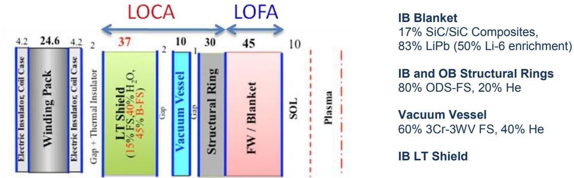
Fig. 5. Schematic of the inboard radial build with component material compositions with the borated ferritic steel filler in low temperature shield.
