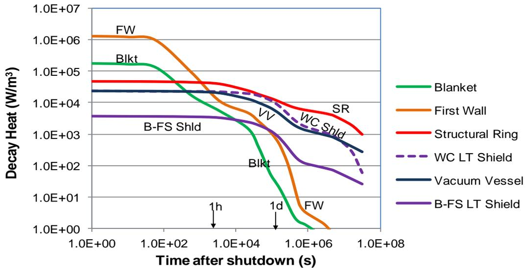
Fig. 8. Decay heats in inboard components.
