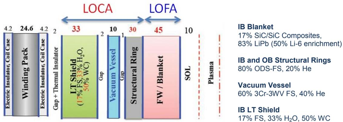
Fig. 4. Schematic of the inboard radial build with component material compositions with the tungsten carbide filler in low temperature shield.
