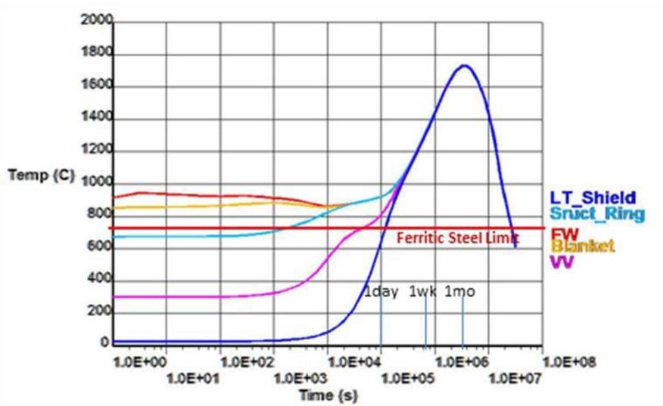
Fig. 10. Transient temperatures at midplane of inboard components after LOCA without cross-channel radiation modeled.
