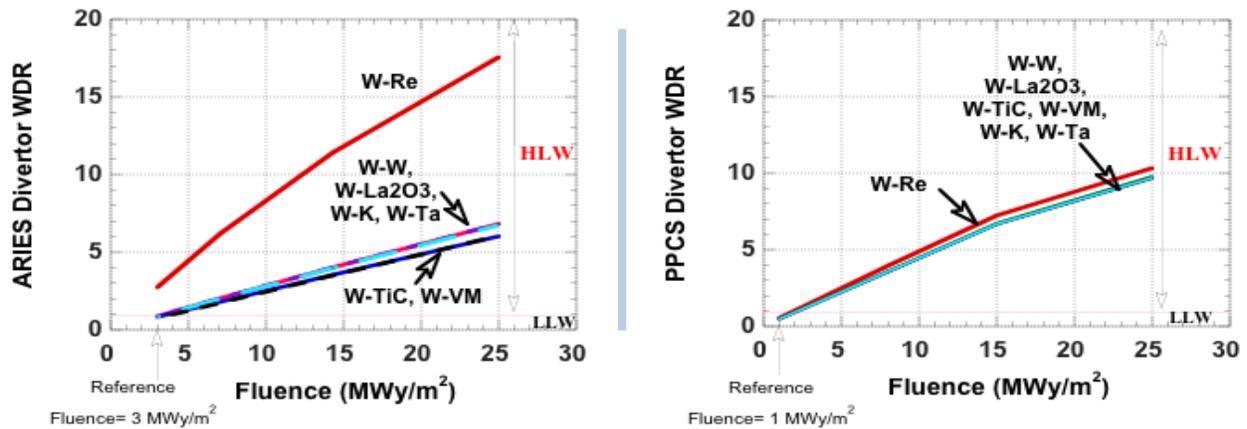
Figure 20. Waste disposal ratings of W-based alloys versus fluence for the ARIES and the PPCS divertors.
