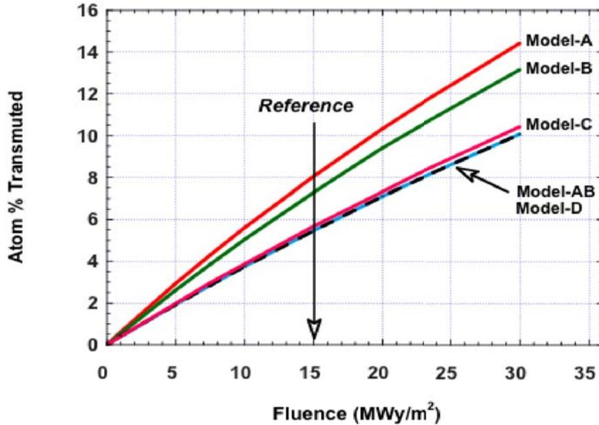
Figure 26. Percentage of W transmuted in the first pure W protective armor of different PPCS models versus fluence.
