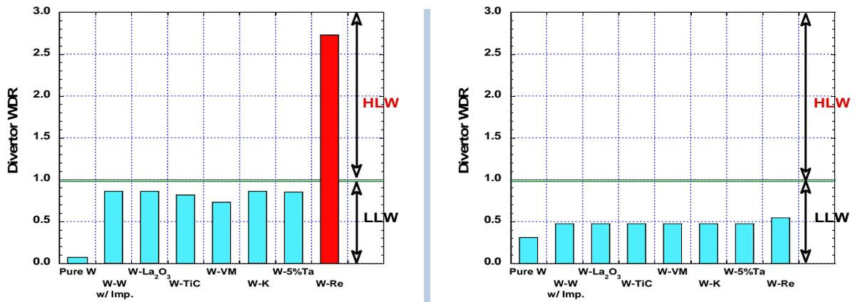
Figure 19. Waste disposal ratings of compacted ARIES and PPCS divertors at the end of 3 MWy/m<sup>2</sup> and 1 MWy/m<sup>2</sup> fluences, respectively.
