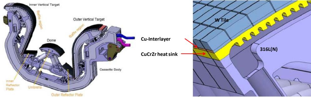
Figure 2. ITER divertor cassette (picture on the left) and detail of the dome components (picture on the right).
