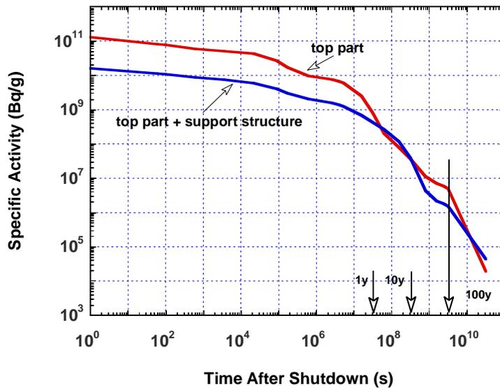
Figure 6. Specific activity versus time after shutdown of the top part of the divertor dome and the entire divertor dome (top part + support structure).
