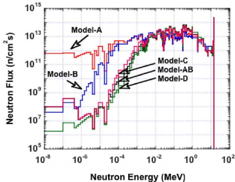
Figure 25. Neutron energy spectra in the W armor of PPCS models normalized to  $3 \text{ MW/m}^2$  NWL.
