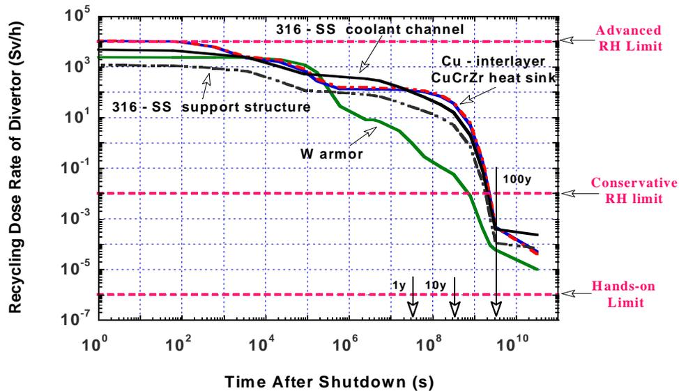
Figure 8. The recycling dose to the components of the ITER divertor dome versus time after shutdown after being exposed to a total fluence of 0.15 MWy/m<sup>2</sup> – the end of the divertor service lifetime.
