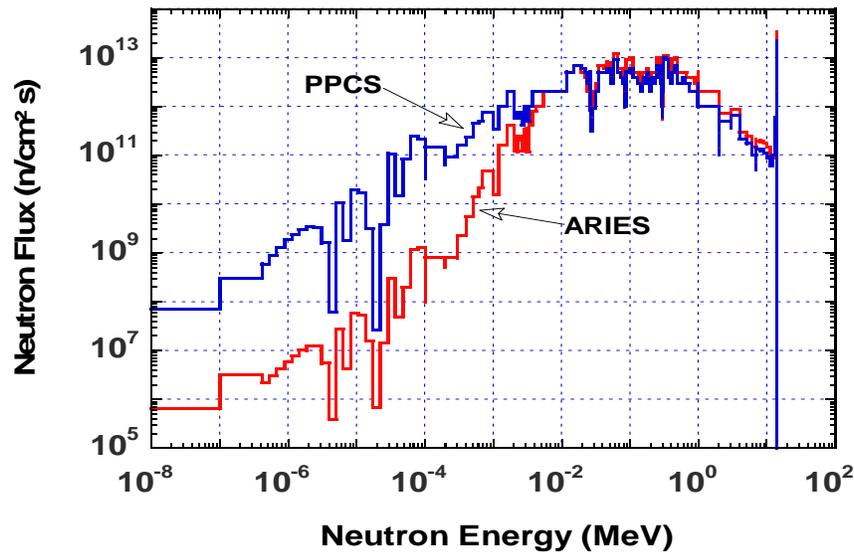
Figure 17. Comparison of neutron spectra in PPCS cooling channel 1 and front 2.4 cm of ARIES cooling channel.
