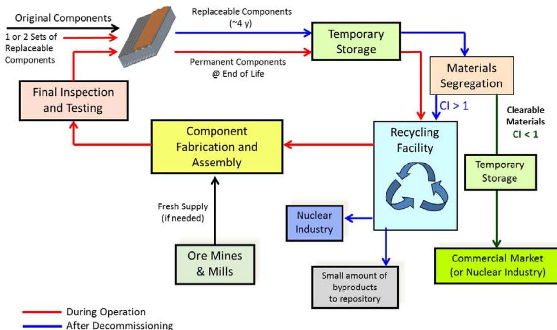
Figure 1. Recycling and clearance flow diagram.
