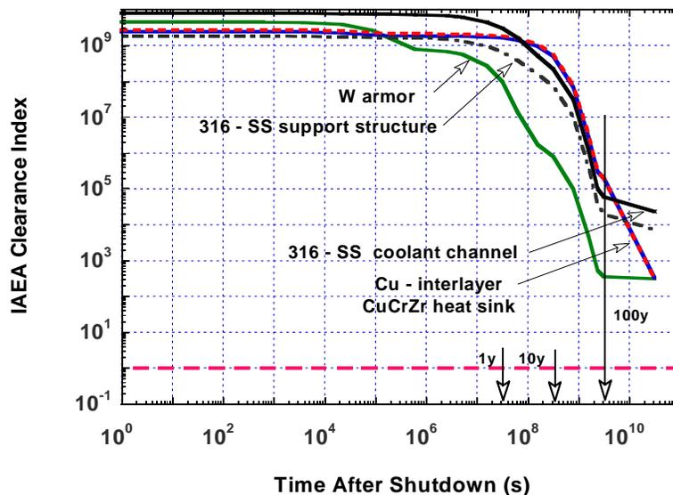
Figure 7. IAEA clearance index versus time after shutdown for the components of the ITER divertor dome after being exposed to a total fluence of 0.15 MWy/m<sup>2</sup> – the end of the divertor service lifetime.
