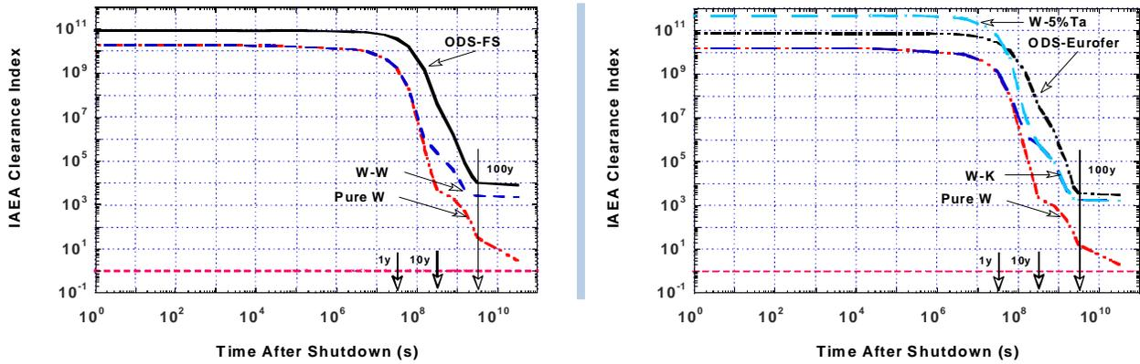
Figure 14. IAEA clearance index for W alloys of cooling channels.
