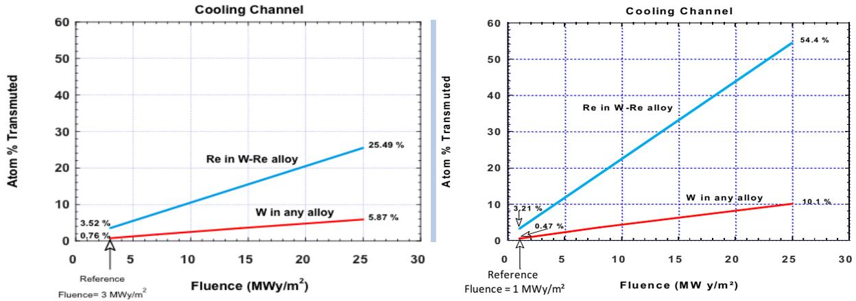
Figure 18. Percentage of W (in any W alloy) and Re (in W-Re) transmuted in cooling channels versus fluence for ARIES divertor (left) and PPCA divertor (right).
