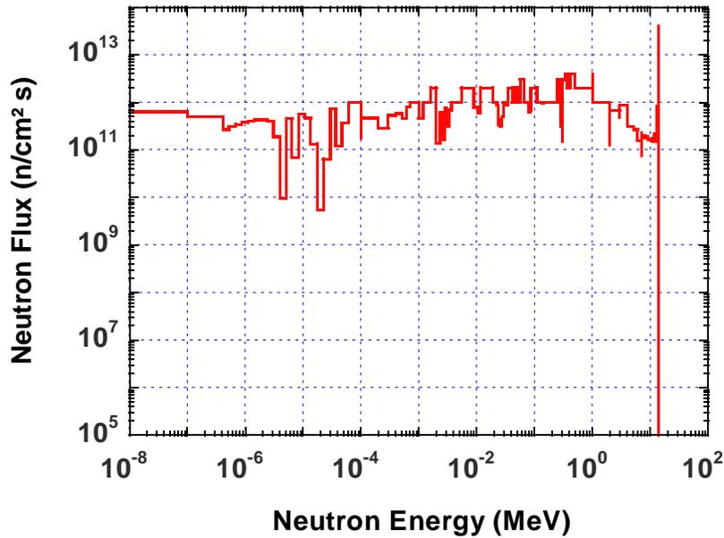
Figure 5. Spectrum in W armor normalized to 0.6 MW/m<sup>2</sup> NWL.
