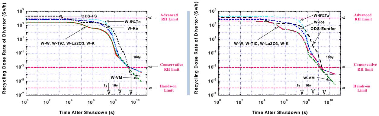
Figure 15. Recycling dose rate for W alloys of cooling channels.
