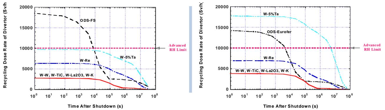
Figure 16. Recycling of W-alloy of cooling channels using a semi-log scale.
