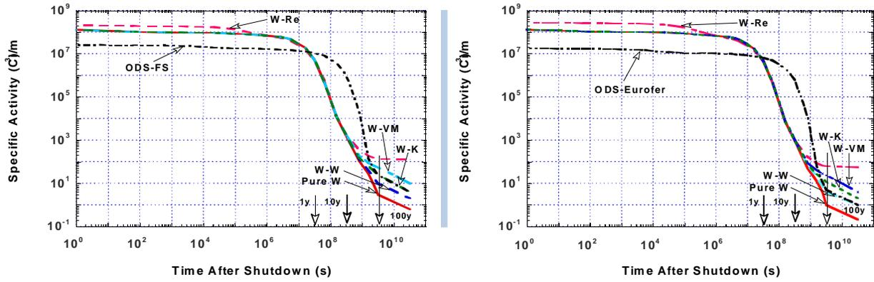
Figure 13. Specific activity of the W-alloys in cooling channels.
