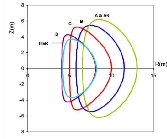
Figure 21. Sizes and shapes of plasma in PPCS models.
