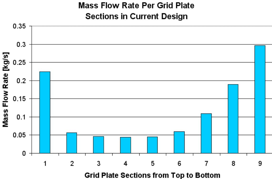
Figure 11. Results illustrating the uneven flow to the sections of the grid plate/divider assembly within the current design. Each section is a separate group of four channels except for section 9 with two channels.
