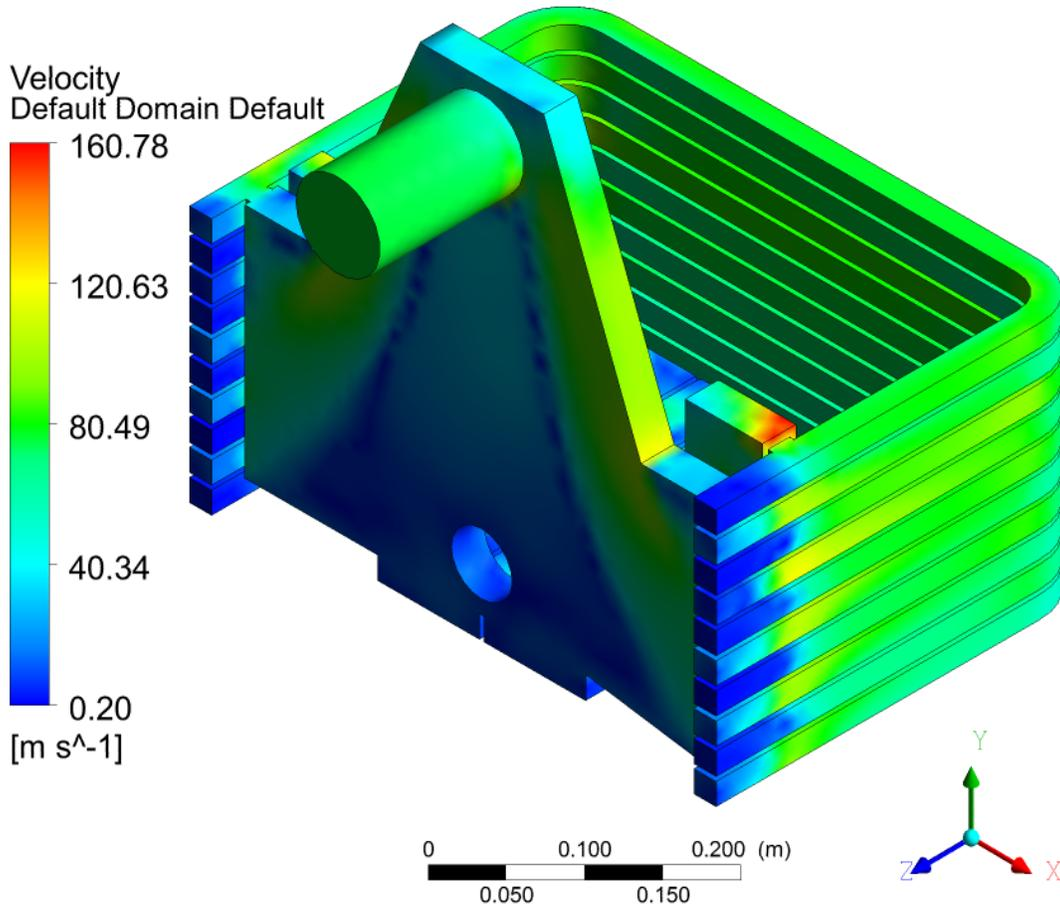
Figure 5. ANSYS CFX results illustrate the flow velocity within the improved design of the helium entry region within the TBM
