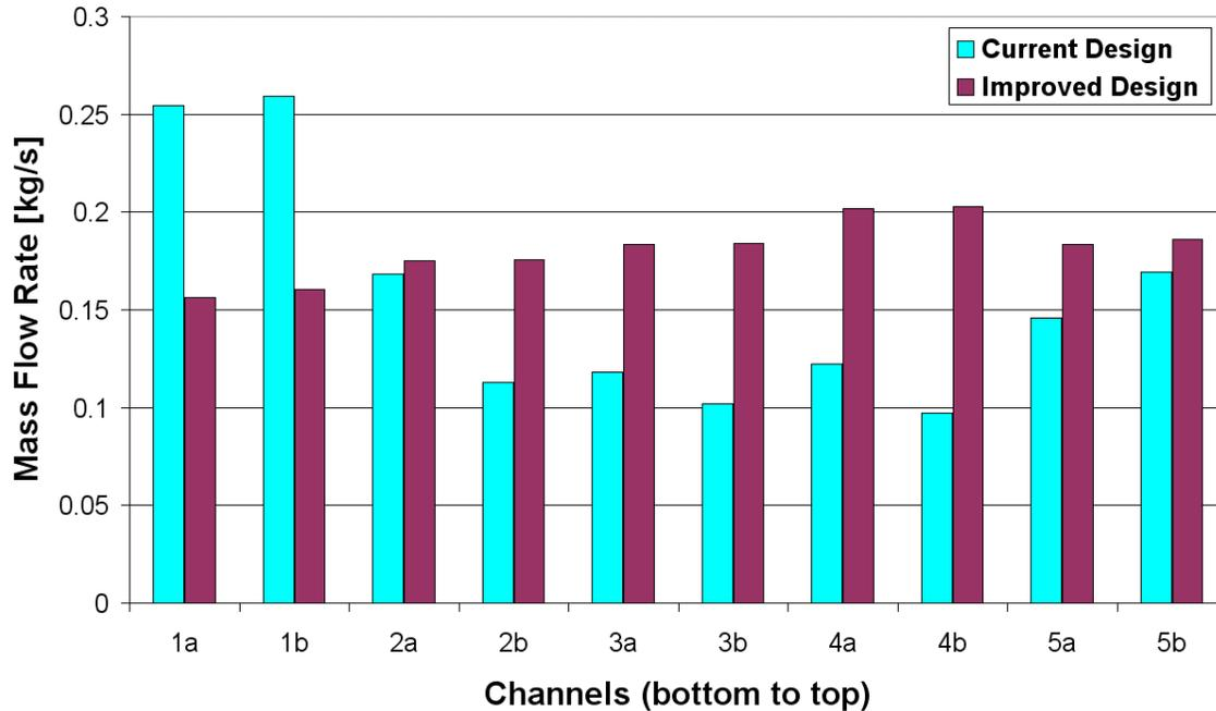
Figure 6. Mass flow rates for the first wall channels in the current design and improved design analysis results.
