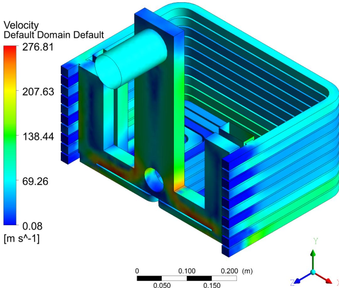
Figure 4. ANSYS CFX results illustrate the flow velocity within the current design of the helium entry region of the TBM.
