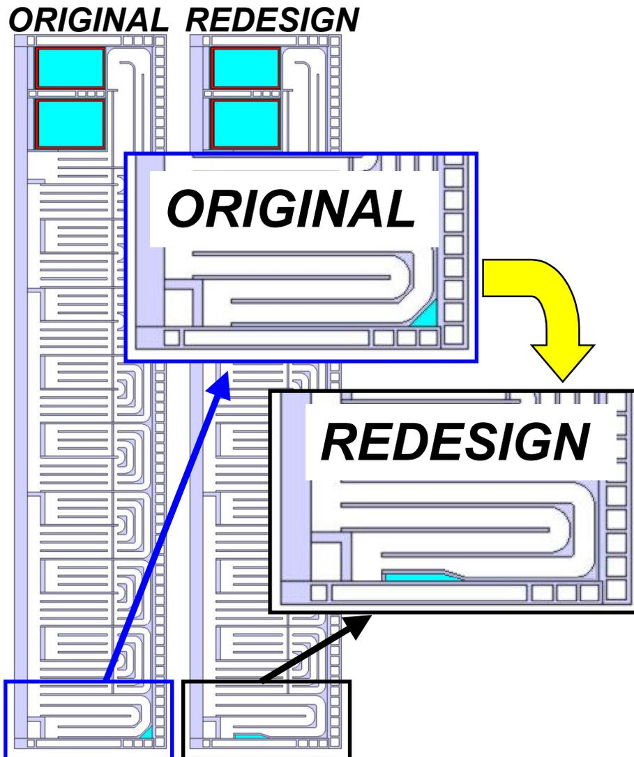
Figure 2. Illustrating the local solution to improve the hot spot in the PbLi due to neutron and gamma heating.
