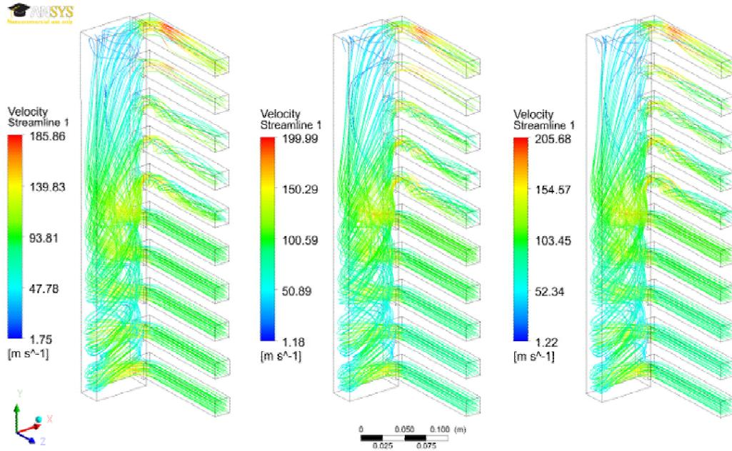
Figure 8. Velocity streamlines from analysis of the current header design.
