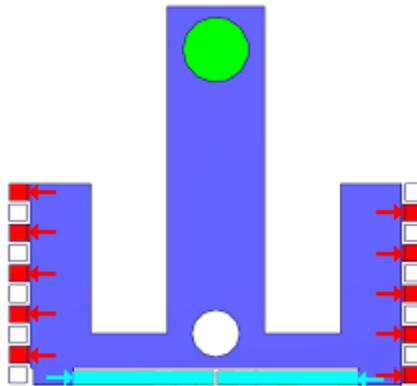
Figure 3. An illustration of the cause of flow asymmetry in the helium entry region. Green represents the entry tube, red represents flow to the first wall channels, light blue represents flow to the bottom plate.
