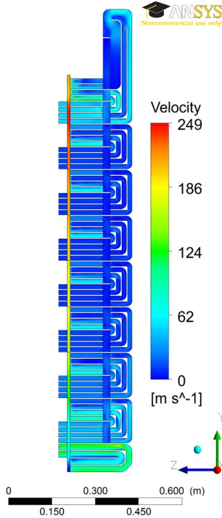
Figure 12. ANSYS CFX results for helium velocity within the grid plate/divider assembly of the current design.
