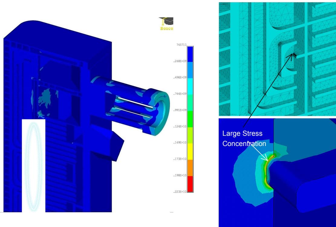
Figure 9. An illustration of the high structural stress within the grid plate/divider assembly.
