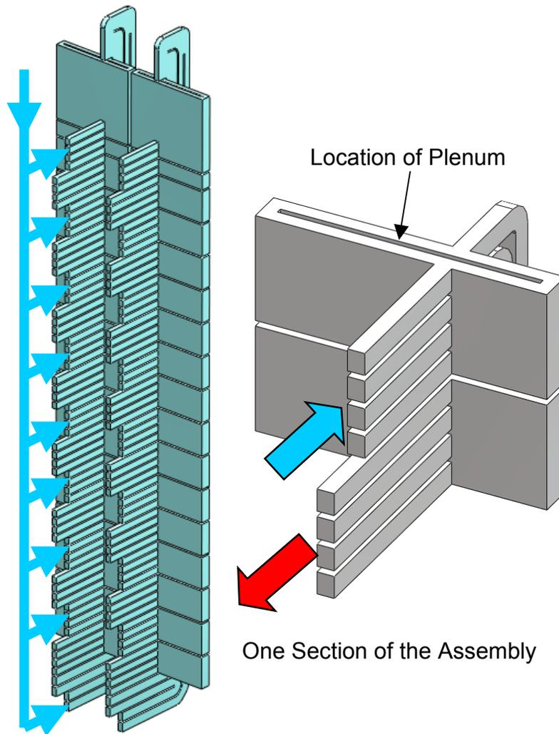
Figure 10. The grid plate/divider assembly showing the helium volume. Flow must enter 68 channels before following a complicated flow path.
