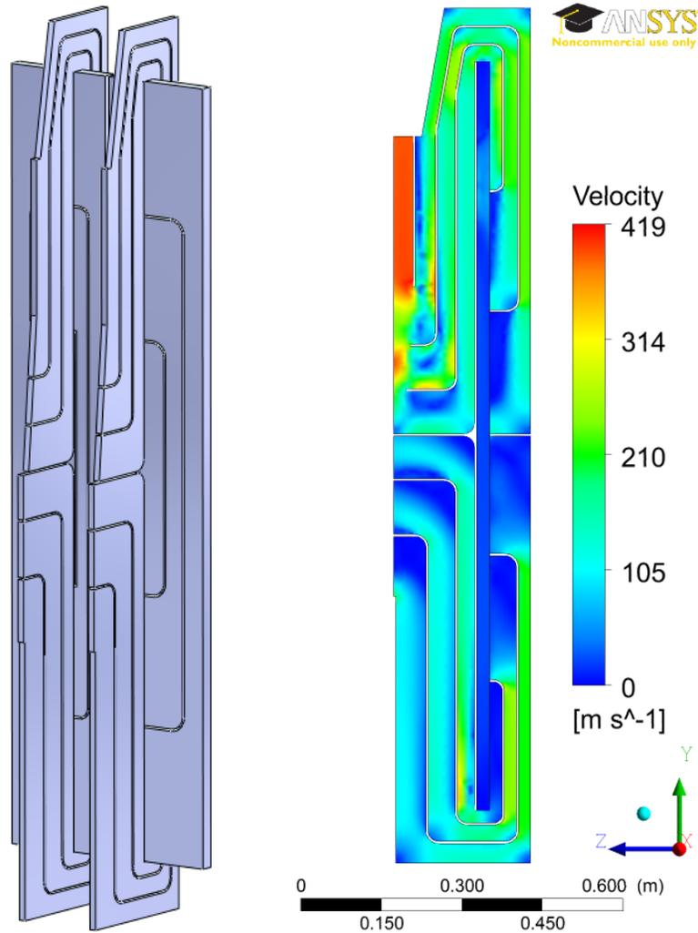
Figure 13. The geometry of the proposed redesign for the grid plate/divider assembly (left) and the ANSYS CFX results for helium velocity within the redesigned assembly.
