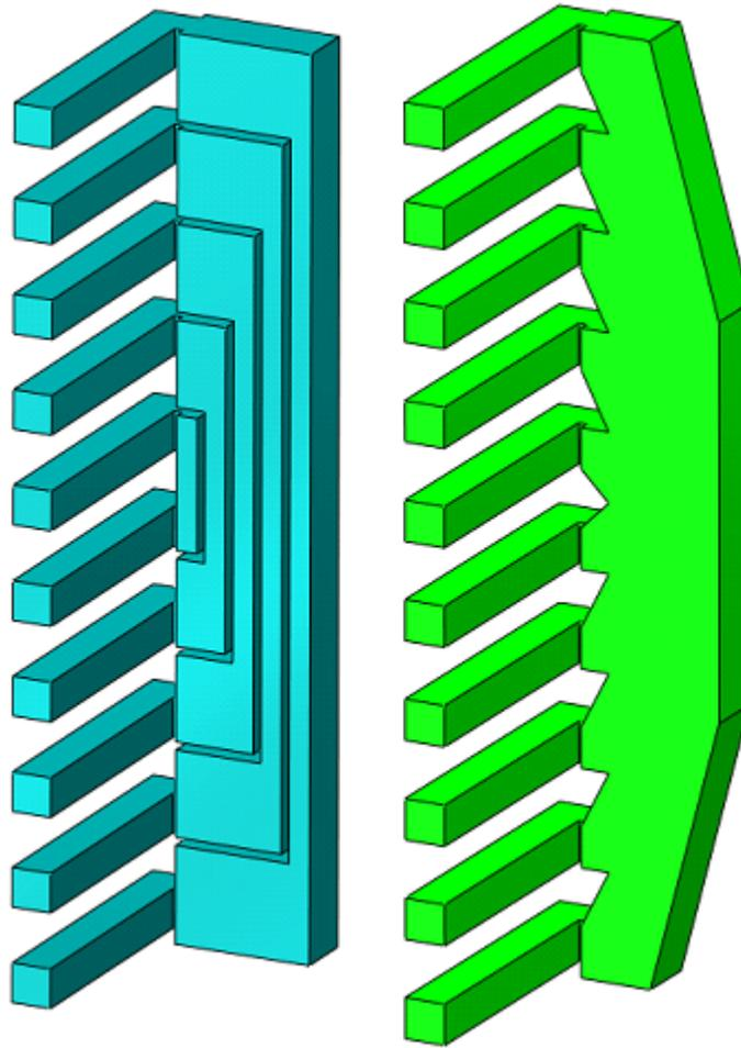
Figure 7. Two potential header design improvements: Left – Flow Continuation, Right – Flow Steering.
