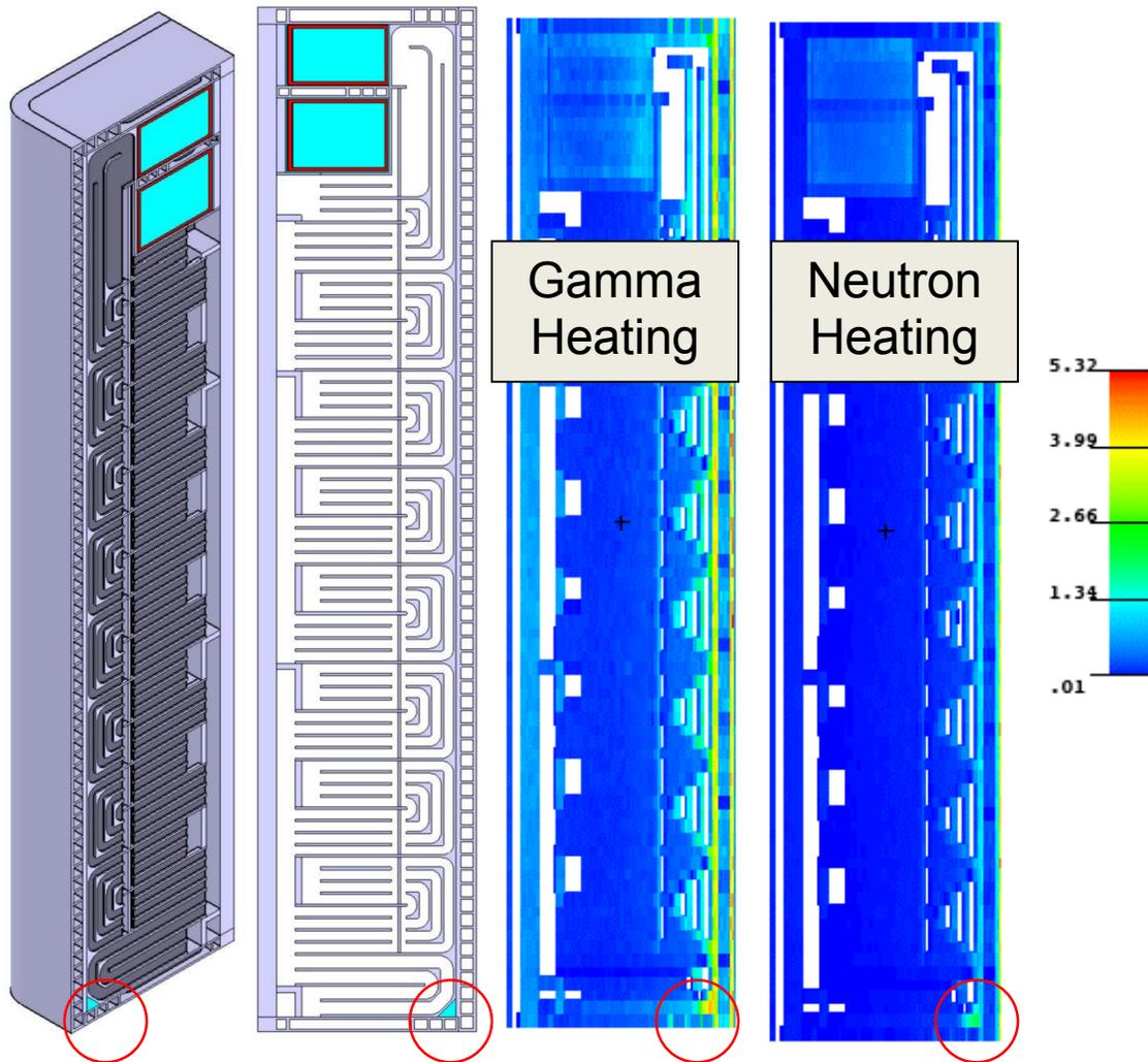
Figure 1. Neutronics results illustrating the elevated neutron and gamma heating in the stagnant PbLi channel location.
