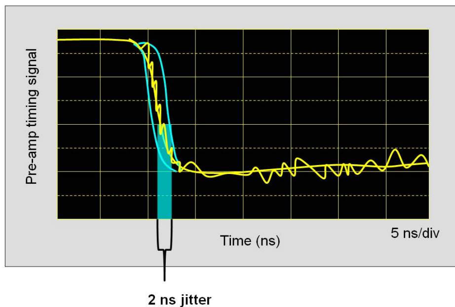
Figure 11.4 Timing jitter of Pre-Amplifier caused by thermal noise in circuitry. Jitter causes a level of uncertainty in the timing signal of approximately 2 ns.
