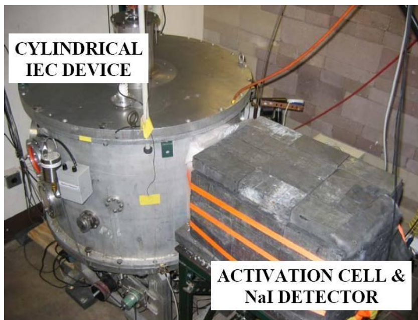
Figure 4.11 : UW IEC chamber and Wehmeyer explosive detection setup [15].
