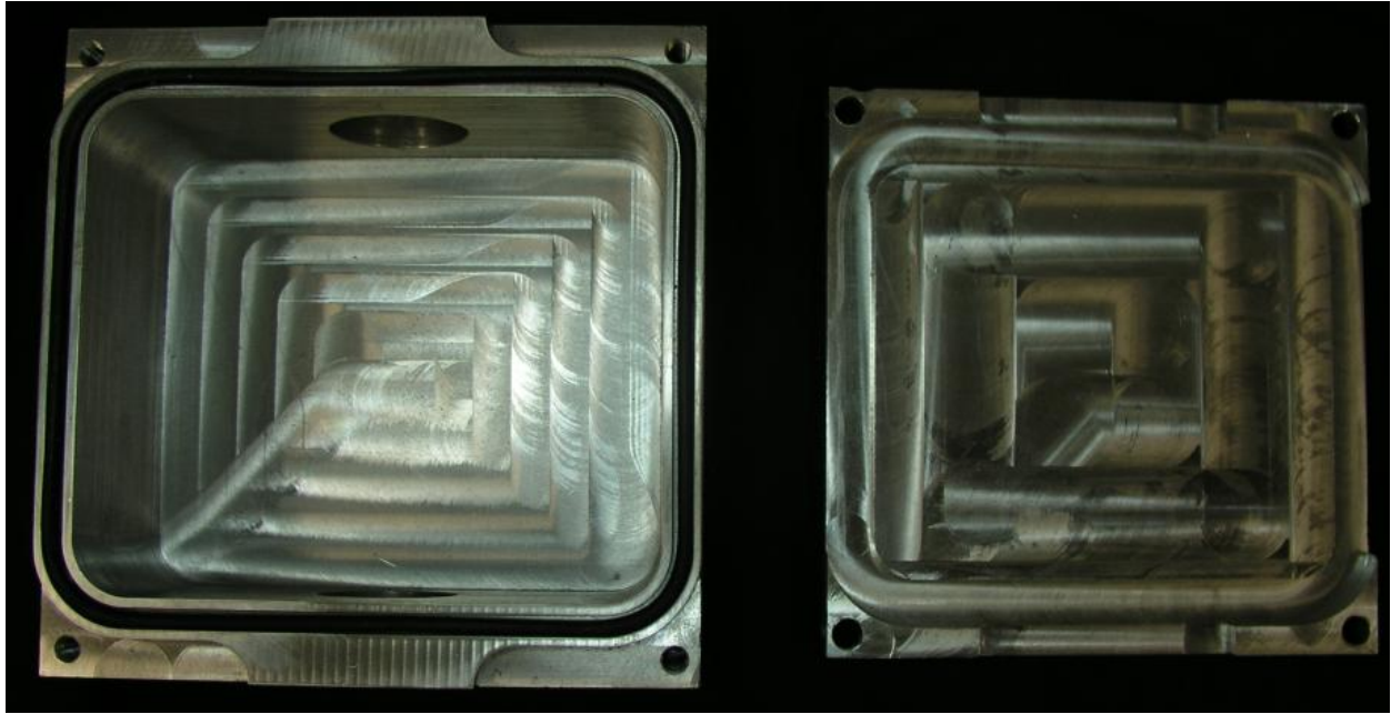
Figure 10.2 X-ray trap used in adjustable arm assembly. Constructed from aluminum, utilizes O-ring seals on the lid and all ports to seal the trap to high vacuum conditions.
