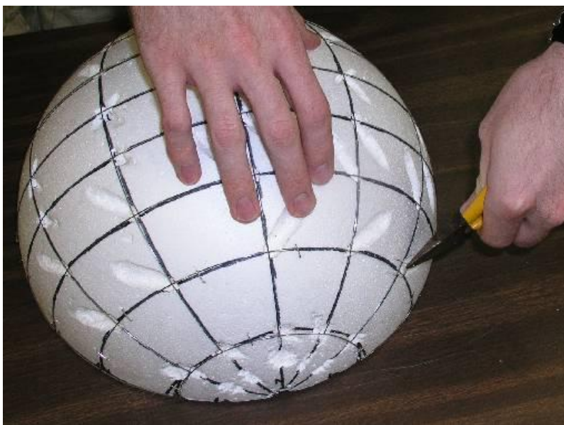
Figure 7.17: Construction of 30 cm diameter anode.
