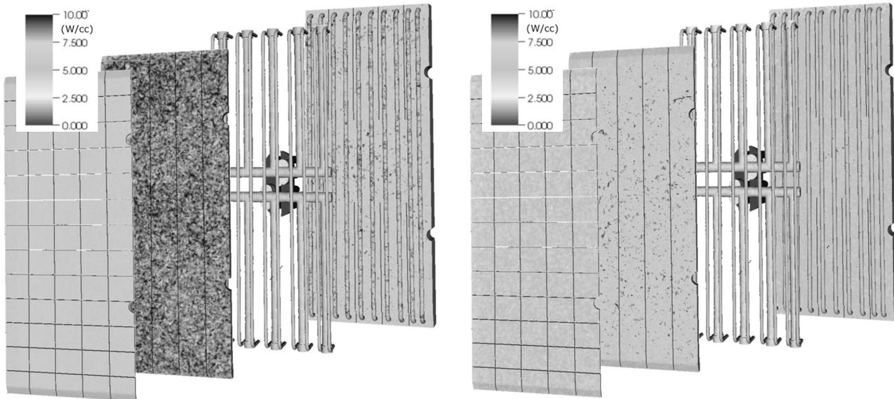
Fig. 7. Module 13 FW heating in the cylindrical hybrid model (left) and surface source model (right).
