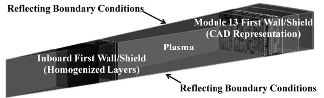
Fig 2. 1-D/3-D cylindrical hybrid model.
