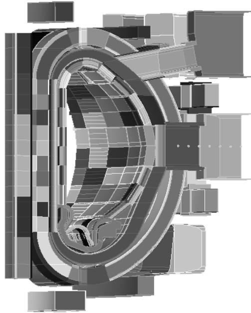
Fig. 3. 3-D model of the 40° sector of ITER.
