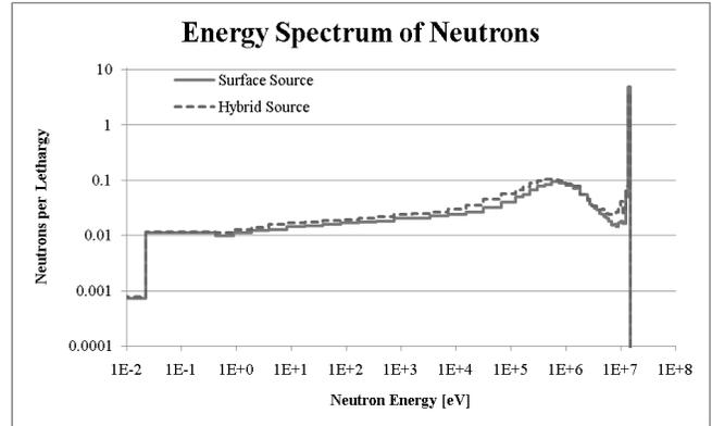
Fig. 6. Normalized neutron and gamma photon energy distribution incident on Module 13.
