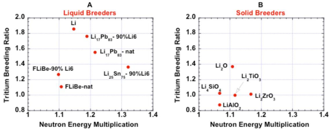
Fig. 4. Local TBR vs. energy multiplication for selected liquid and solid breeders (100% dense materials at room temperature evaluated with FENDL-2.1 data [18]). Natural Li<sub>25</sub>Sn<sub>75</sub> (not shown) provides a very low TBR (0.45). Note that some breeders may contain a neutron multiplier (e.g., Pb in LiPb and Be in FLiBe).
