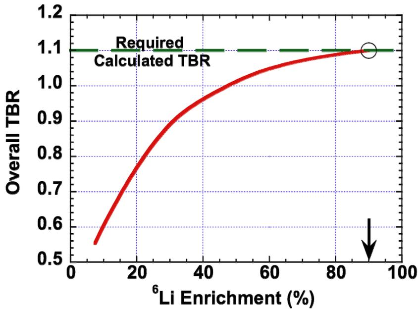
Fig. 10. Sensitivity of TBR to  $^6\text{Li}$  enrichment for ARIES-AT LiPb/SiC blanket [31].
