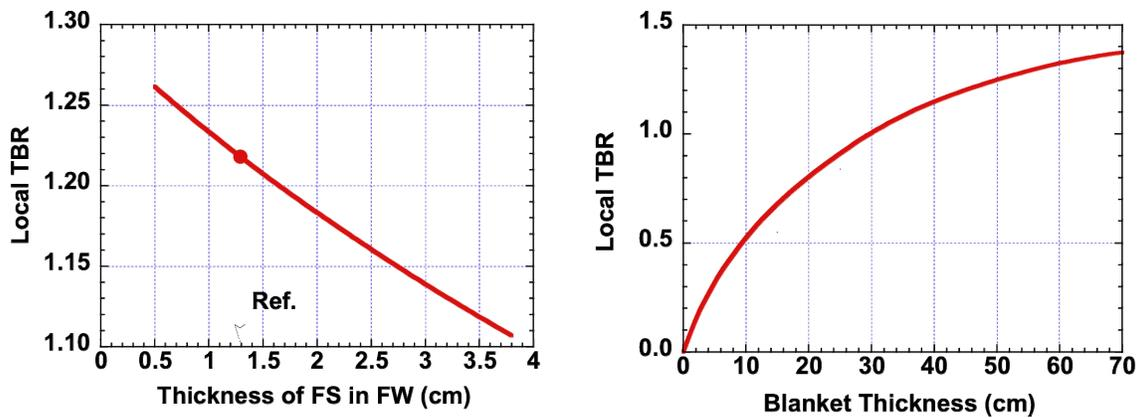
Fig. 7. Sensitivity of TBR to FW and blanket thickness of ARIES-CS [29].
