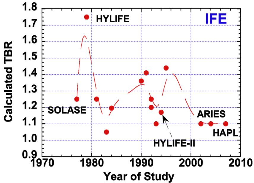
Fig. 1. Evolution of calculated TBR for U.S. MFE and IFE fusion power plant designs. The dashed curve is included just to guide the eye.
