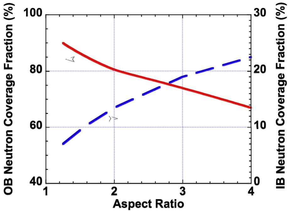
Fig. 6. IB and OB coverage fractions (defined as fraction of source neutrons incident directly on FW) as a function of aspect ratio [32]. This plot confirms the importance of OB for breeding, particularly for devices with low aspect ratio.
