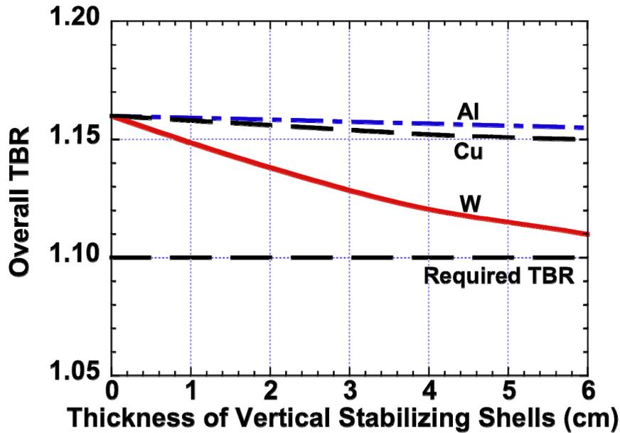
Fig. 8. Degradation of ARIES-AT TBR with thickness of stabilizing shell placed between OB blanket segments [31].
