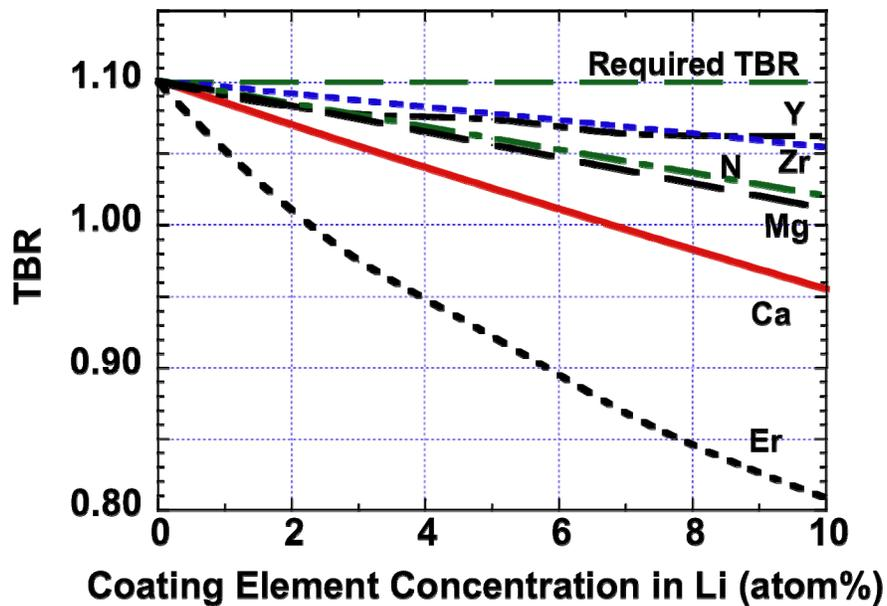
Fig. 5. Relative effect of coating materials on breeding of Li/V system [33].
