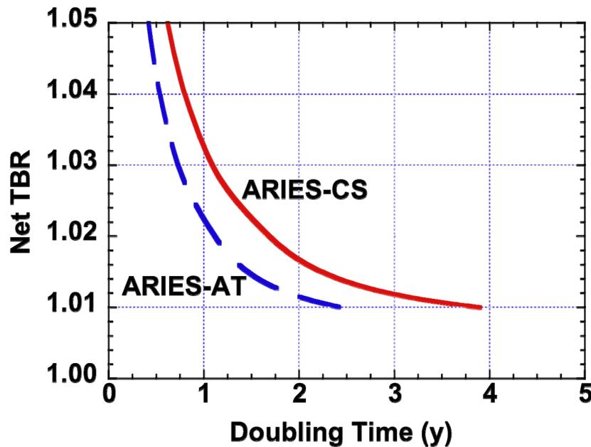
Figure 3. Sensitivity of Net TBR to doubling time.
