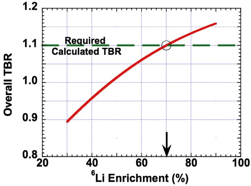
Fig. 9. Sensitivity of TBR to  $^6\text{Li}$  enrichment for ARIES-CS LiPb/He/FS blanket [29].
