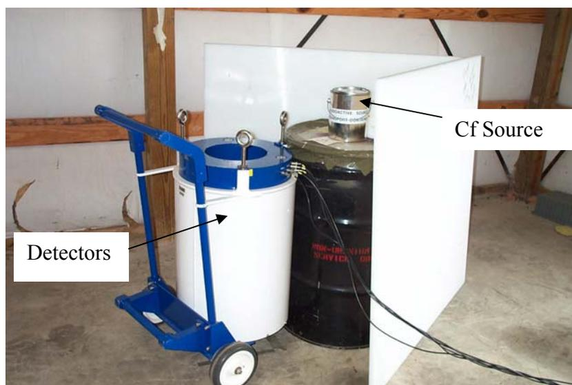
**Figure 2.7:** Photograph of active well coincidence counter setup at Savannah River [44].
