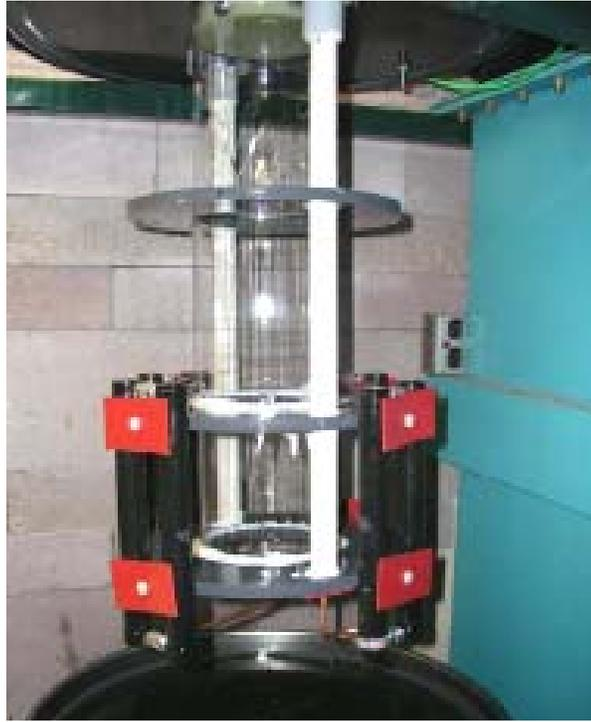
**Figure 4.4:** High-voltage buffer resistors.
