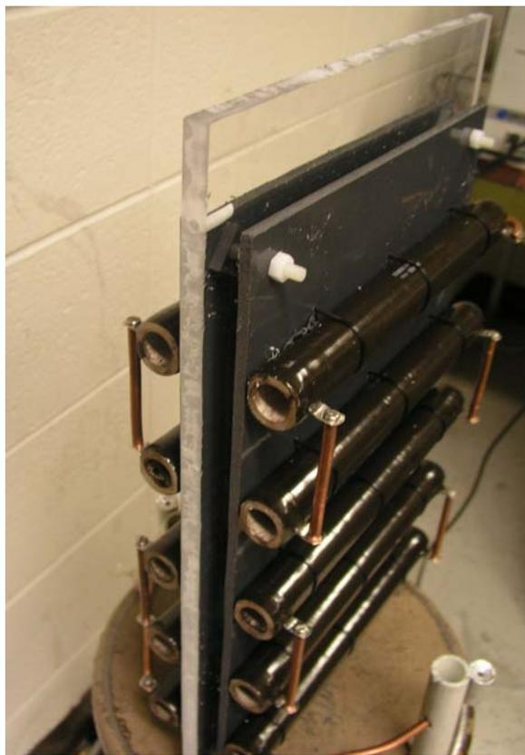
**Figure 4.15:** Buffer resistors for high voltage pulsing circuit.
