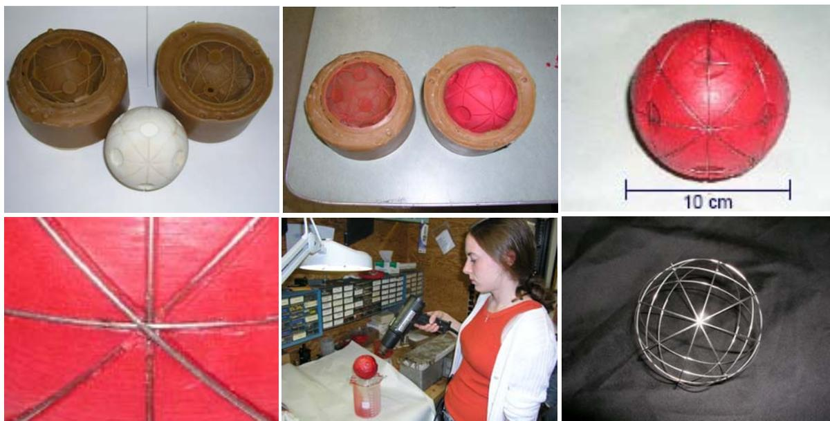
**Figure 4.7:** Grid construction procedure, (a) Mold produced from rapid prototype model, (b) Wax poured into mold, (c) Wires wound around wax form, (d) Wires spot-welded at junctions, (e) Wax form melted away at  $\sim 80^{\circ}\text{C}$ , (f) Completed cathode.
