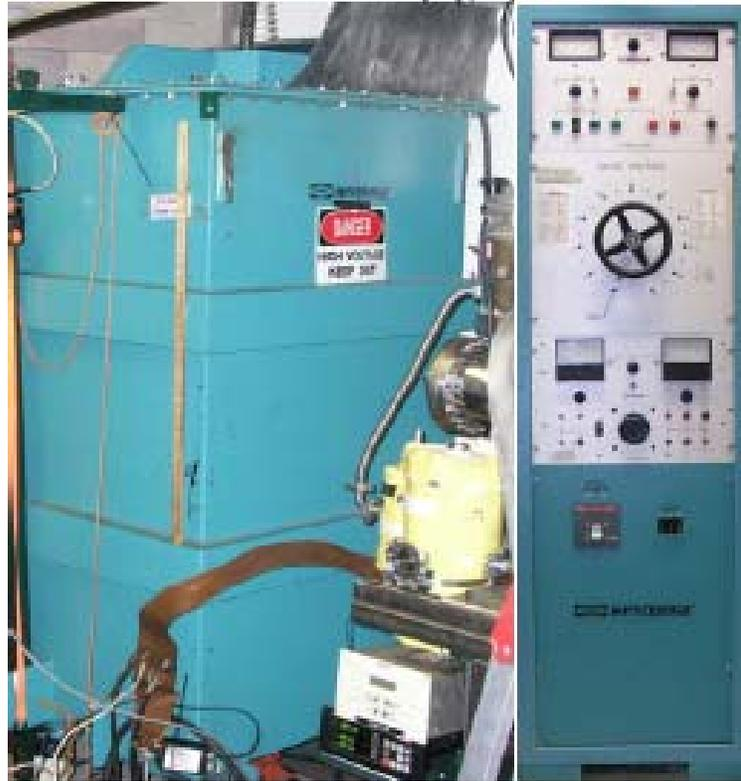
**Figure 4.3:** Hipotronics 8200-75 transformer (left) and controller (right).
