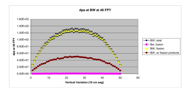
Fig. 6. Vertical variation of dpa along the 5 m high back wall (20 segments, 10 cm each).
