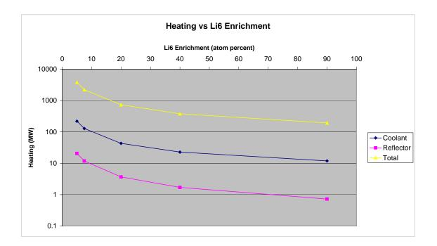
Fig. 13. Sensitivity of heating in Pb coolant and reflector and total heating to Li enrichment.
