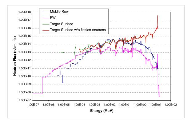
Fig. 17. Neutron flux spectra at FW and third row of tubes.
