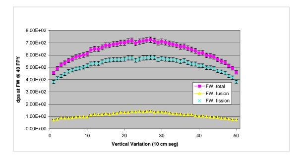
Fig. 3. Vertical variation of dpa along the 5 m high first wall (20 segments, 10 cm each).
