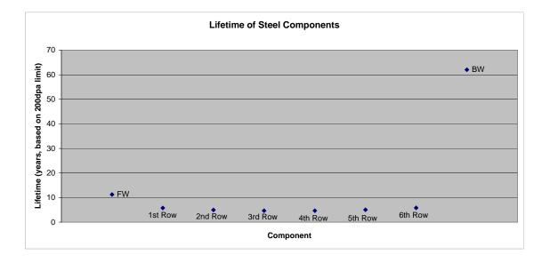
Fig. 5. Service lifetimes of FW, tubes, and back wall.
