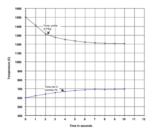
Fig. 15. Flibe and Pb temperature profiles.
