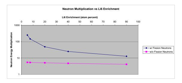
Fig. 14. Sensitivity of M<sub>n</sub> to Li enrichment.
