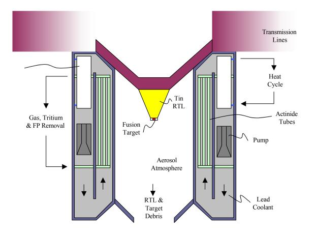
Fig. 1. Vertical cut through In-Zinerator showing actinide tubes and Pb pool.
