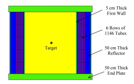
Fig. 2. In-Zinerator MCNP model.
