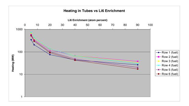
Fig. 12. Sensitivity of actinide mixture heating to Li enrichment.
