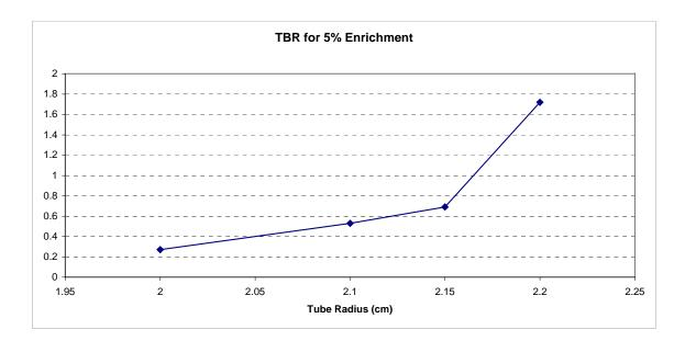
Fig. 9. Sensitivity of TBR to tube radius.
