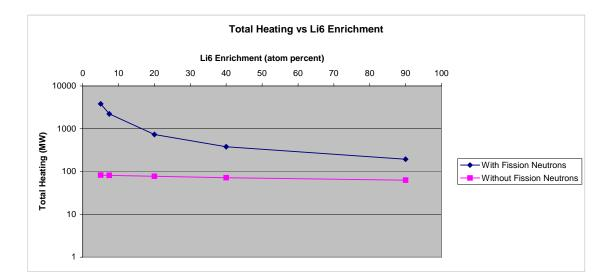
Fig. 11. Sensitivity of total nuclear heating to Li enrichment.
