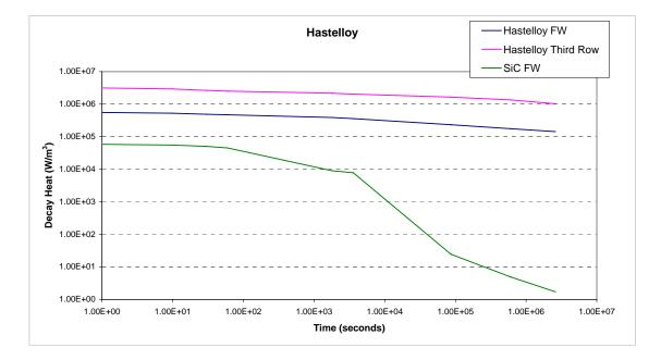
Fig. 18. Variation with time after operation of decay heats in Hastelloy FW and tubes of third row. The SiC FW is included for comparison.
