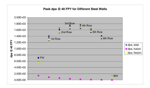
Fig. 4. Peak dpa at the midplane of the FW, tubes of 6 rows, and back wall.
