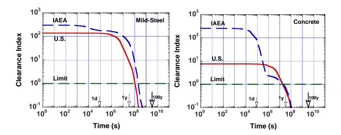
Fig. 1. Comparison of U.S. and IAEA clearance indices for steel and concrete of innermost segment of bioshield.
