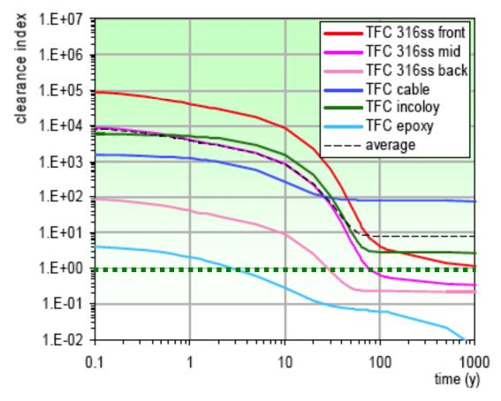
Fig. 3. CI time histories of the different TFC materials at the inboard midplane of PPCS-AB.
