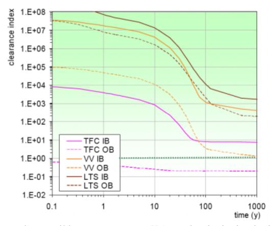
Fig. 2. CI time histories of lifetime components in PPCS-AB, at inboard and outboard midplane.
