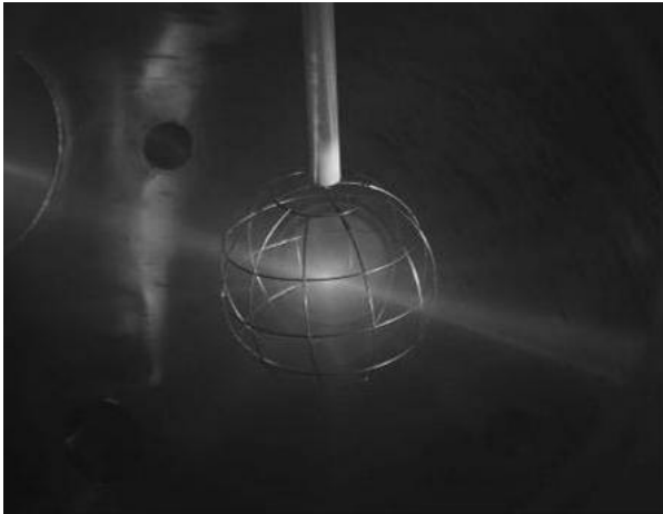
Figure 11: He beam discharging into IEC device at I_{\text{cath}}=10 mA, V_{\text{cath}}=30 kV, 20 mPa
