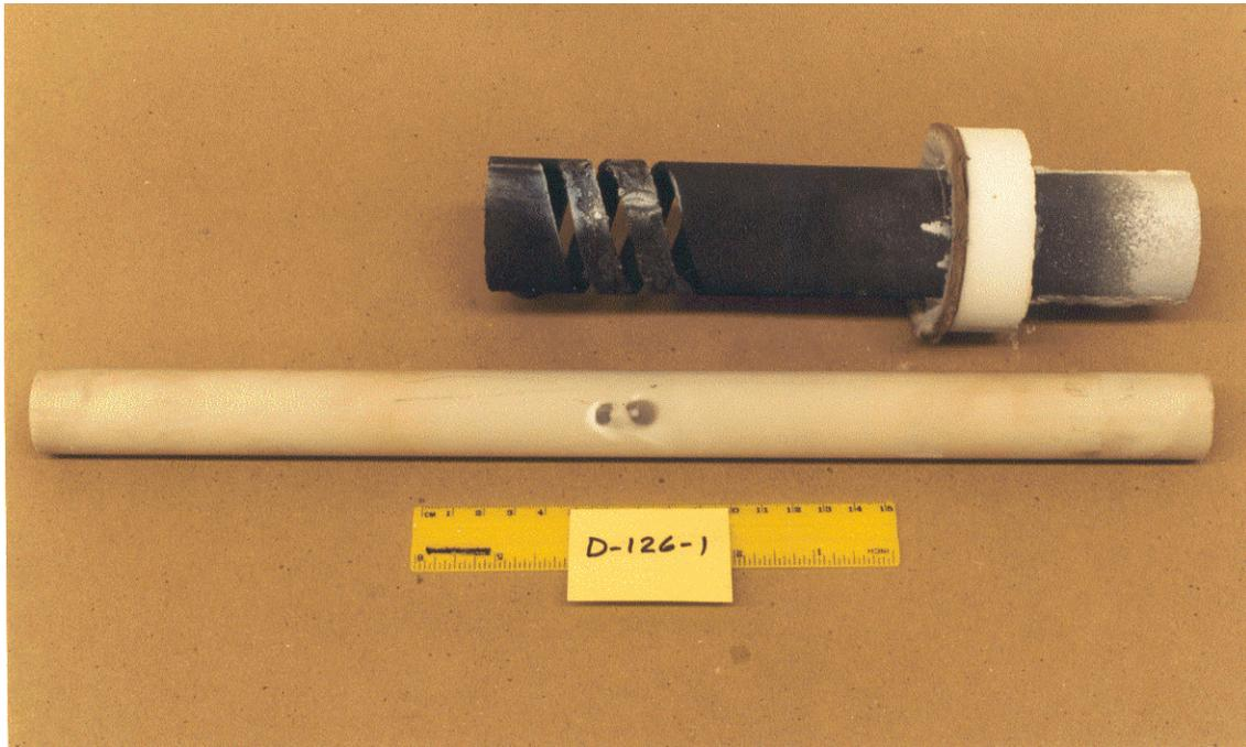
Figure C-5a. Photograph of the failed silicon carbide heating element and mullite furnace tube after Experiment D-126-1.
