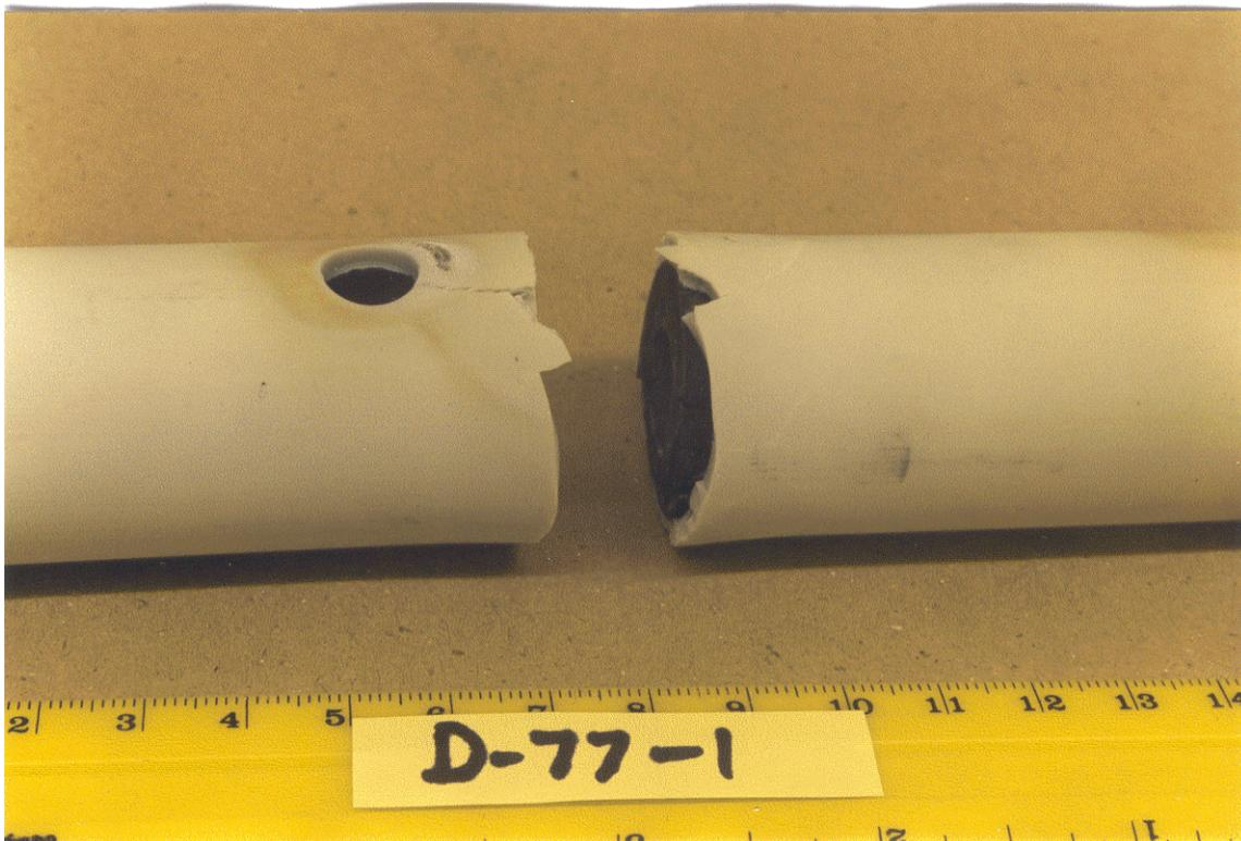
Figure C-2b. Photograph of the damaged mullite tube after Experiment D-77-1, close-up side view.
