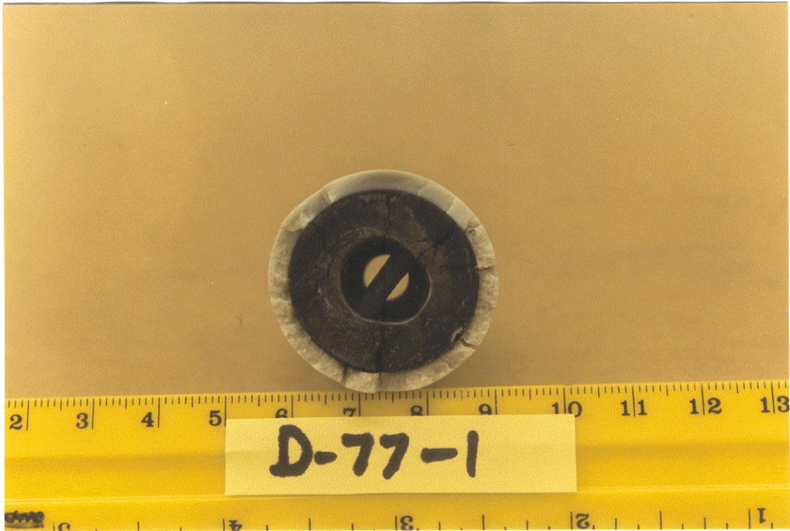
Figure C-2c. Photograph of the damaged mullite tube after Experiment D-77-1, close-up end view. In this view, note that no silicon remained in the graphite afterward, even though at least 3 g was present before the failure.
