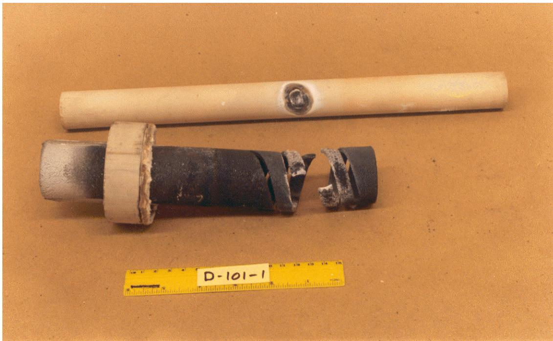
Figure C-3a. Photograph of the failed silicon carbide heating element and mullite furnace tube after Experiment D-101-1.
