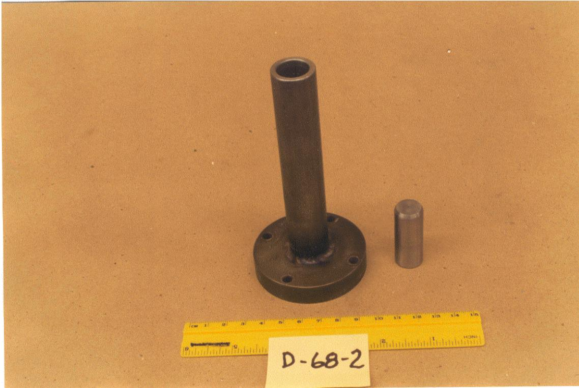
Figure 2a. Photograph of Impactor 3 during assembly.
