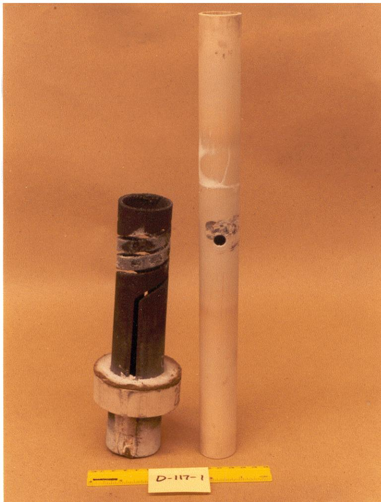
Figure C-4a. Photograph of the failed silicon carbide heating element and mullite furnace tube after Experiment D-117-1.
