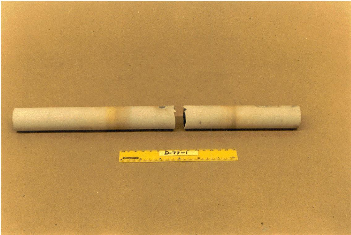
Figure C-2a. Photograph of the damaged mullite tube after Experiment D-77-1, overall side view.
