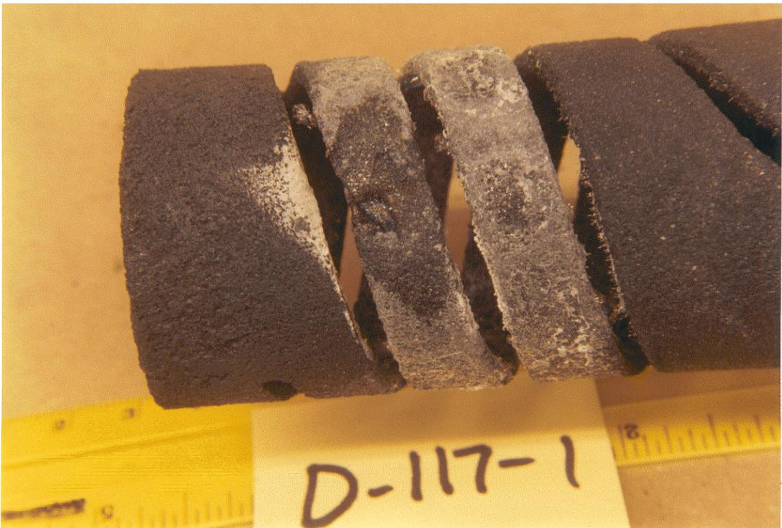
Figure C-4c. Photograph of the failed silicon carbide heating element after Experiment D-117-1.
