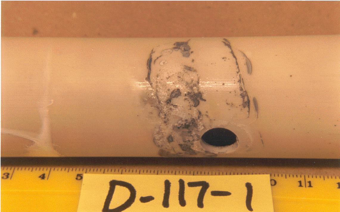
Figure C-4b. Photograph of the failed mullite furnace tube after Experiment D-117-1.
