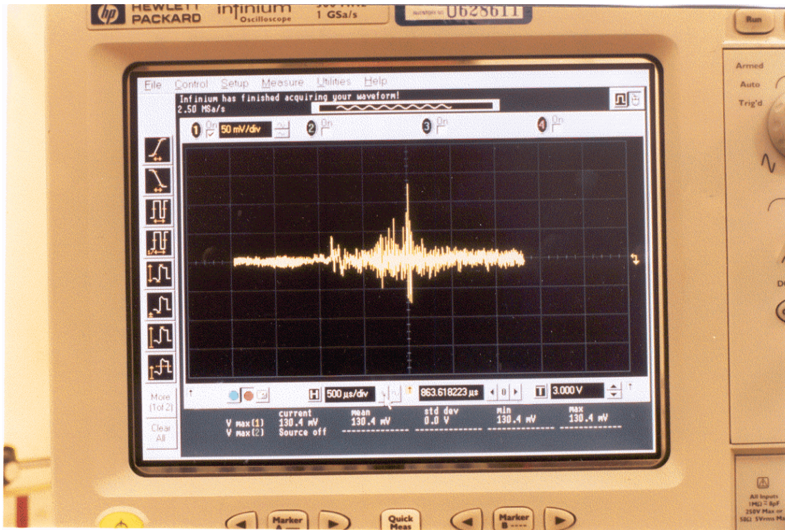
Figure 11. Typical oscilloscope trace recorded when the tourmaline transducer was impacted at 102 mm with a pressure pulse generated by the solenoid-driven impactor. The transducer was placed a few millimeters beneath the surface of the water with the surface of the impactor 102 mm below. The vertical scale is 50 mV / large division; the horizontal scale is 500 \mu s / large division. (C-256-1 #2)
