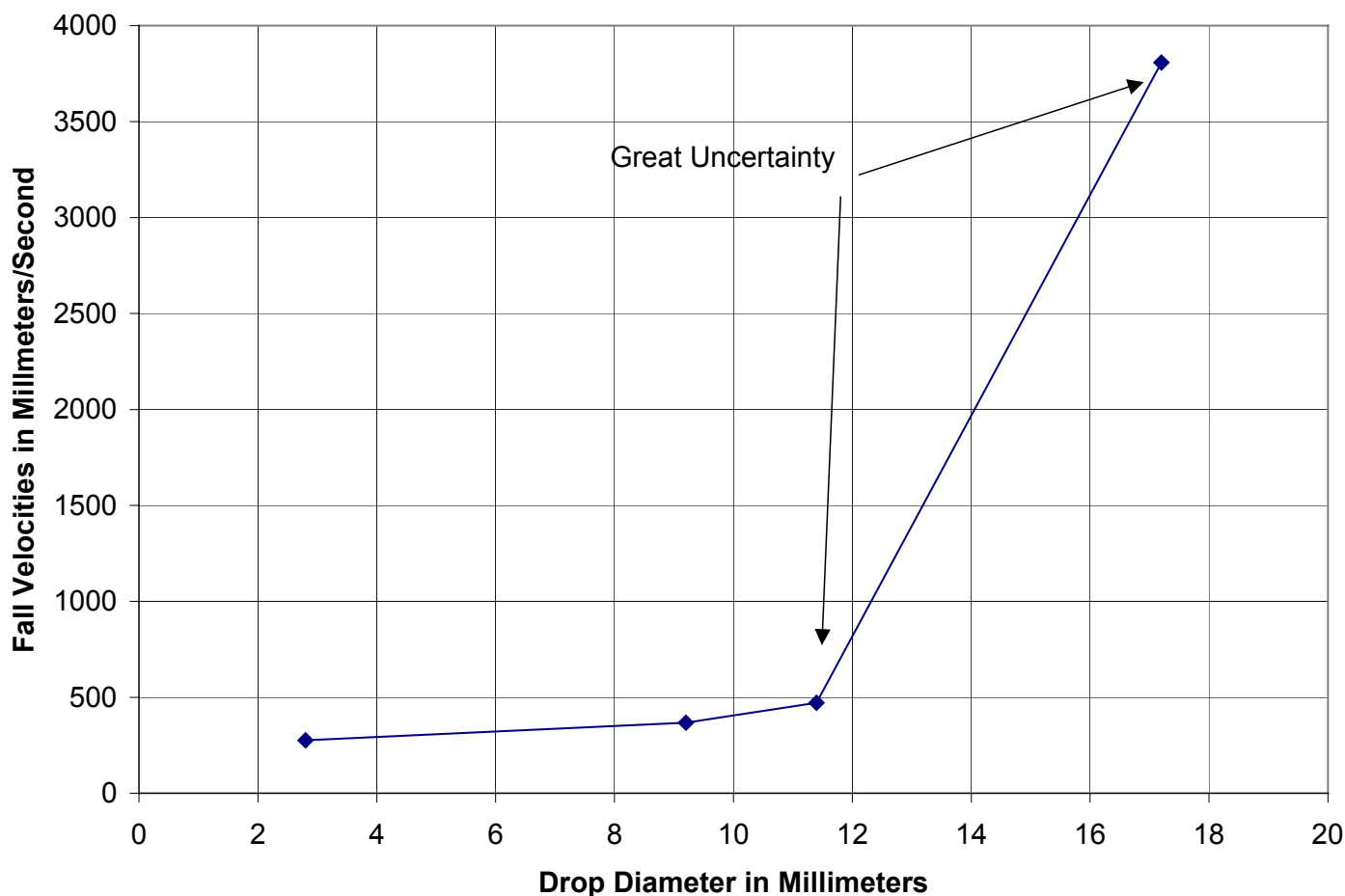
Figure 21. Fall velocities of molten ferrosilicon drops with several diameters released into room temperature water. The velocities were calculated as the slopes of the fall distance-time points plotted in Figure 20.
