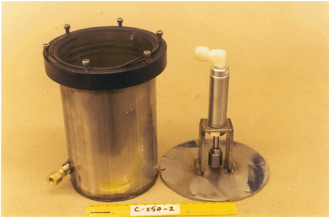
Figure 7. The piston and plate assembly and the canister used in the pneumatic impactor are shown before assembly. The 22.66 g weight has been threaded onto the driver rod. The piston is almost completely extended in this photograph. One of the two ports for passing an air line through the wall of the canister is visible at the lower left of the photograph. (C-250-2)
