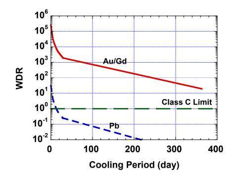
Figure 9. Effect of cooling period on waste disposal rating of hohlraum wall materials assuming continuous recycling over plant life without transmutation product removal.
