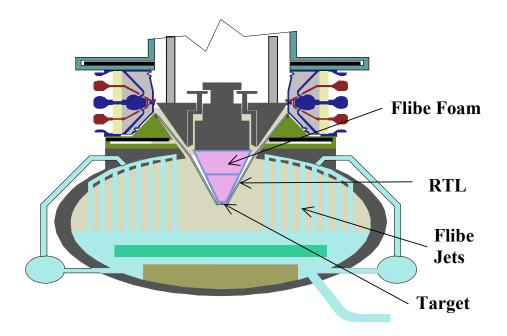
Figure 4. Z-pinch chamber and RTL connecting the target to the power supply.
