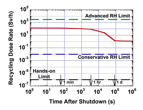
Figure 12. Reduction of dose with time after shutdown for no cooling period and without transmutation product removal.
