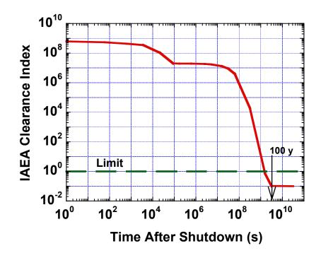
Figure 11. Variation of RTL clearance index with time after shutdown for no cooling period and without transmutation product removal.
