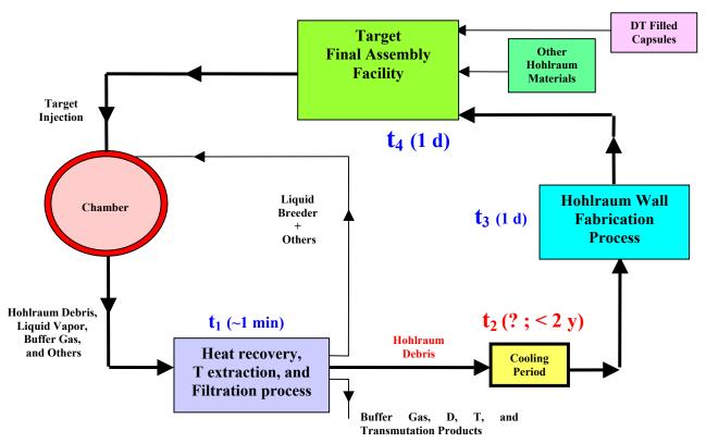
Figure 2. HI target recycling processes and proposed timeline.
