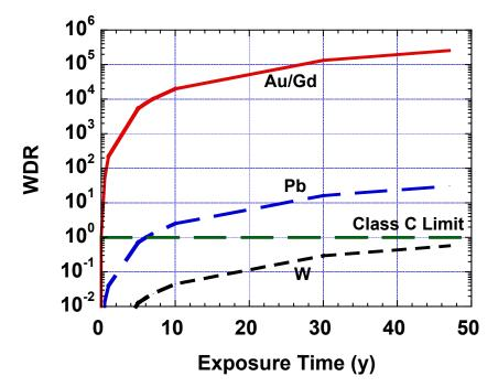
Figure 8. Increase of waste disposal rating of hohlraum wall materials with irradiation time for no cooling period and without transmutation product removal.
