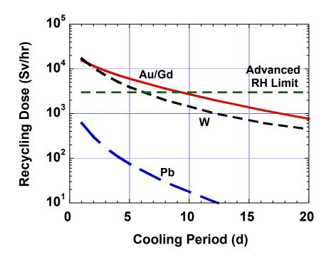
Figure 10. Effect of cooling period on recycling dose of hohlraum wall materials assuming continuous recycling over plant life without transmutation product removal.
