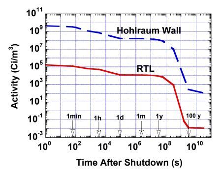
Figure 6. Comparison of activities of hohlraum wall and RTL made out of pure iron.
