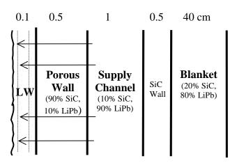
Fig. 1. Representative radial build and typical dimensions of essential components for the porous wall injection scheme (not to scale). A thick LiPbcooled shield follows the blanket.
