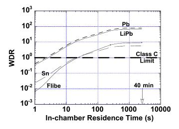
Fig. 2. Variation of liquid film WDR with in-chamber residence time for 47 y of operation without removal of transmutation products.
