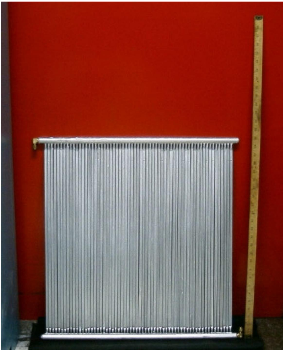
**Figure 3.8** – Picture of the Model ALM1 water containment apparatus. Note that the vertical tubes have been flattened to present a constant wall thickness to incoming protons.
