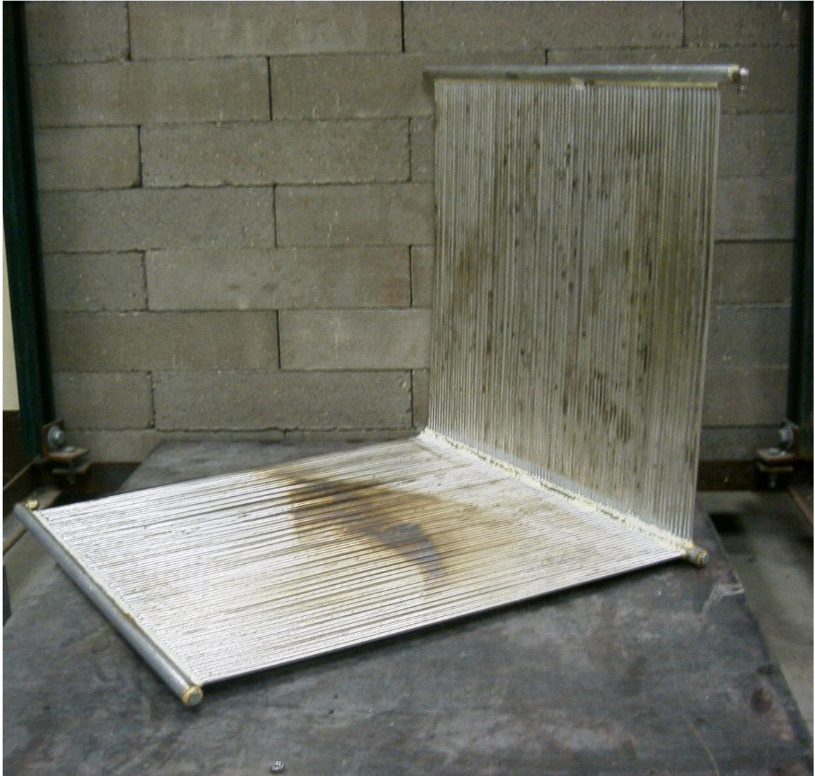
**Figure 3.13** – The Model ALM2 apparatus. This L-shaped apparatus was designed to have the horizontal panel fit below the anode, and the vertical panel fit between the anode and the IEC chamber wall. Numerous leaks developed in the joints of this apparatus, however, and it was retired after only a few weeks of testing.
