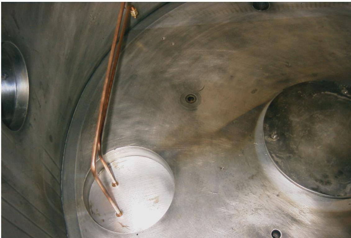
**Figure 3.9** – Photograph of plate through which the copper plumbing of the isotope production system passes. The copper tubes are fed through Swageloc™ fittings, which are screwed into the plate and their threads sealed with Torr Seal™. The fittings fix the copper tubes in place and provide a leak-tight seal.
