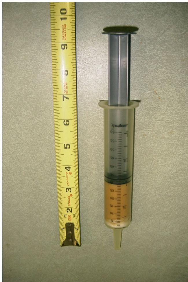
**Figure 5.2** – Photograph of resin column with ion exchange resin inside.
