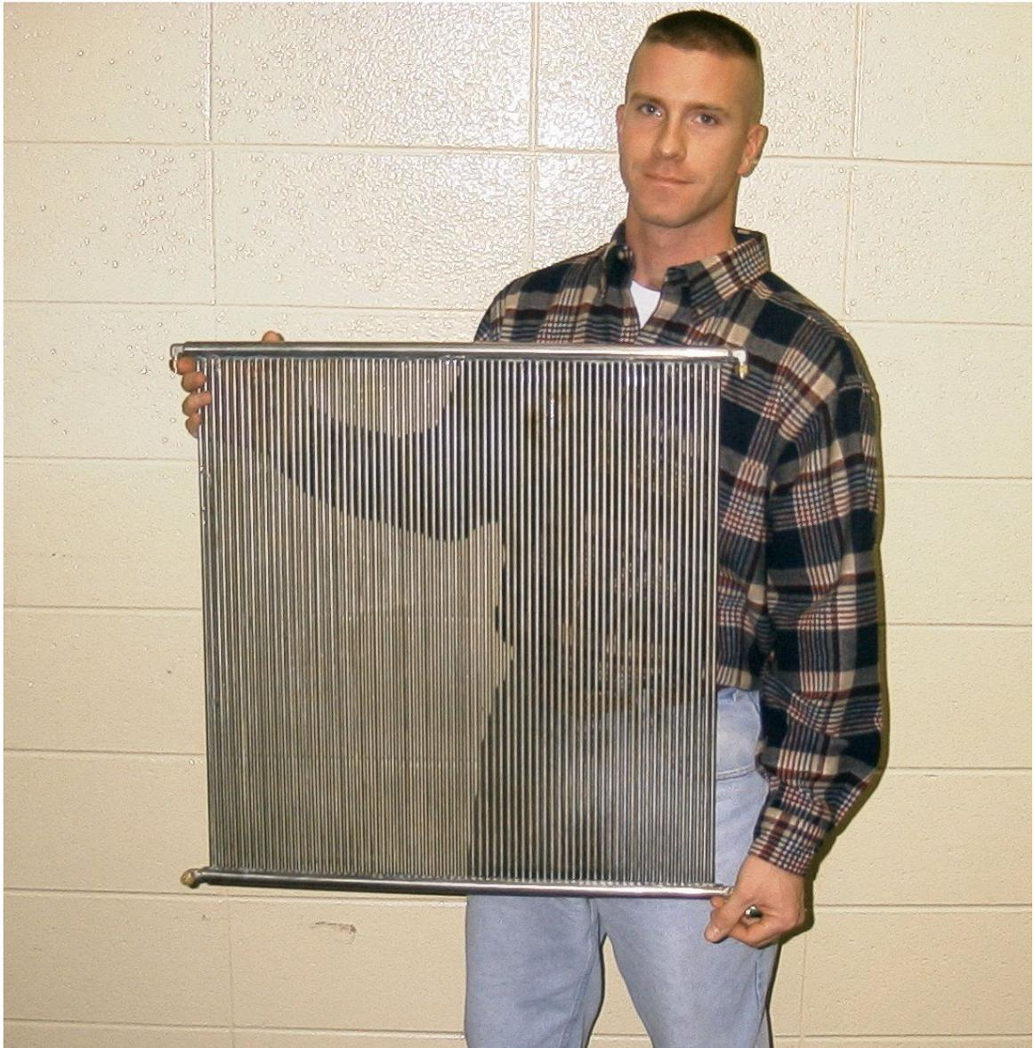
**Figure 3.15** – The Model SSM2 water containment apparatus. This model was constructed entirely from stainless steel and used tubes with 0.013 cm thick walls. The tubes were soldered to the manifold creating a rugged, high temperature joint.
