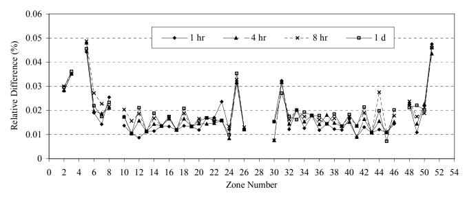
Figure 2. Relative difference (%) between the 100-pulse hybrid approximation and the exact pulsing solution at different cooling times.
