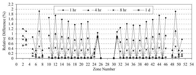
Figure 1. Relative difference (%) between the steady-state approximation and the exact pulse solution at different cooling times.
