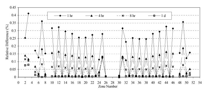
Figure 4. Relative difference (%) between the results from schedule 8 and the exact pulse schedule at different cooling times.
