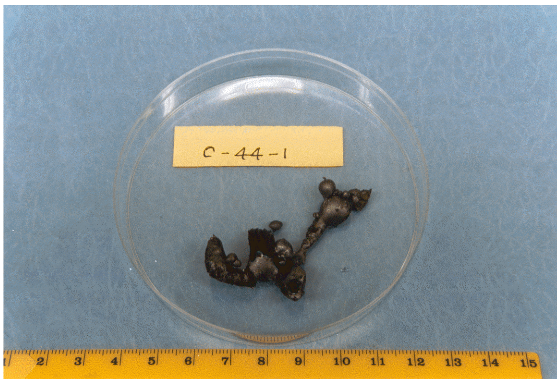
Figure 18. Strange-looking globule produced in experiment C-44-1. Water temperature was 21.1 °C. The scale is divided into millimeters.
