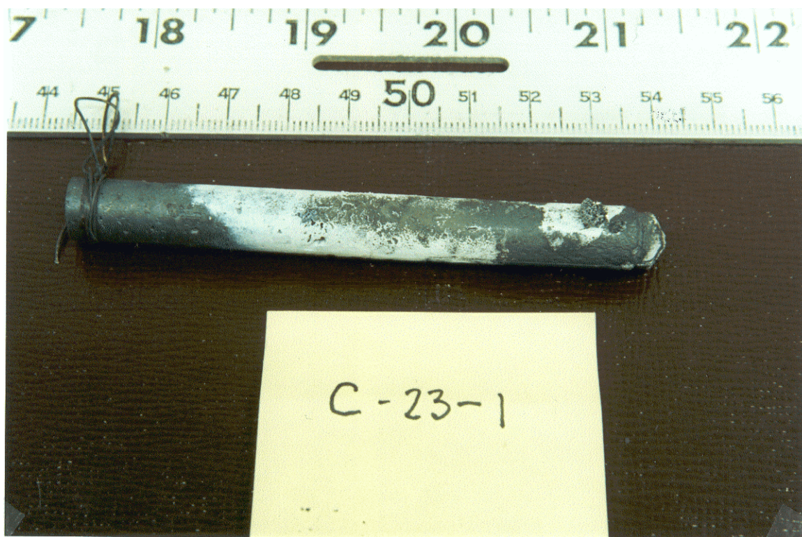
Figure 5. Ferrosilicon rod that had been heated to about 1550 °C in a high alumina furnace tube before cooling to room temperature. The rod was kept in flowing cylinder argon at all times. Notice the powdery white deposit on the sides of the rod. Notice also the rosette of solidified melt near the right end of the rod. The scale immediately above the rod is divided in millimeters. (C-23-1)
