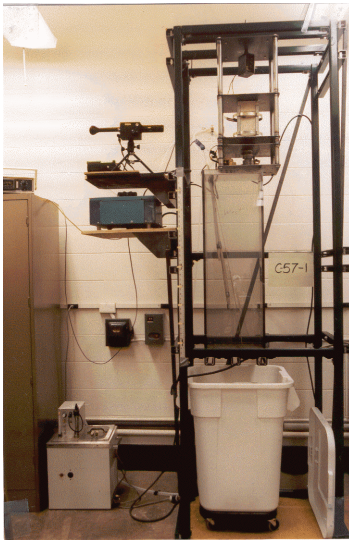
Figure 1. Photograph of the 3 m-tall tower in which the ferrosilicon drop release experiments were performed. The upper meter contains the trolley-mounted furnace and drop release apparatus. The center section contains the 1 m-deep water chamber. The lower meter is devoted to the spill control system. At the upper left of the tower is the optical pyrometer. Below it is the 60 A variable transformer, the power supply for the silicon carbide furnace element. On the floor at the left is the constant temperature water circulation bath. Above, at the far left, is the digital thermocouple readout for the meter-long Type E thermocouple that estimates water temperatures in the chamber. (C-57-1)
