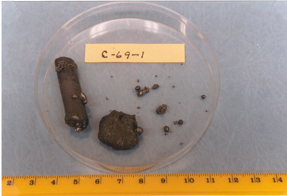
Figure 25. On many of the globules and the rods after cooling to room temperature were small nodules or rosettes of solidified melt that seemed to have been forced as a liquid from pores in the larger ferrosilicon bodies as they cooled.
