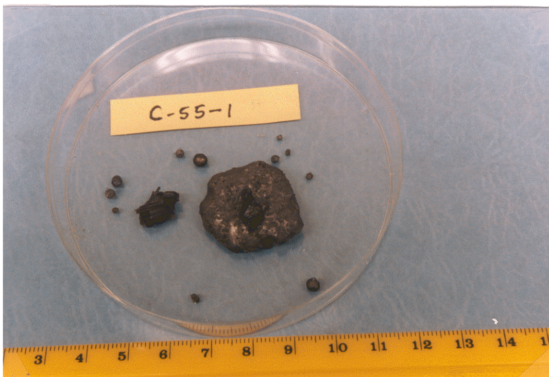
Figure 15. Typical debris recovered from an experiment performed with cold water; water temperature was 8 °C. Note the large number of smaller particles. The scale is divided into millimeters. (C-55-1)
