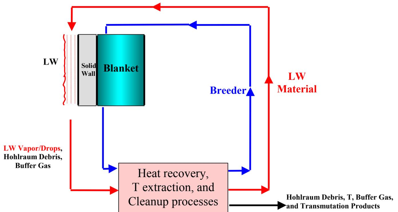
Figure 1. Liquid wall cycle for tangential injection scheme (no outside mixing of LW and breeding materials).
