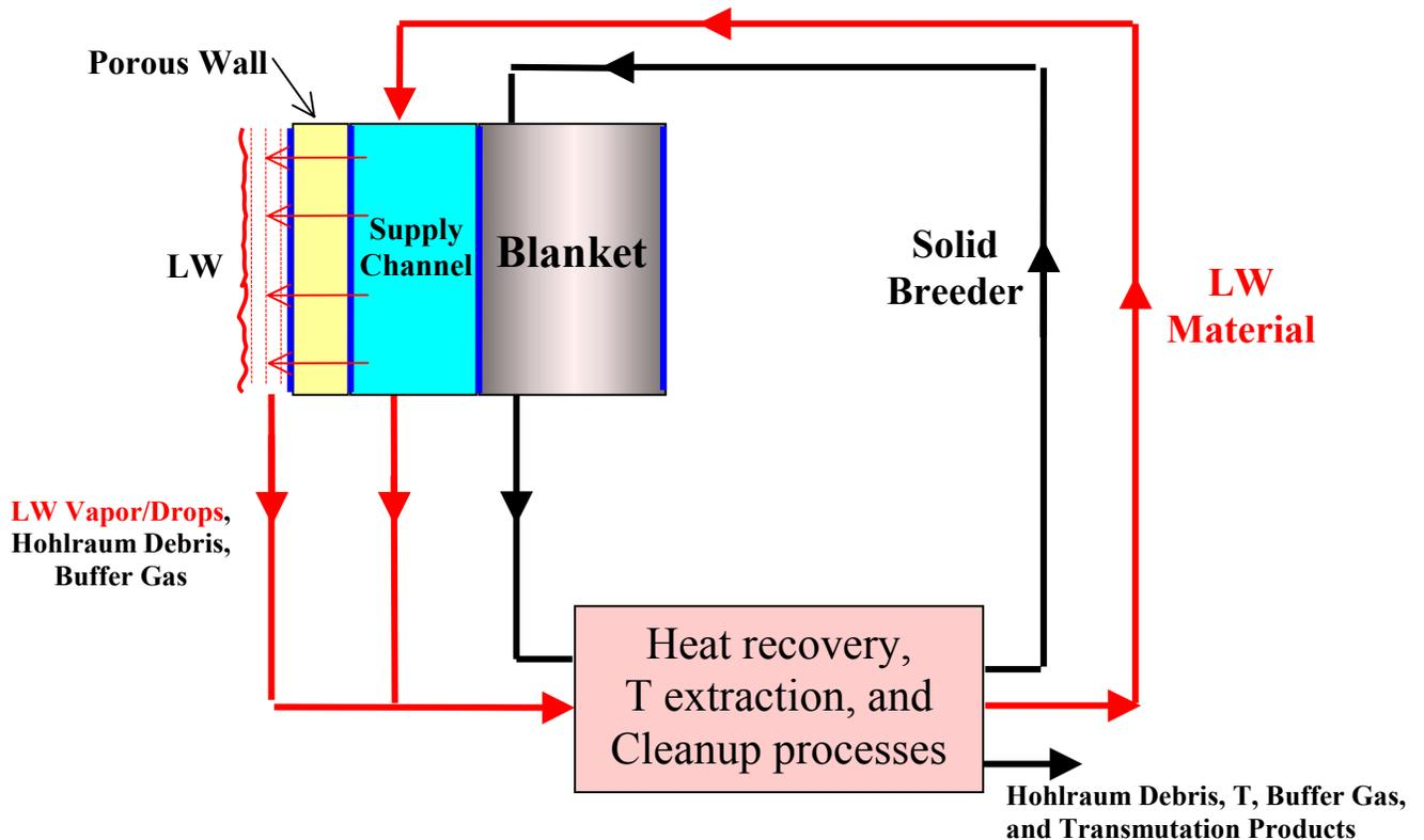
Figure 2. Flow diagram of liquid wall material seeping through porous wall from supply channel (no mixing of LW and breeding materials outside chamber).
