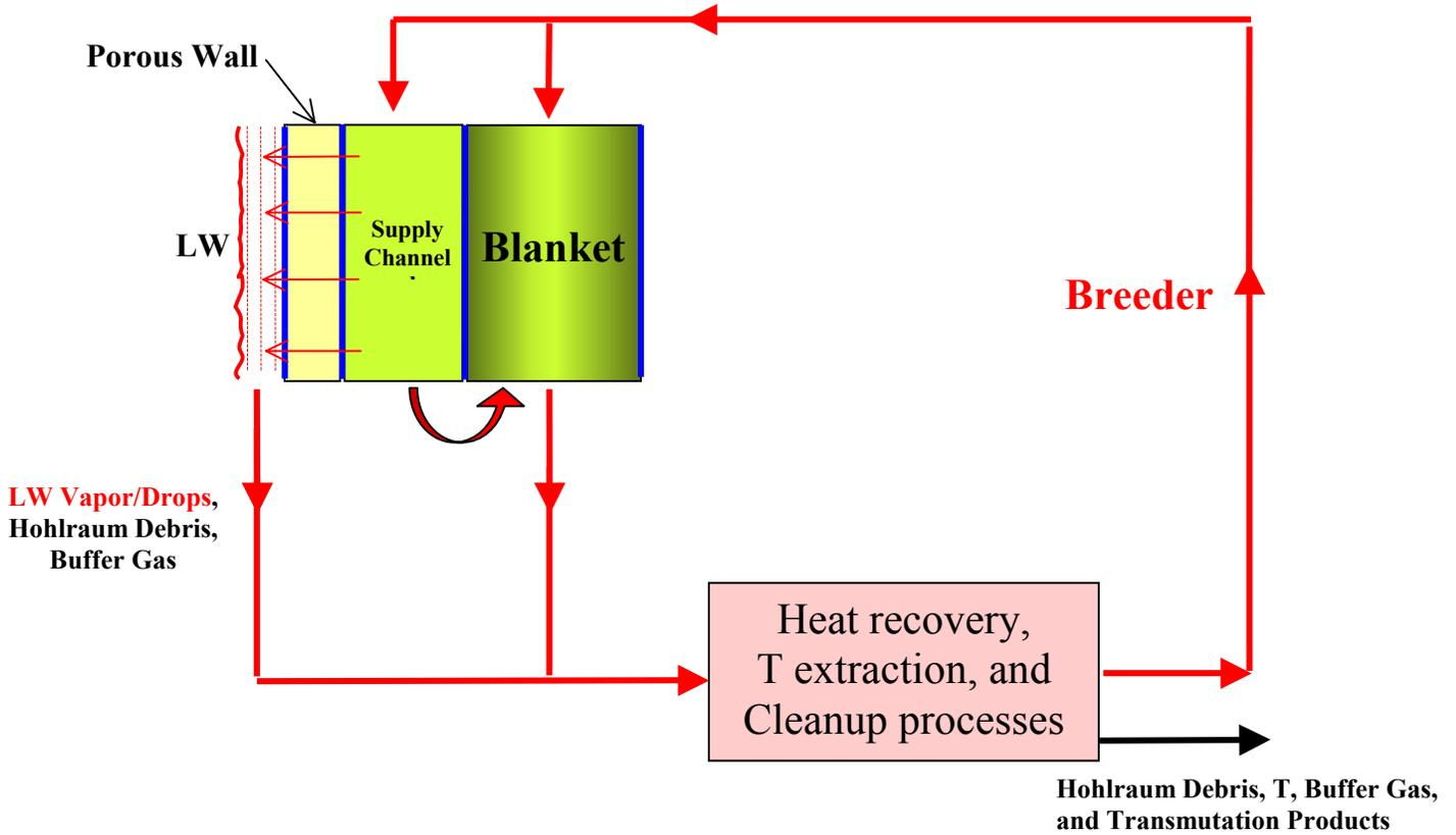
Figure 3. Porous wall injection scheme for liquid breeder blanket concept where LW and breeding materials mix inside and outside the chamber.
