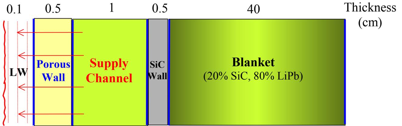
Figure 4. Representative radial build and typical dimensions of essential components for the porous wall injection scheme (not to scale).
