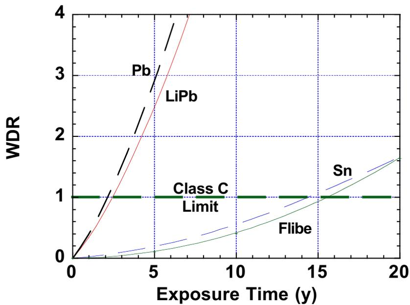
Figure 9. Increase of liquid film waste disposal rating with operation time assuming ~40 min in-chamber residence and no online removal of transmutation products.
