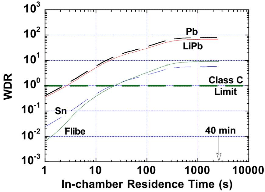
Figure 8. Variation of liquid film waste disposal rating with in-chamber residence time for 47 y of operation without removal of transmutation products.
