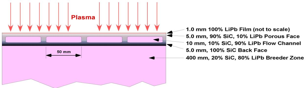
Figure 5. Schematic of thin liquid cooled wall with integral liquid breeding blanket (not to scale).
