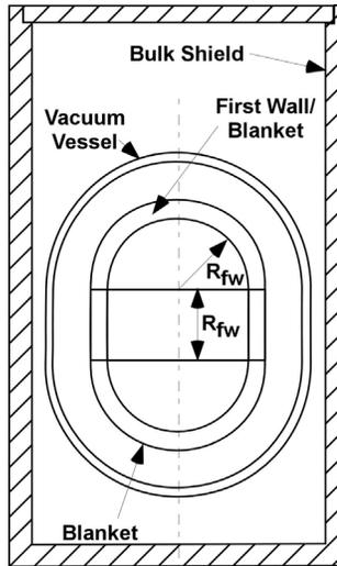
Figure 6. Representative power core geometry used for this analysis.
