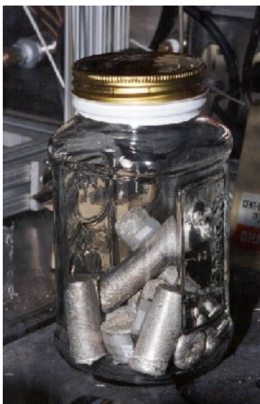
Figure 9: Alloy billets were stored in a sealed glass jar under an argon environment.
