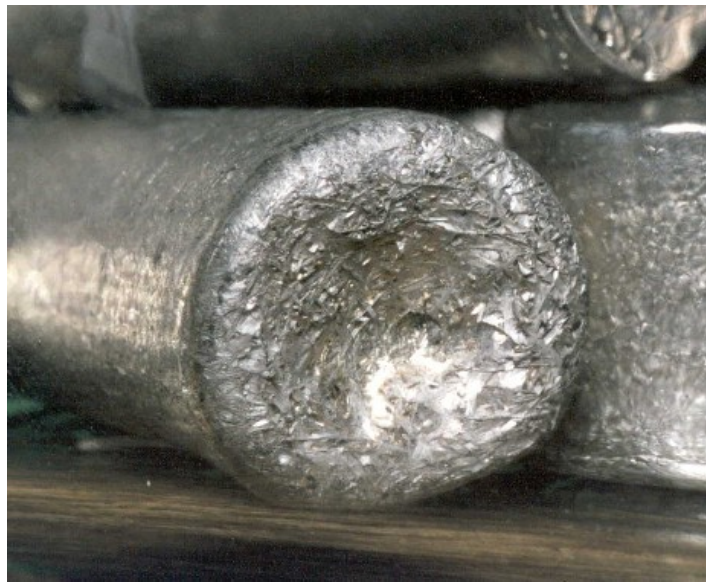
Figure 6: Crystal structure was formed at the billet alloy surface.
