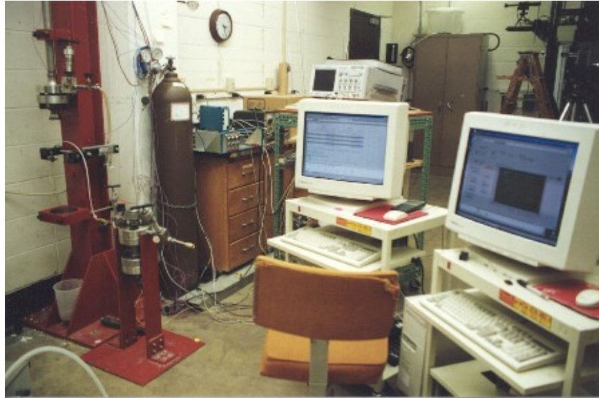
Figure 11: Data acquisition system recorded pressure and temperature data from the transducers.
