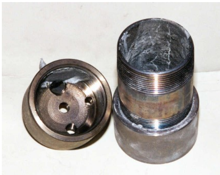
Figure 7: Reactor and reactor cap after casting the alloy.
