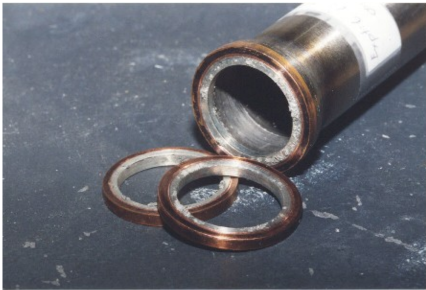
Figure 18: Some of the alloy debris can not be removed from the copper gasket.
