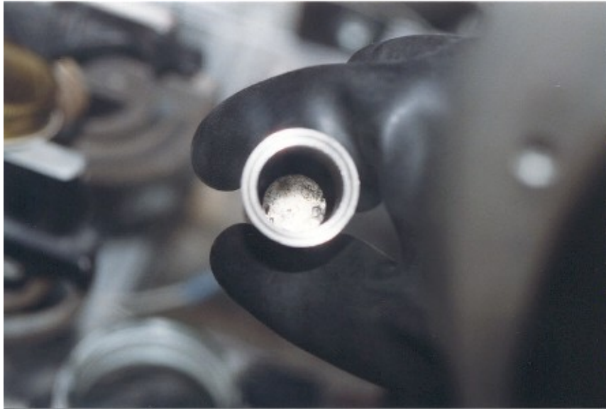
Figure 13: The test material is put into the crucible in the glovebox then seal the crucible with a rubber cap.
