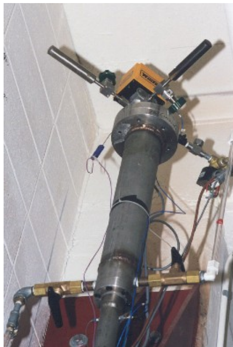
Figure 15: Two gas sample bottles are installed on the top of the expansion chamber.
