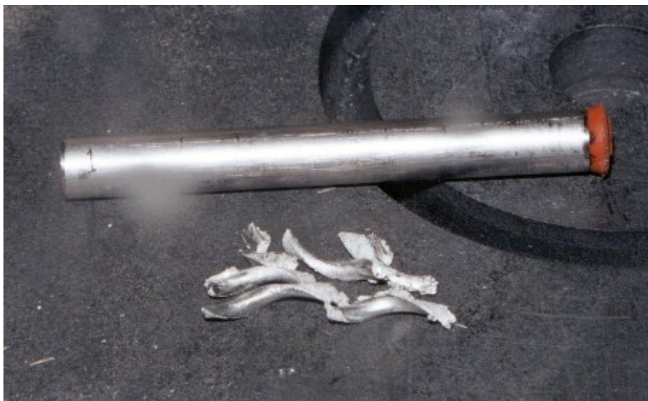
Figure 8: Core sample of the alloy to be sent to the laboratory.
