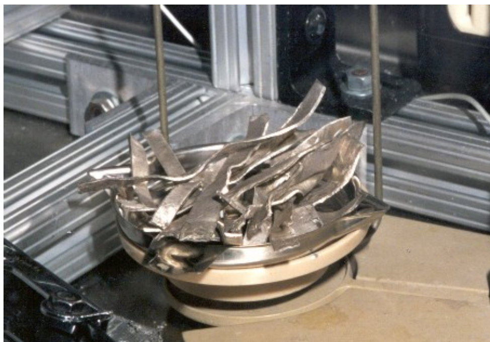
Figure 3: Li strip on the scale ready to put into the reactor.
