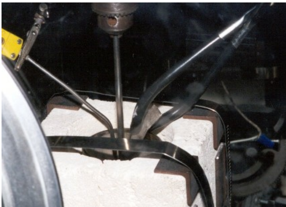
Figure 4: A lithium strip was added into the reactor after the tin was melted.
