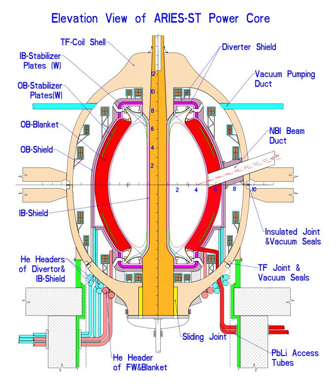
Figure 1. Vertical cross-section of ARIES-ST.
