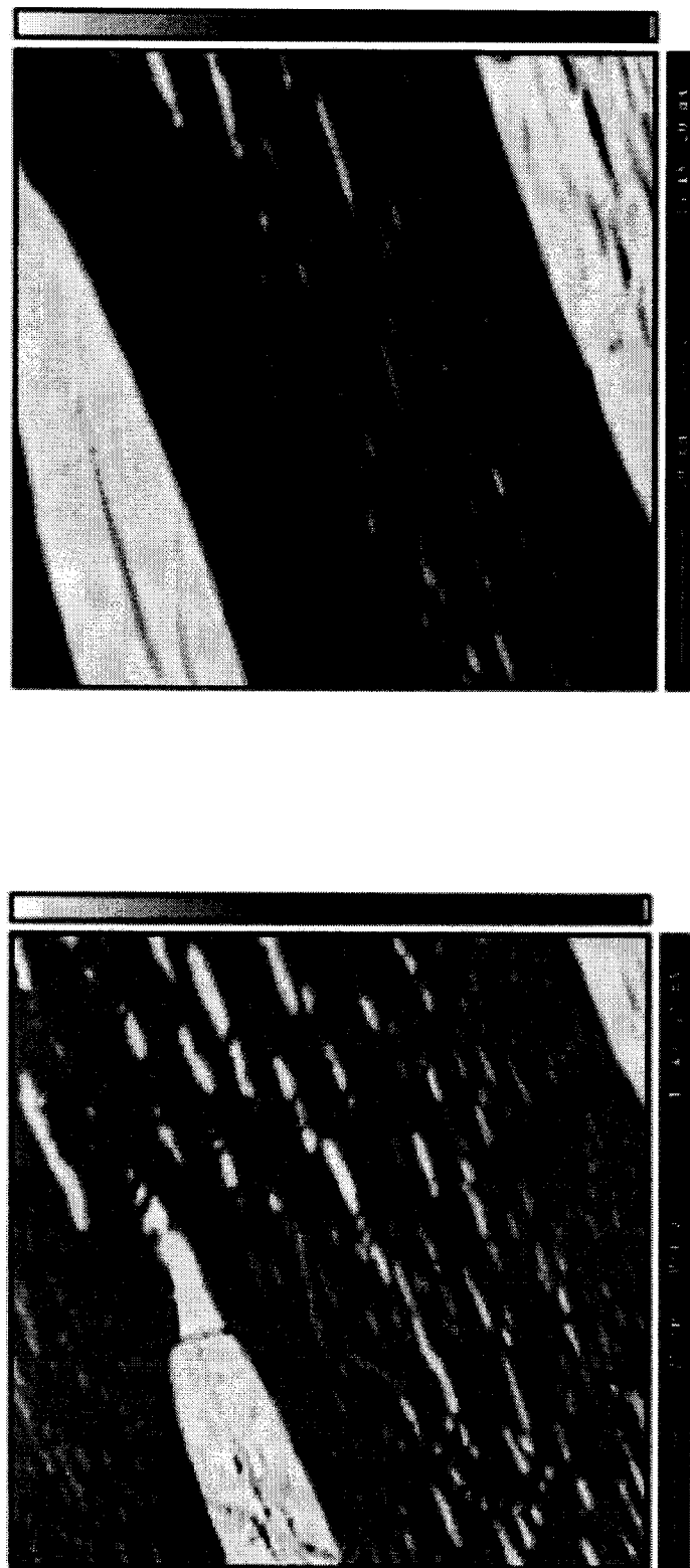
Figure 6-10. Backscattered electron micrographs of the ilmenite from St. Urbain, Quebec used in this thesis. Note the difference in scale between the two images. The dark gray bulk is ilmenite and the light gray is hematite.
