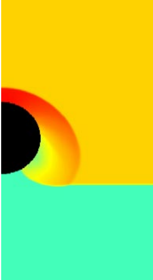
Figure 13. Density of shock in Wisconsin Shock Tube as it flows around a 3.175 cm radius cylinder. Calculated by RAGE for M=1.85 shock in atmospheric air.
