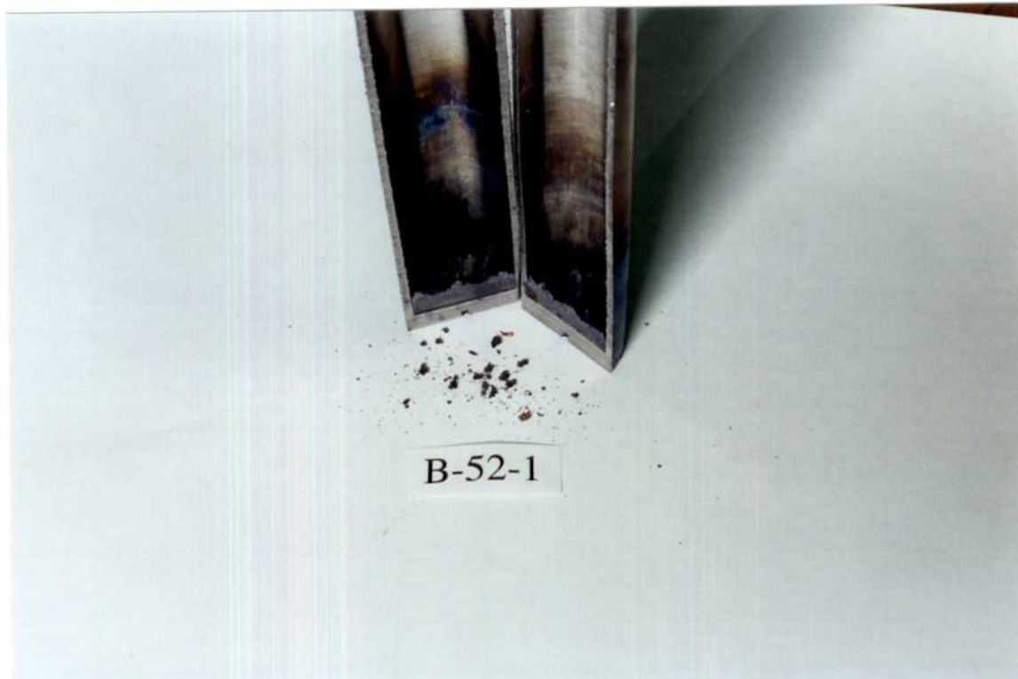
Figure 25. Photographs of the crucible with adhered Pb-Li debris from experiment B-52-1 after longitudinal sectioning: (a) (above) essentially perpendicular view (B-52-1-1); (b) (below) view from about 45^\circ to show the upper surface of the adhered debris (B-52-1-4). Notice in (b) the small amount of debris freed by the sectioning.
