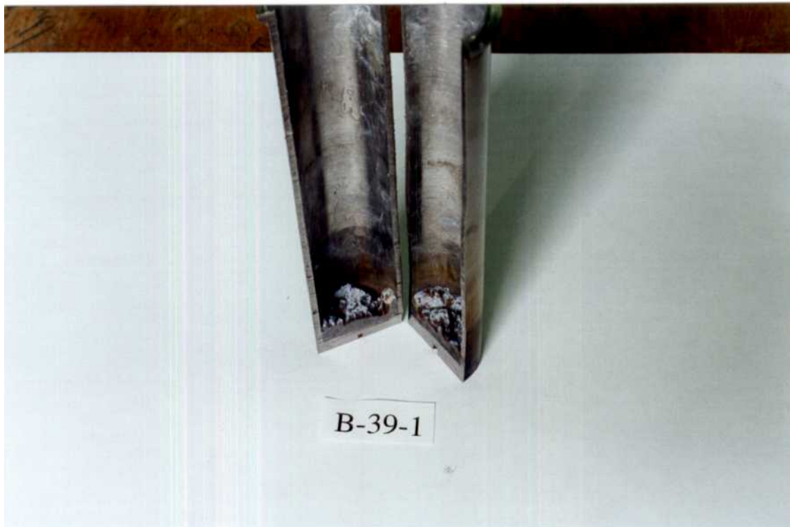
Figure 22. Photographs of the crucible with adhered Pb-Li debris from experiment B-39-1 after longitudinal sectioning: (a) (above) essentially perpendicular view (B-39-1); (b) (below) view from about 45^\circ to show the upper surface of the adhered debris. (B-45-1-4). Notice in (b) that essentially no debris was freed by the sectioning.
