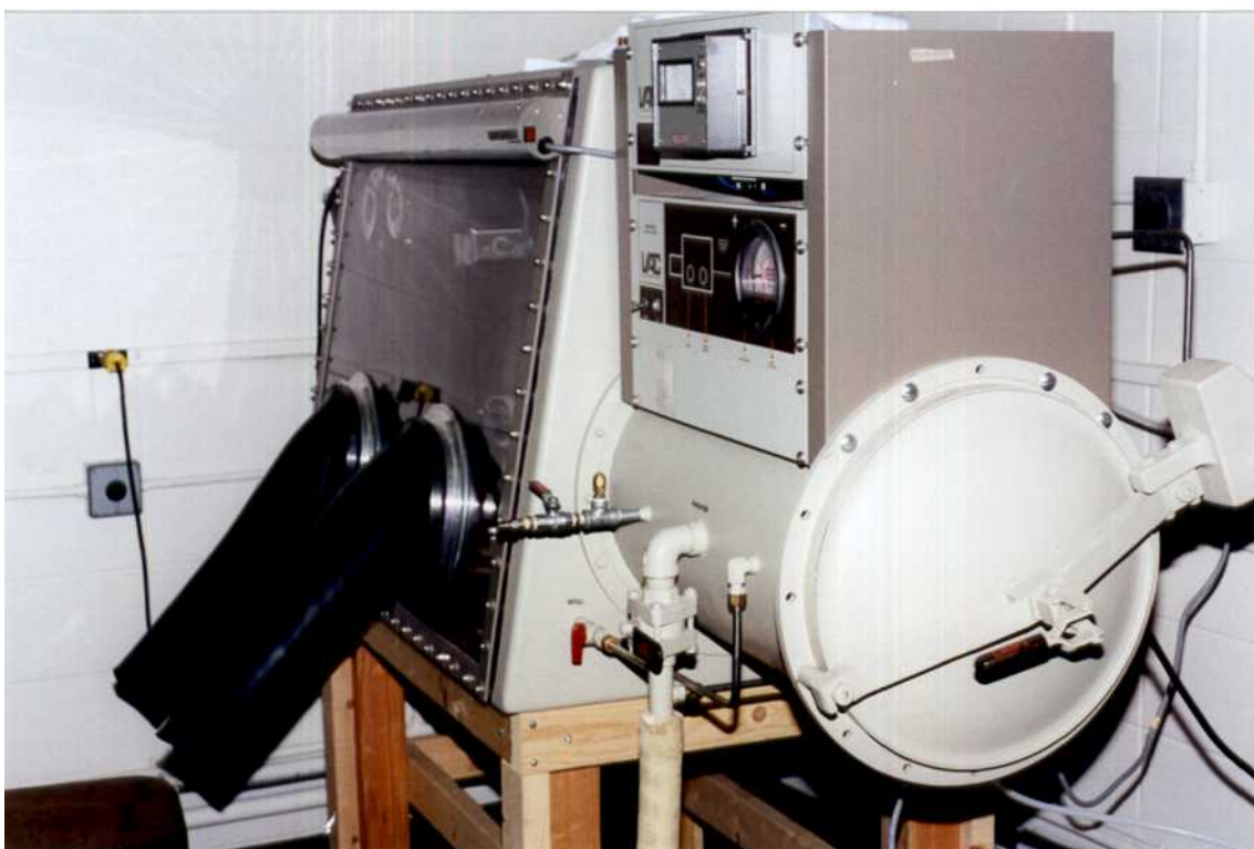
Figure 7. Glove box in which 83a/oPb-17a/o Li alloy was cast, weighed and loaded into the crucibles. (B-56-18)
