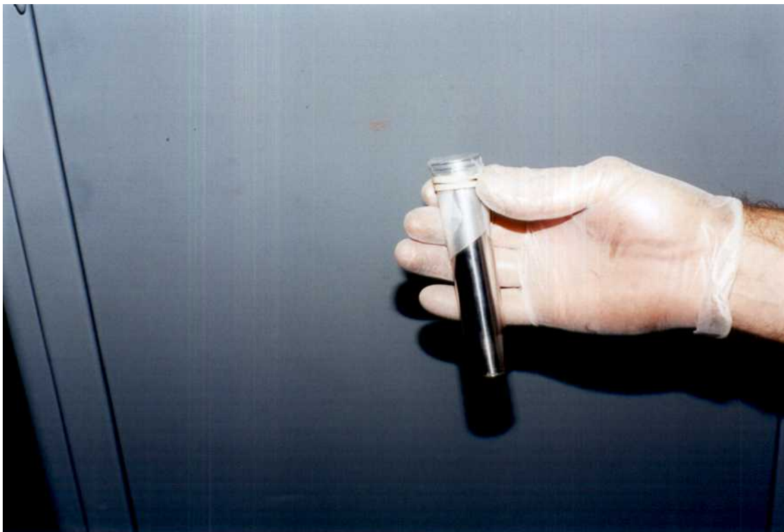
Figure 9. Crucible containing sample of the alloy and covered with paraffin foil after removal from the glove box. (B-39-1-1)
