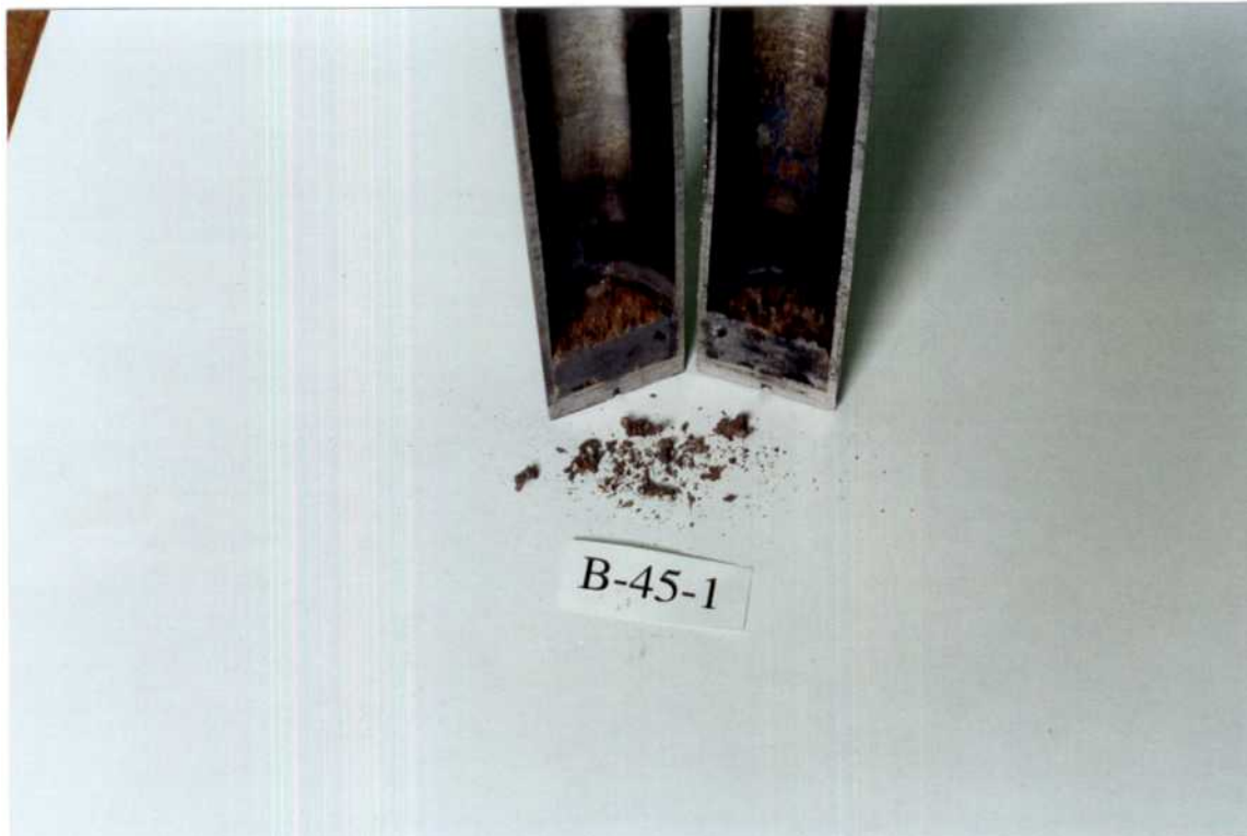
Figure 23. Photographs of the crucible with adhered Pb-Li debris from experiment B-45-1 after longitudinal sectioning: (a) (above) essentially perpendicular view (B-45-1-1);(below) view from about 45^\circ to show the upper surface of the adhered debris (B-45-1-4). Notice in (b) the small amount of red-brown debris freed by the sectioning.
