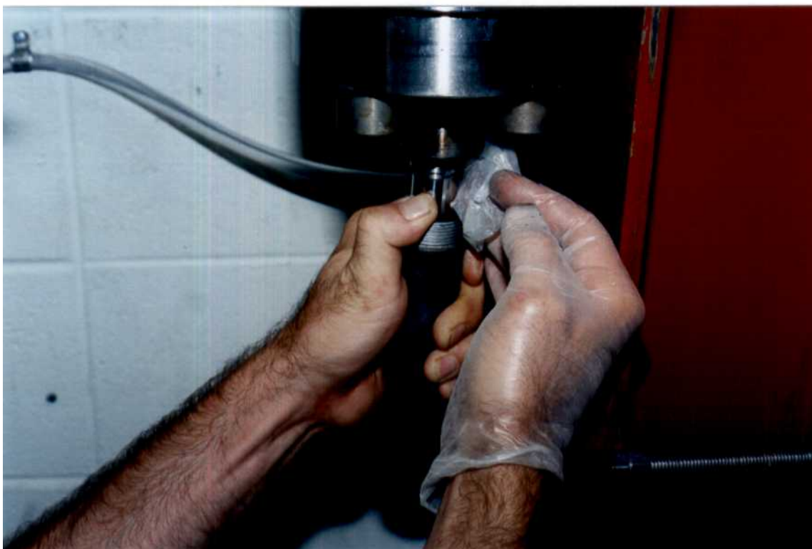
Figure 10. Top of crucible being stripped of paraffin foil just before the crucible is installed in the apparatus. Argon is flushing downward over the mouth of the crucible from the lower opening of the apparatus during the installation. (B-39-1-2)
