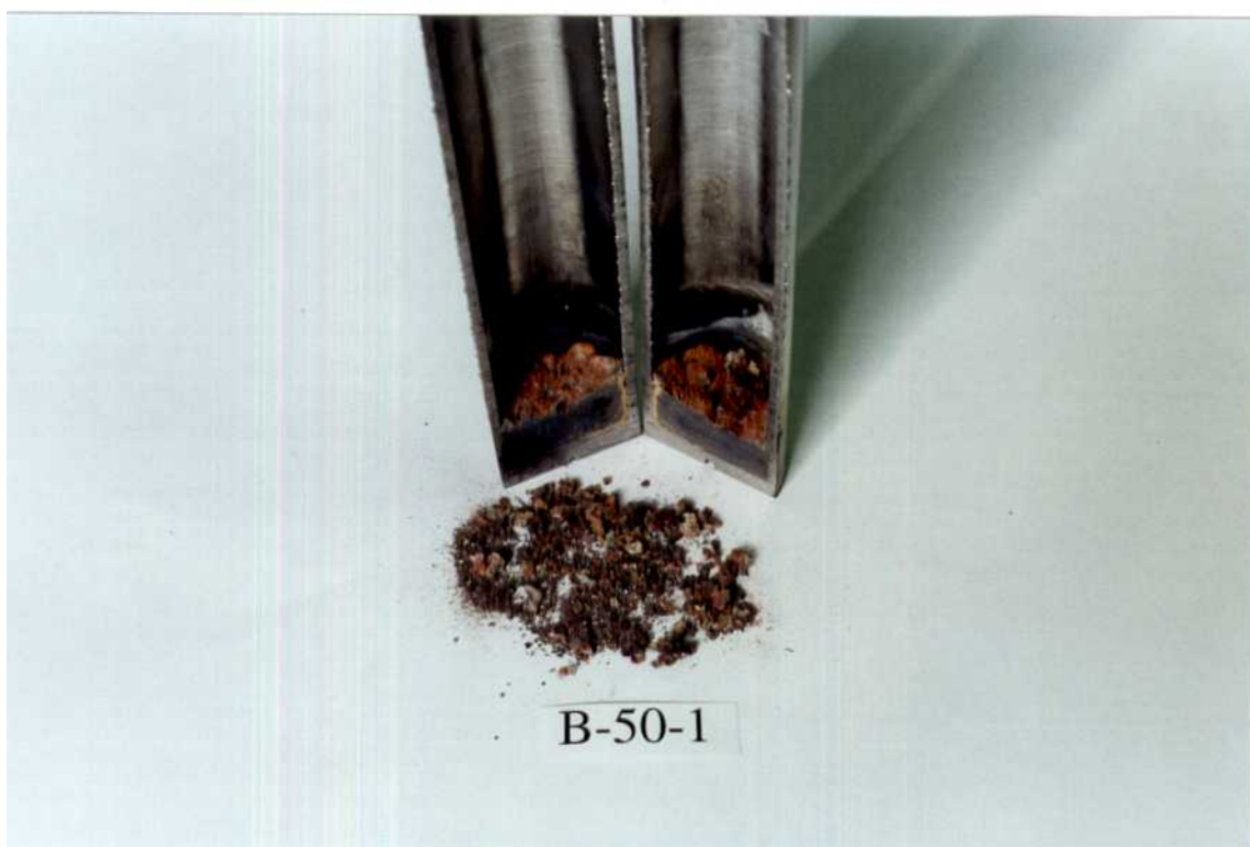
Figure 24. Photographs of the crucible with adhered Pb-Li debris from experiment B-50-1 after longitudinal sectioning: (a) (above) essentially perpendicular view (B-50-1-1); (b) (below) view from about 45° to show the upper surface of the adhered debris (B-50-1-5). Notice in (b) the large amount of red-brown debris freed by the sectioning.
