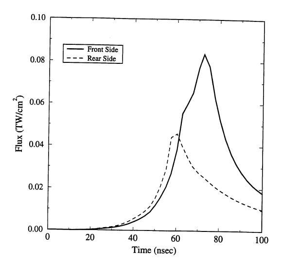
Figure 9. Time-dependence of radiation flux emitted from front (beam-irradiated) and rear sides of target for 6  $\mu$ m Al baseline simulation.
