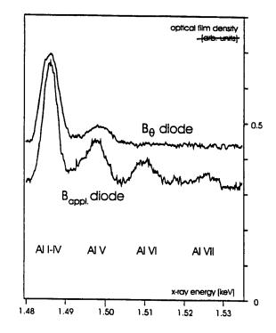
Figure 1. (Top) Comparison of  $K_{\alpha}$  emission spectra from 2  $\mu m$  and 6  $\mu m$  Al targets obtained in KALIF applied-B diode experiments. (Bottom) Comparison of  $K_{\alpha}$ emission spectra from KALIF  $B_{\theta}$  diode and applied-B diode shots (from Ref. [1]).
