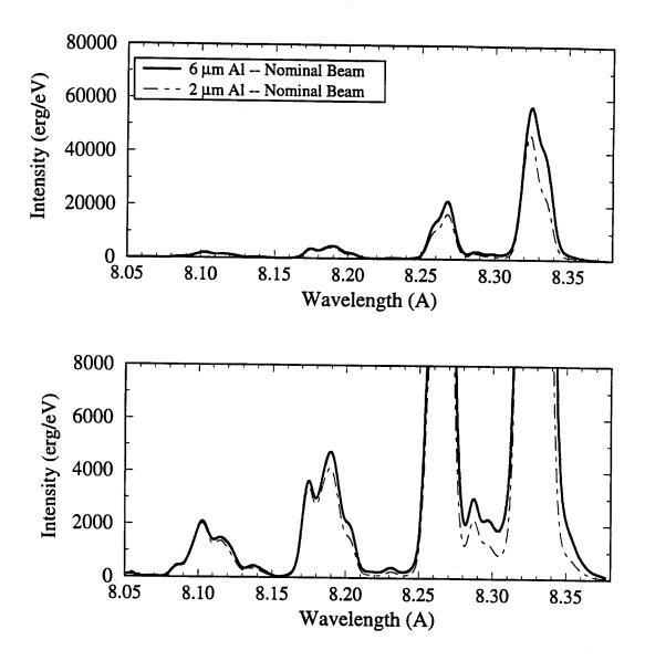
Figure 17. Comparison of space- and time-integrated  $K_{\alpha}$  spectra for 2  $\mu$ m and 6  $\mu$ m Al targets. Bottom plot shows same results on a different scale.
