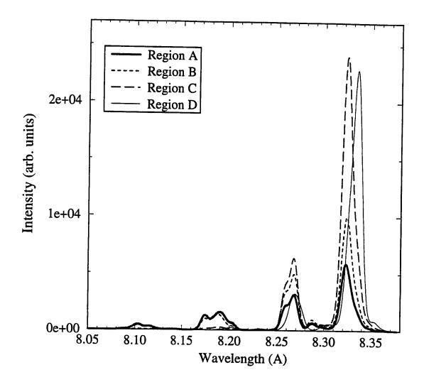
Figure 14. Area-weighted time-integrated spectra from Regions A through D for 6  $\mu$ m Al baseline simulation.
