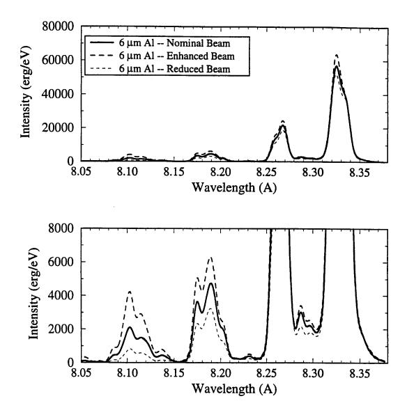
Figure 16. Comparison of space- and time-integrated  $K_{\alpha}$  spectra for 6  $\mu$ m Al targets using beam current density multipliers of 0.75, 1.0, and 1.25. Bottom plot shows same results on a different scale.
