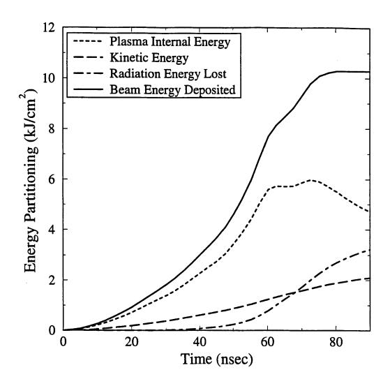
Figure 10. Energy partitioning in 6  $\mu$ m Al baseline simulation (Region A).
