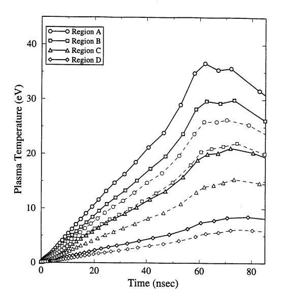
Figure 12. Evolution of mean temperatures in simulations using enhanced (multiplier = 1.25) and reduced (multiplier = 0.75) proton beam current densities.
