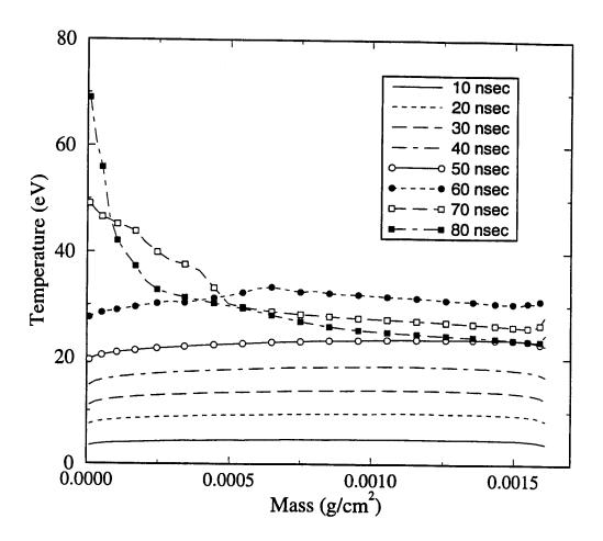
Figure 5. Temperature distribution in 6  $\mu$ m Al target at several rad-hydro simulation times (for Region A, nominal beam case).
