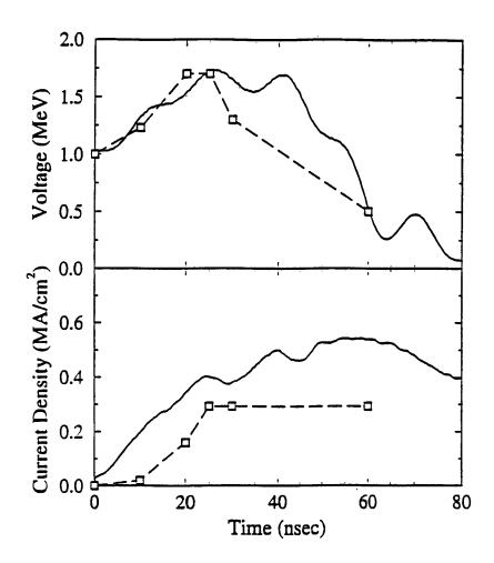
Figure 3. Time-dependent proton beam voltage and peak current density used in radiationhydrodynamics simulations. (solid curves).
