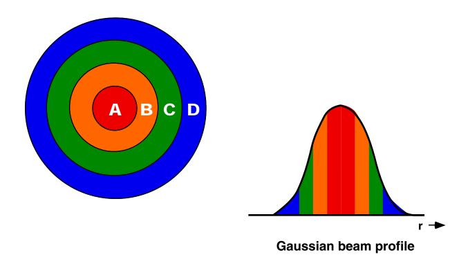
Figure 2. Schematic illustration of assumed Gaussian current density distribution on the target plane.
