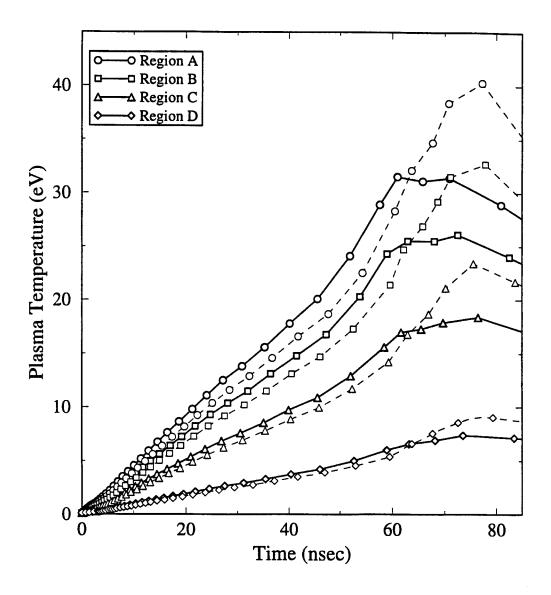
Figure 11. Comparison of mean temperatures in 2  $\mu$ m Al (dotted curves) and 6  $\mu$ m Al (solid curves) simulations.
