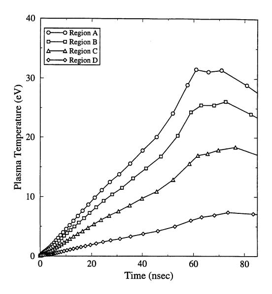
Figure 4. Time dependence of mean temperature in the Al target. Regions A through D represent different areas of the target plane (see Figure 2).
