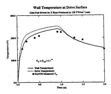
Fig. 1. Wall and drive temperatures in Nova Hohlraums. Drive and wall temperatures calculated by BUCKY for 150 TW/cm<sup>2</sup> laser. Wall temperatures are measured with DANTE.
