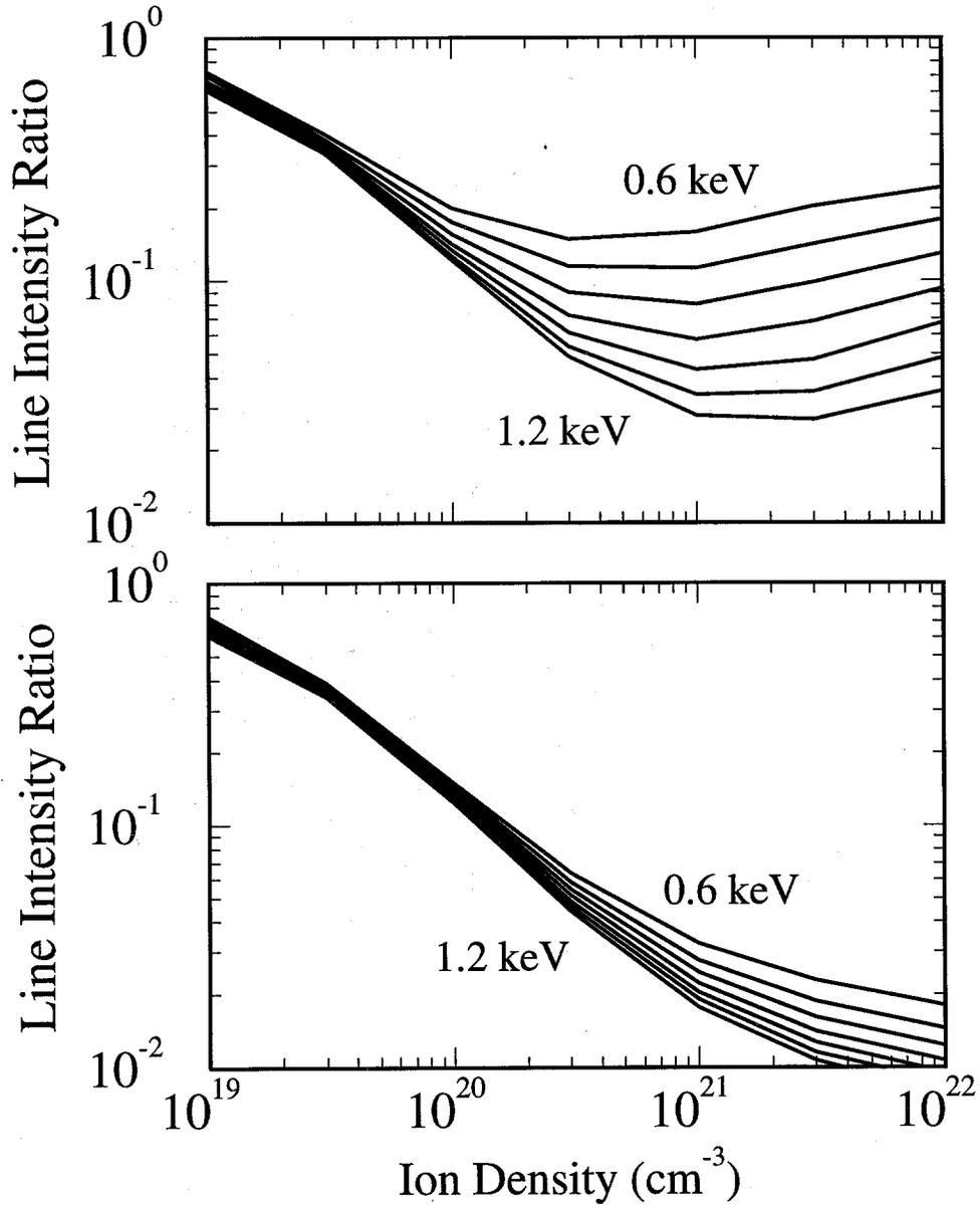
Figure 3. Intensity ratios for He IC plus Li-like satellites ( $mn + st$ ) to the  $\text{He}_\alpha$  line for  $\text{SiO}_2$  plasmas. (Top) For a finite cylindrical mass of  $6 \mu\text{g}/\text{cm}$ . (Bottom) Optically thin case. Curves correspond to temperatures ranging from 0.6 to 1.2 keV in increments of 0.1 keV.
