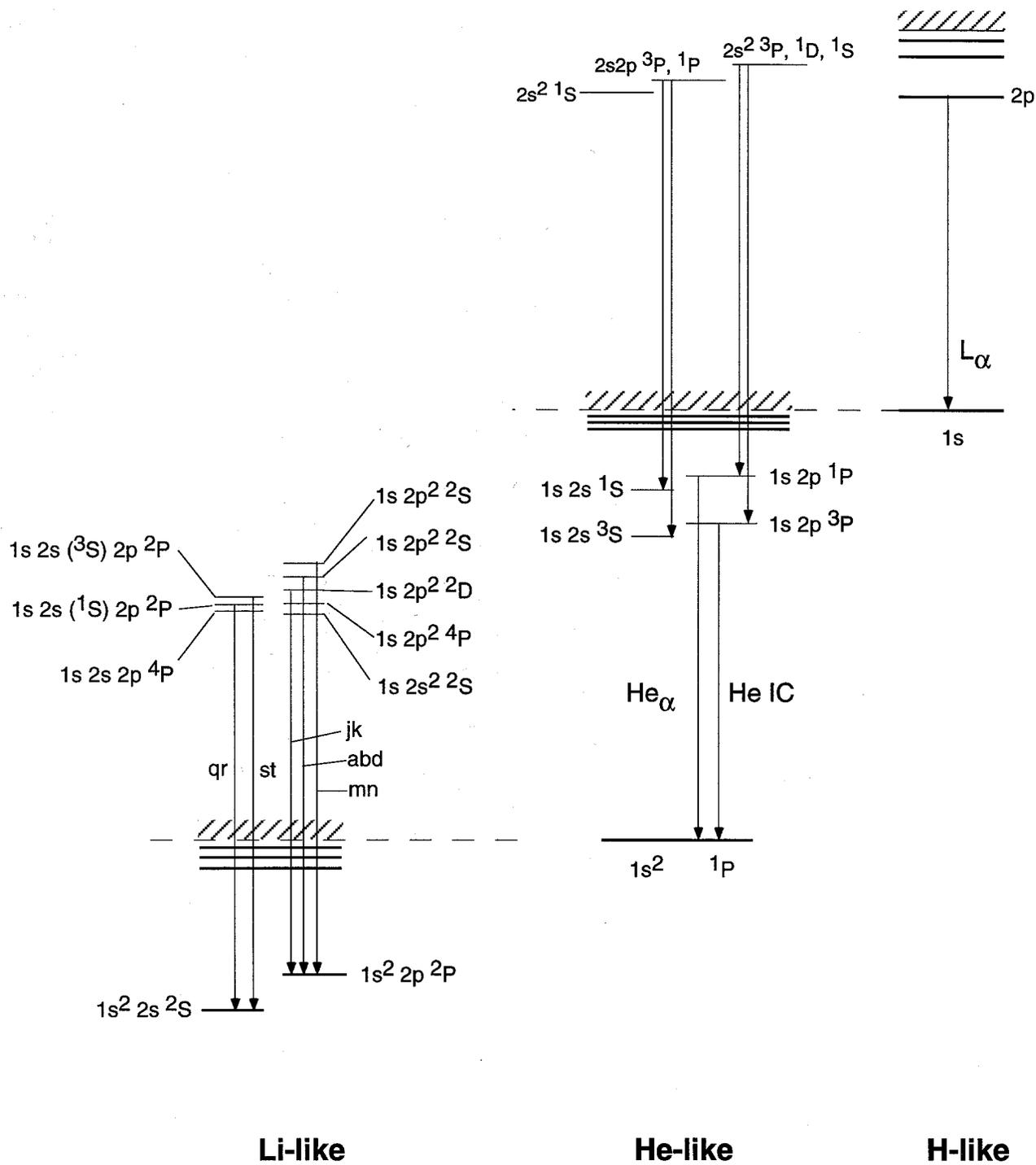
Figure 2. Schematic energy level diagram showing  $He_\alpha$  and  $L_\alpha$  lines and their satellites.
