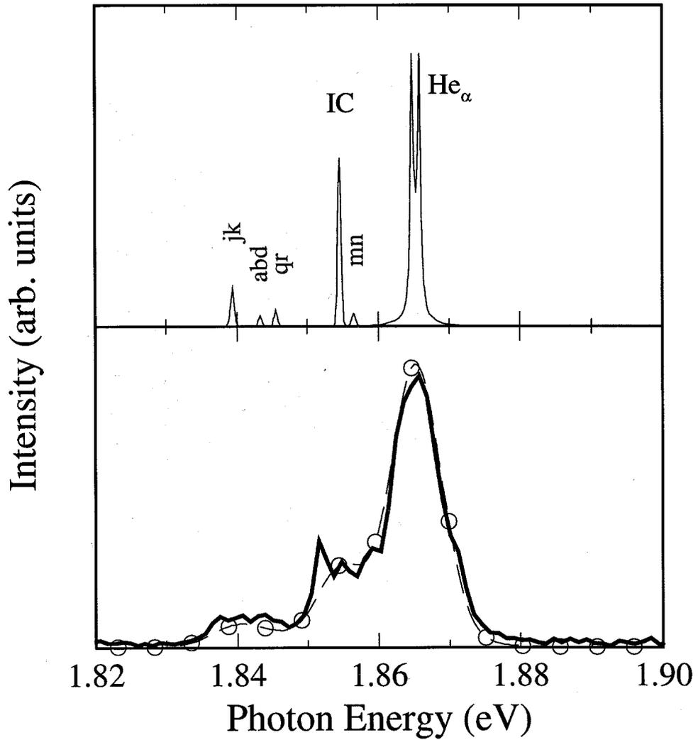
Figure 5. (Top) Calculated spectrum near Si He<sub>α</sub> line for an SiO<sub>2</sub> plasma at  $T = 400$  eV,  $n = 3 \times 10^{19}$  ions/cm<sup>3</sup>, and  $M = 6 \mu\text{g}/\text{cm}$ . (Bottom) Comparison of calculated spectrum including instrumental response of  $\lambda/\Delta\lambda = 250$  (dashed curve with circles) and experimental spectrum from Shot 2249 (solid curve).
