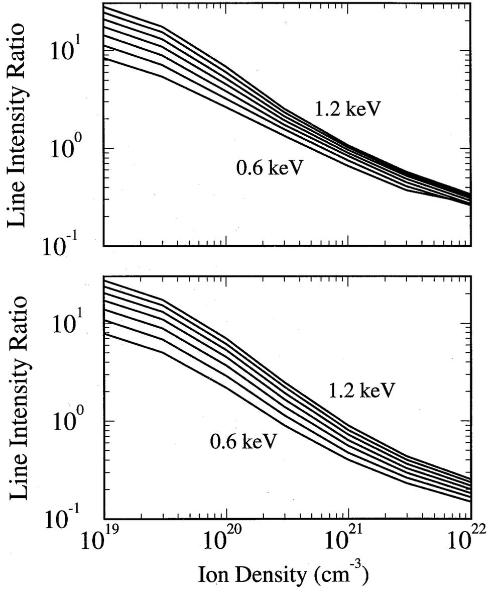
Figure 4. Intensity ratios for He IC plus Li-like satellites ( $mn + st$ ) to Li-like satellites ( $jk + qr + abd$ ) for  $\text{SiO}_2$  plasmas. (Top) For a finite cylindrical mass of  $6 \mu\text{g}/\text{cm}$ . (Bottom) Optically thin case. Curves correspond to temperatures ranging from 0.6 to 1.2 keV in increments of 0.1 keV.
