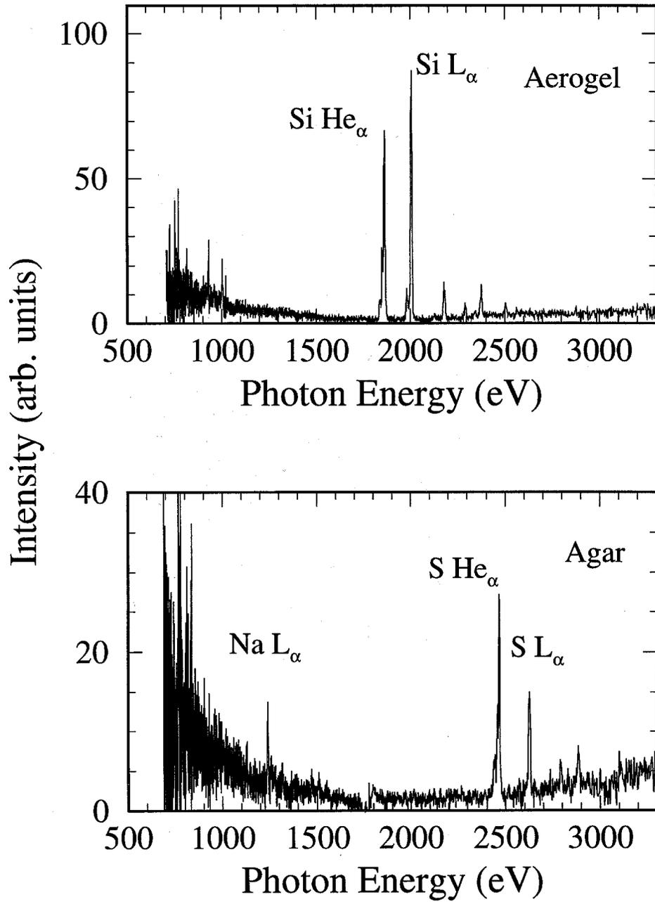
Figure 1. Time-integrated x-ray spectra for Shot 2249 (Si aerogel load) and Shot 2252 (agar load).
