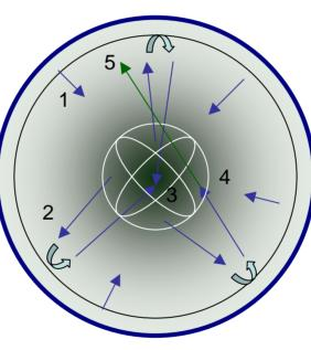
4. The ions can also undergo a charge exchange, creating a fast neutral.
