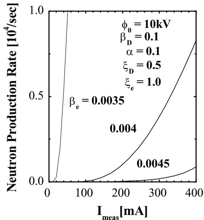
Neutron production rate for several  $\beta_e$  values as a function of the discharged current.
