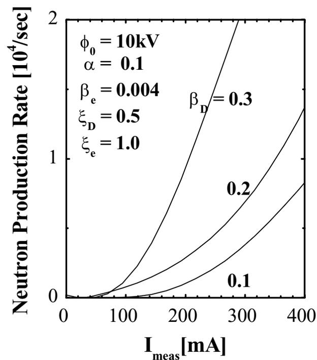
Neutron production rate for several  $\beta_D$  values as a function of the discharged current.
