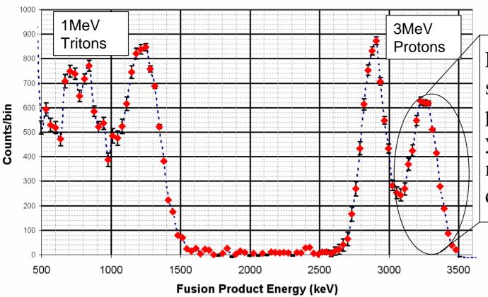
Examining either side of the double peaked spectra can yield center of mass energy of the deuterium reactants
