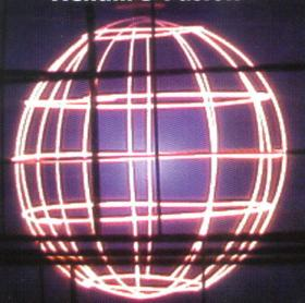
Approximately seven times hotter than the Sun's core, the fusion of Helium-3 and Hydrogen-2 within an electrostatic containment reactor at the Fusion Technology Institute, University of Wisconsin in Madison.
